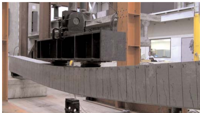
Figure 8. Crack patterns and curvature in Specimen F4 immediately prior to failure.
