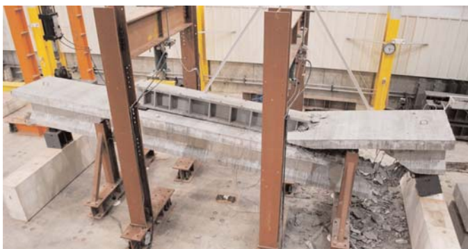
Figure 18. Failure mode of SP4 (A1035 side).
