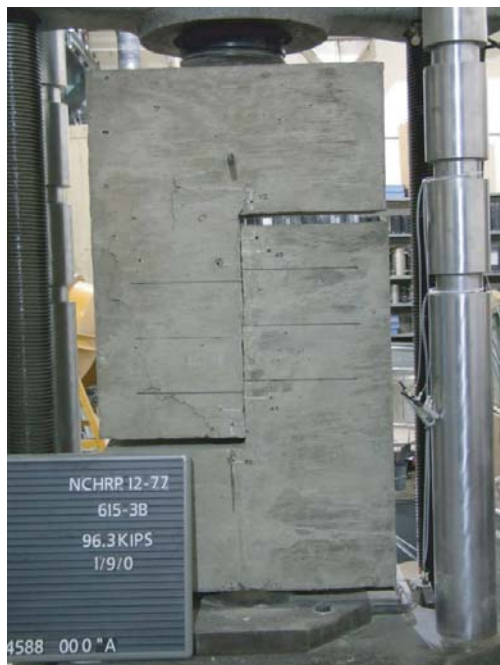
(a) P615-3B at a slip exceeding 1 in. ( \Delta can be seen as displaced horizontal lines representing interface reinforcement locations)
