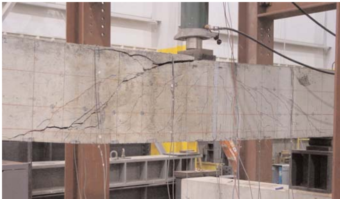
Figure 17. Failure mode of SR2 (A615 side).
