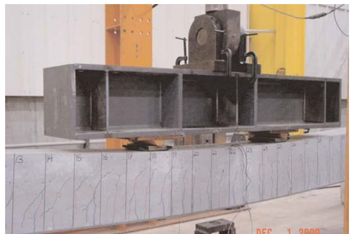
Figure 7. Cracking patterns in Specimen F4 prior to failure.
