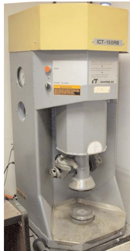
Figure 5. Gyratory compactor with shear stress measurement.
