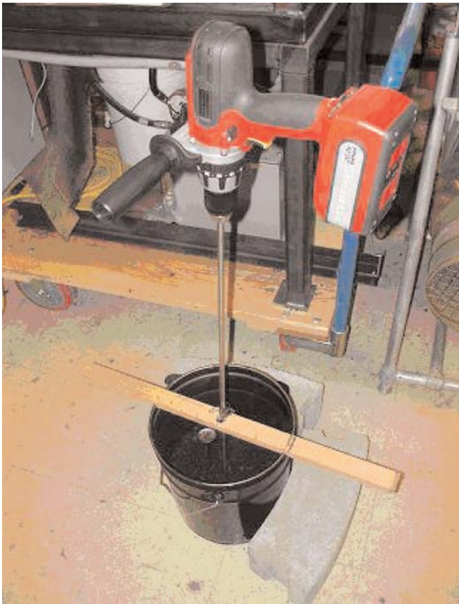
Figure 4. University of New Hampshire workability device.
