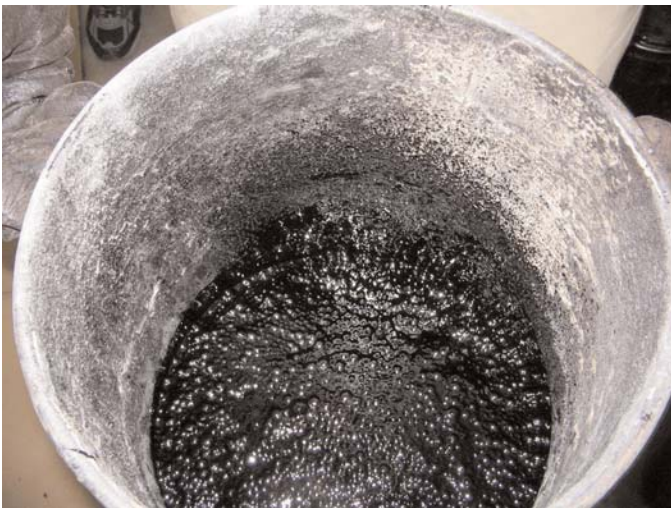
Figure 37. Foamed asphalt before mixing.
