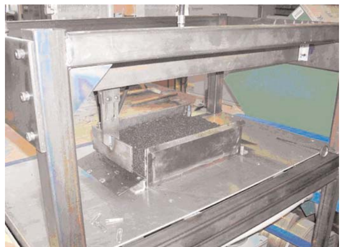
Figure 3. Nynäs workability device.
