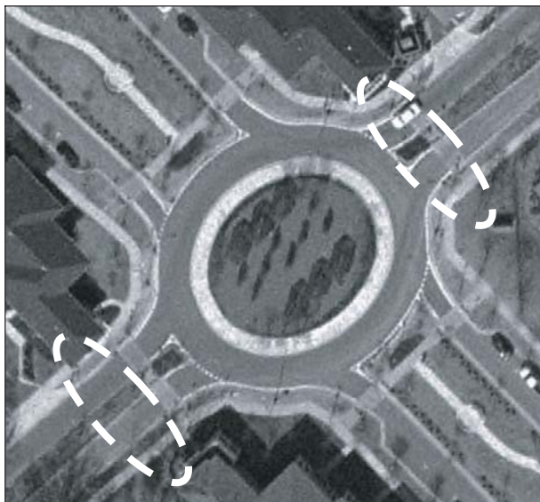
This figure shows two photographs of the studied single-lane roundabout at the intersection of Davidson Street and 9th Street in Charlotte, NC. The left image shows an aerial photograph with the studied crosswalks highlighted on the southwest and northeast approaches of Davidson Street. The right image shows a pedestrian-level photograph of the roundabout entry leg.
