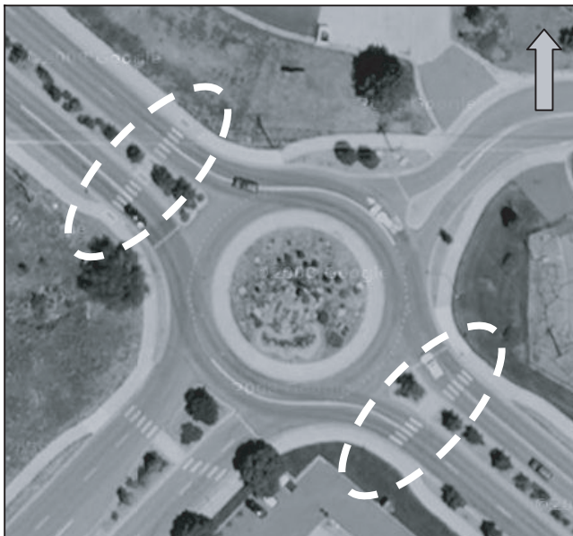
This figure shows an aerial photograph of the two-lane roundabout treatment site at the intersection of Golden Road and Johnson Road in Golden, CO. The studied crosswalks are highlighted and located in the southeast and northwest approaches of Golden Road.
