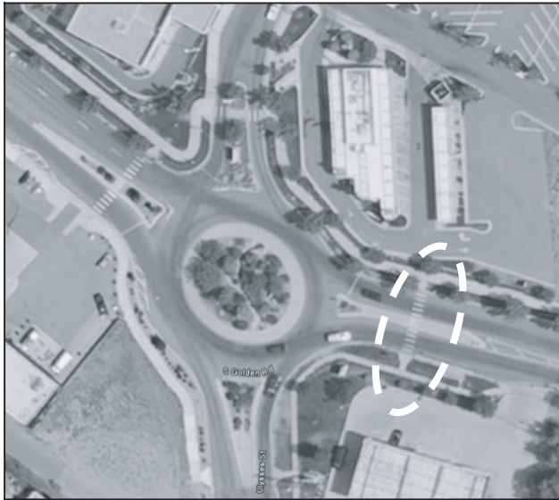
This figure shows two photographs of the studied single-lane roundabout at the intersection of Golden Road and Ulysses Street in Golden, CO. The left image shows an aerial photograph with the studied crosswalks highlighted on the east approaches of Golden Road. The right image shows a pedestrian-level photograph of the roundabout entry leg.
