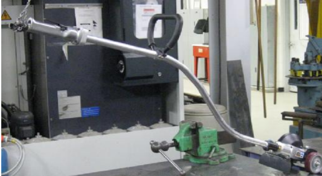
FIGURE 17: Finalized shaft design.
