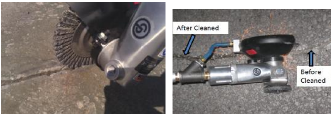
FIGURE 12: Twisted wire narrow faced brush test.
