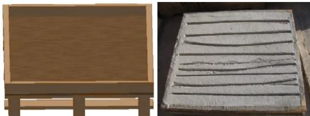
FIGURE 19: As modeled(left) and as tested standardized crack test bed(right).
