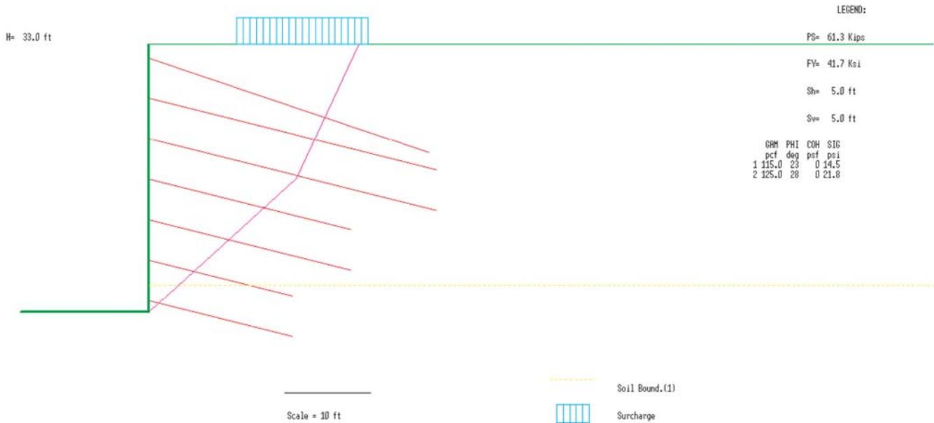
Figure D-6. Critical failure surface calculated using SNAILZ.
