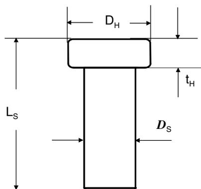
Figure 11.12.6.4-1 Geometry of a Headed-Stud
