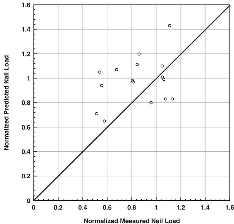
Figure 3-31. Measured and predicted maximum nail load.
