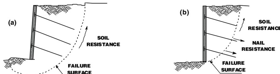
**Figure 11.12.3.3-1 Limit States in Soil Nail Walls—Overall Stability: (a) Slip Surface not Intersecting Nails; (b) Slip Surface Intersecting Nails**
