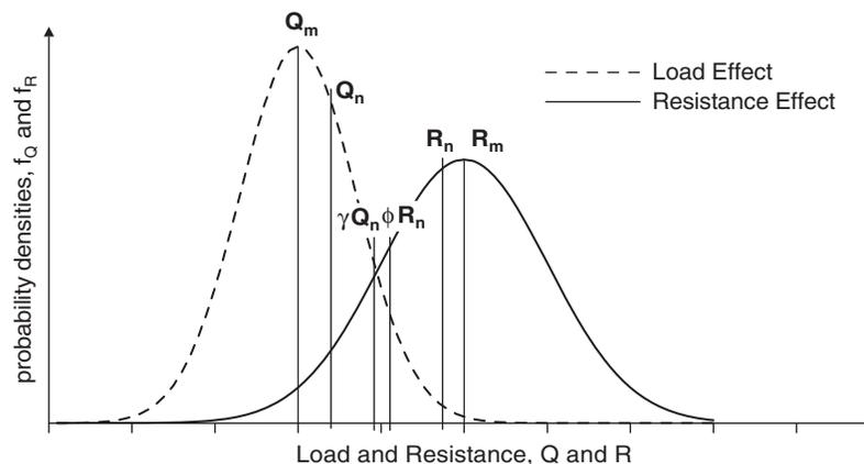
Figure 3-1. Probability density functions for load and resistance.
