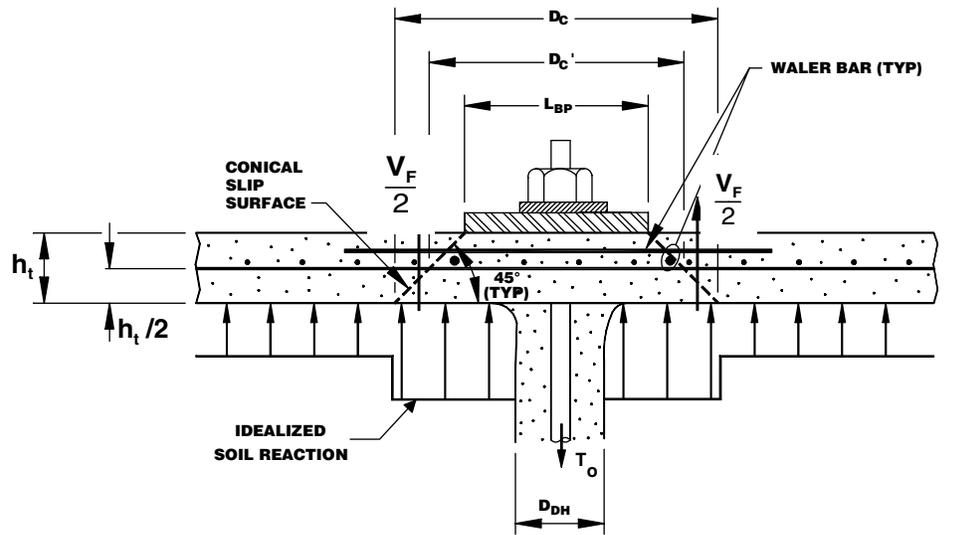
(a) BEARING-PLATE CONNECTION (vertical view)
