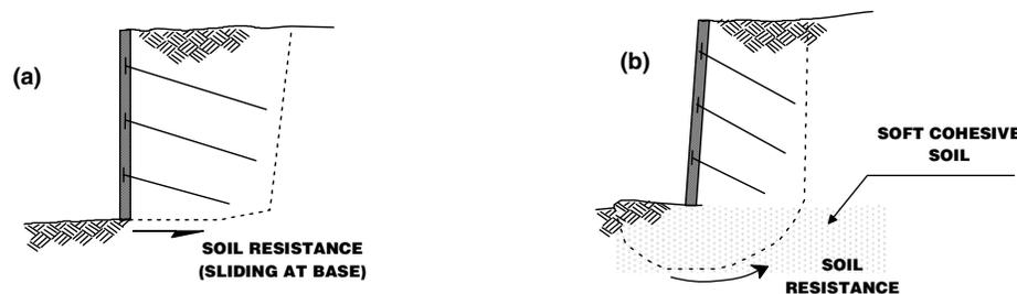
Figure 11.12.4-1 Soil Limit States: (a) Sliding Stability; (b) Basal Heave
