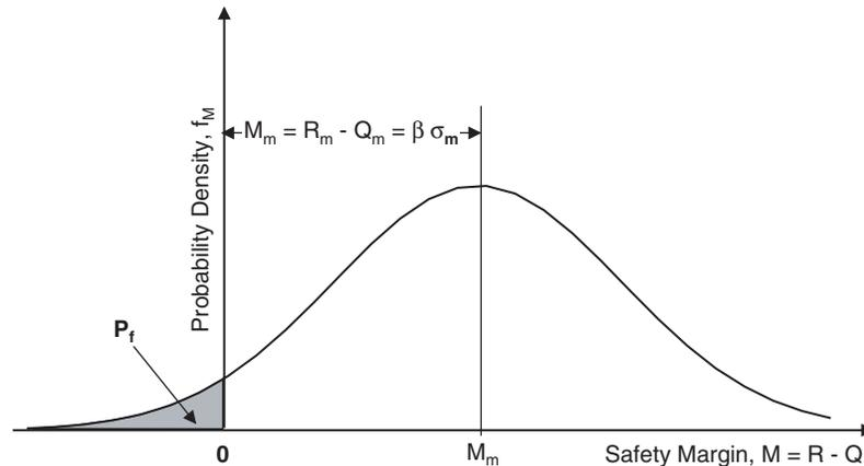
Figure 3-2. Probability density function of safety margin,  $M$ .
