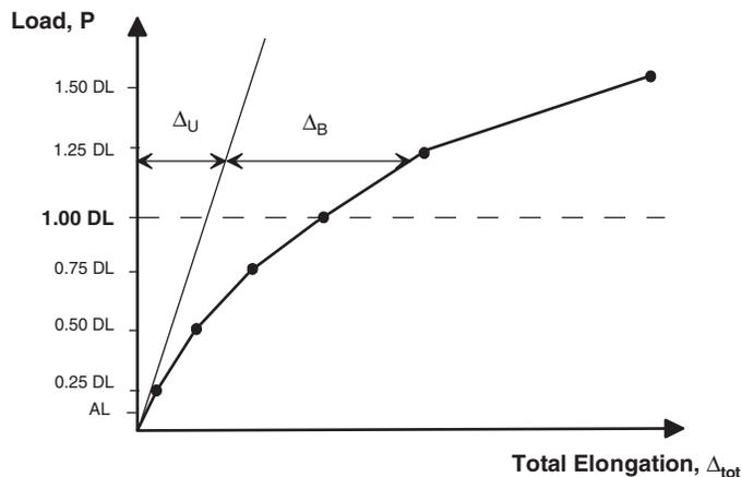
Figure 3-22. Reduction of soil nail load-test data.
