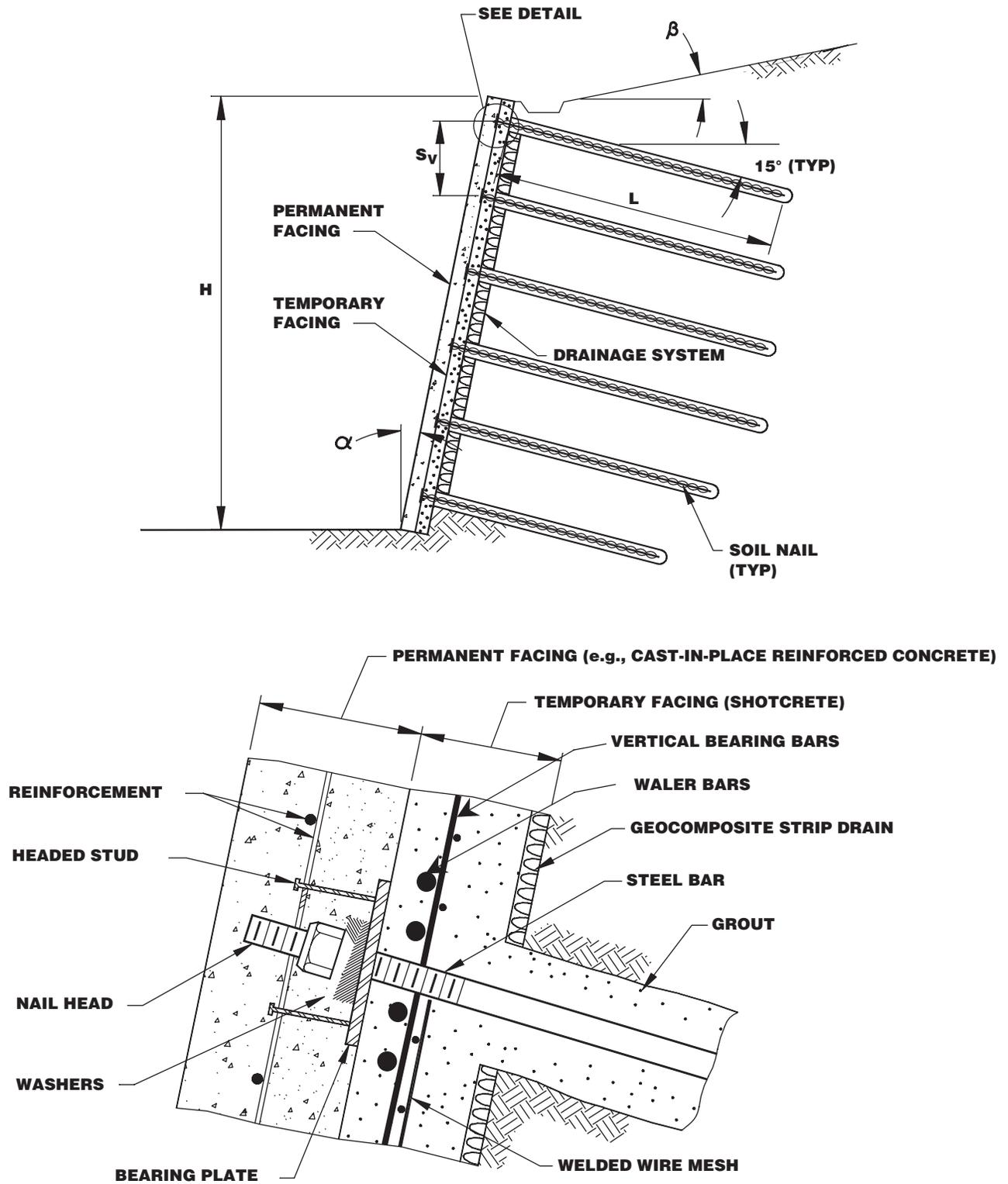
Figure 3-4. Typical cross section of a soil nail wall in common U.S. practice.
