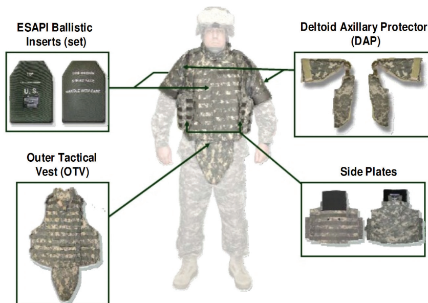
FIGURE 2-5 Interceptor body armor. Shown are the various components that make up the Interceptor body armor system (see DoD Inspector General's Report No. D-2009-047, January 29, 2009). The outer tactical vest, the deltoid axillary protectors, and the carrier for the ESAPI inserts (not shown) are made of Cordura, Kevlar, and/or Twaron fabric. The ESAPI ballistic inserts are composite ceramic plates with ballistic fiber backing (see the Interceptor body armor [IBA] brochure of the Program Executive Office, Soldier, October 2010). SOURCE: DoD Inspector General. 2009. DoD Testing Requirements for Body Armor. Report No. D-2009-047, January 29. Available online at http://www.dtic.mil/cgi-bin/GetTRDoc?AD=ADA499208&Location=U2&doc=GetTRDoc.pdf . Last accessed April 29, 2011.
