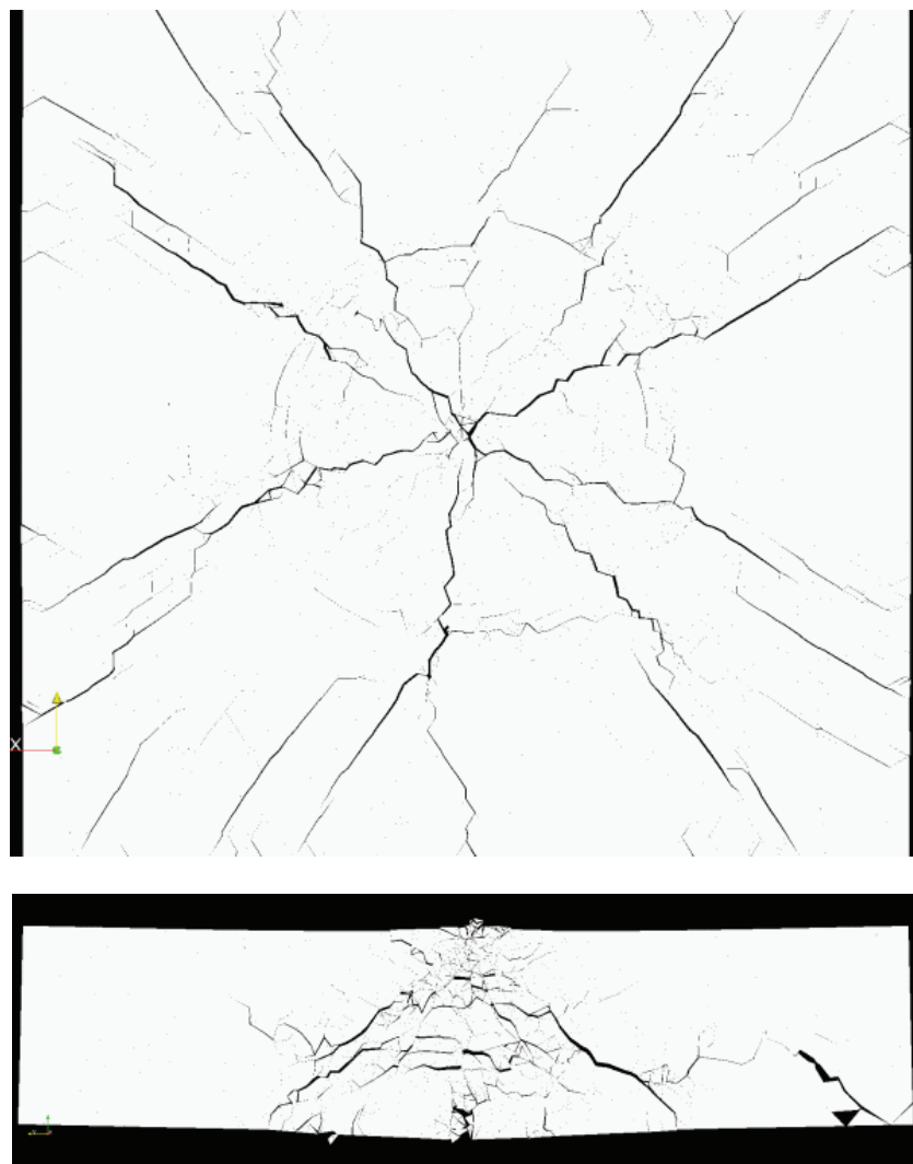
FIGURE 4-18 Prediction of conical, radial, and lateral crack patterns in ceramic plate impact by the recent cohesive zone/discontinuous Galerkin method.
