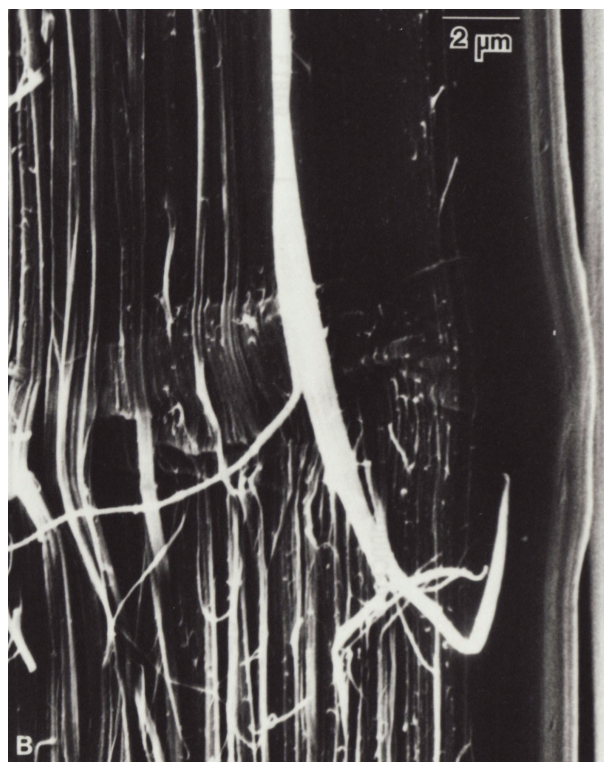
FIGURE 3-8 SEM micrograph revealing fibrillar microstructure in an as-spun PBZT fiber. SOURCE: Allen, S.R. 1983. Mechanical and morphological correlations in poly-(p-phenylene benzobis-thiazole) fibers. Ph.D. Dissertation. Amherst, Mass.: University of Massachusetts.
