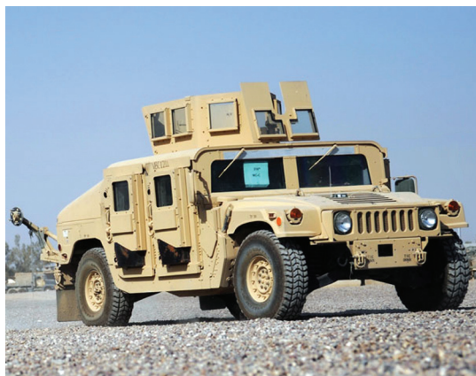
FIGURE 1-2 Up-armored high-mobility multipurpose wheeled vehicle (HMMWV, or Humvee). SOURCE: Available at http://www.militaryfactory.com/armor/imgs/hmmwv-m1114uah.jpg . Courtesy of U.S. DoD.
