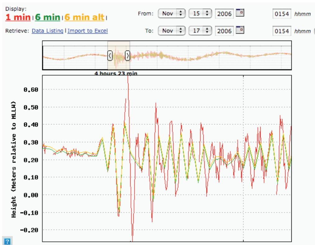
**FIGURE 4.2** Sea level data from Midway Island for a short time period encompassing the arrival of the November 15, 2006, Kuril Island tsunami. One-minute samples are shown in red; two different gauges providing 6-minute samples are shown in green and orange. Note that the 6-minute samples completely miss the highest amplitude component (the third crest and trough) of the tsunami. SOURCE: <http://co-ops.nos.noaa.gov/tsunami/>; NOAA.
