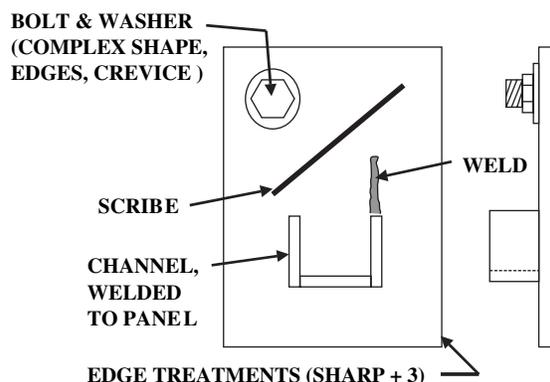
**Figure 1** Test panel used for corrosion testing.
