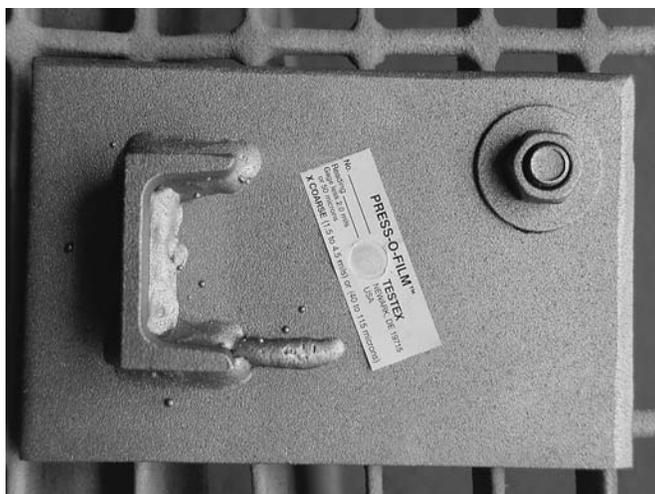
**Figure 2** Testex™ tape to evaluate surface profile.
