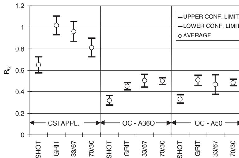
**Figure 9** Values of  $R_Q$  versus abrasive mix and applicator.
