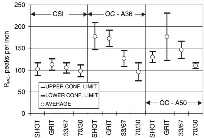
**Figure 8**  $R_{PC}$  versus abrasive mix and applicator.
