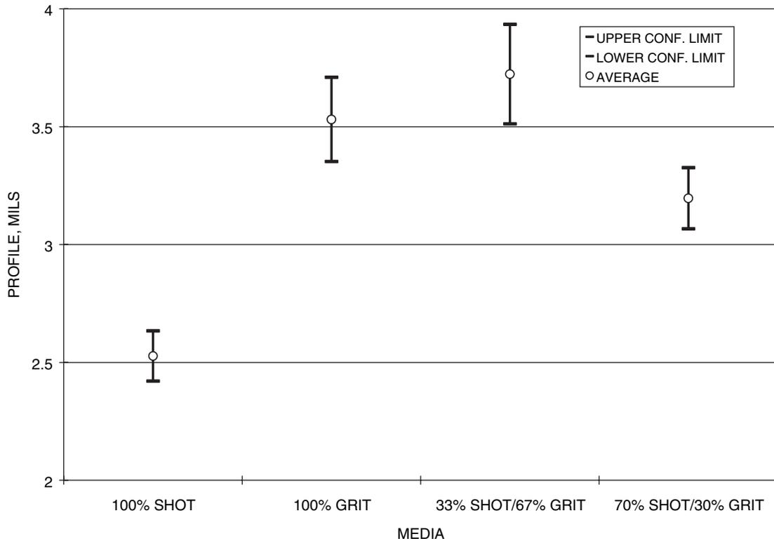
**Figure 5** Testex™ replica tape profile ranges (CSI-prepared test panels).
