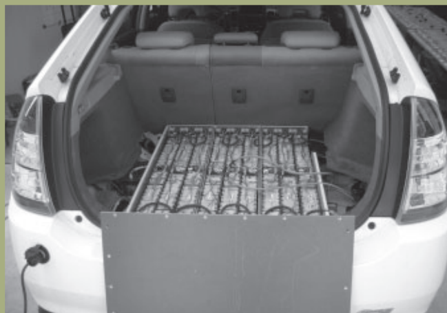
Lithium-ion battery pack developed by CalCars charges up in a PHEV, a converted Toyota Prius.
