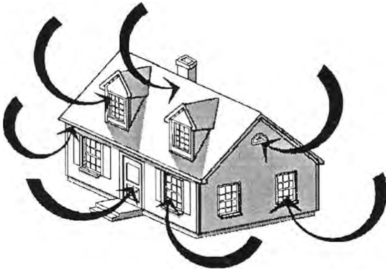
Figure 1.8-6. Home/structure noise entry points.
