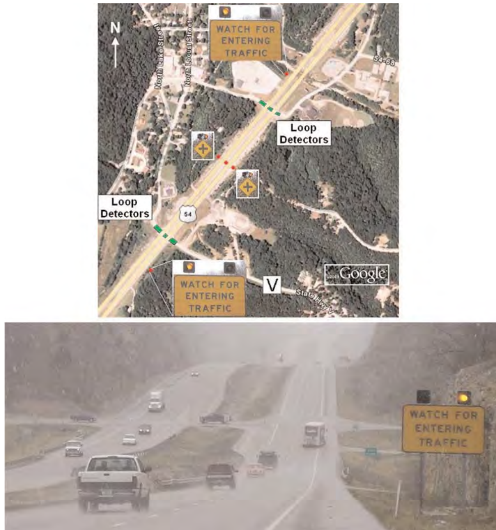
Figure 116. Dynamic advance intersection warning system deployed by MoDOT.
