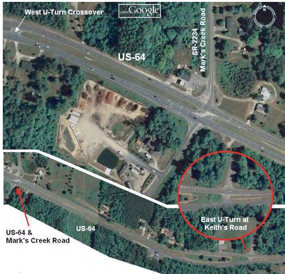
Figure 60. Aerial photo of J-turn intersection at US-64 and Mark's Creek Road.
