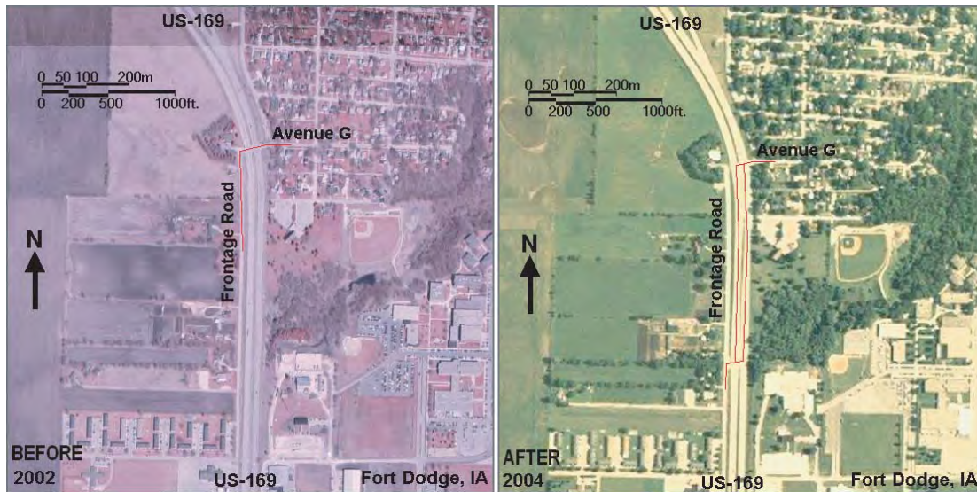
Figure 71. Before and after aerial photos of offset T-intersection in Fort Dodge, IA.
