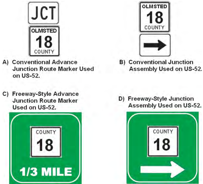
Figure 111. Examples of advance intersection guide signing along US-52 (before and after).
