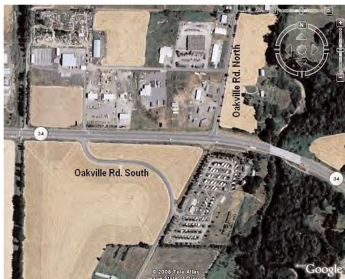
Figure 69. Aerial photo of offset T-intersection in Oregon.
