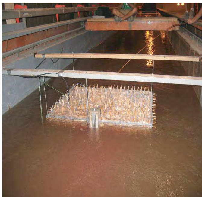
b. Downstream (note upwelling flow and dye dispersal)
