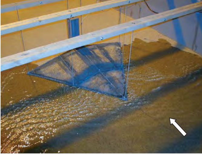
Figure 3.59. Buried wedge debris cluster placed on the bed showing initiation of flow during test.
