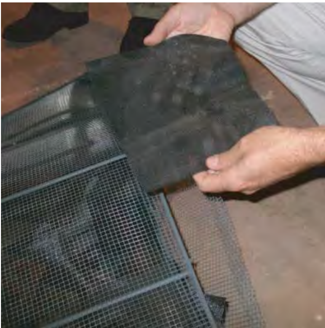
a. Woven geotextile used in filling debris clusters.
