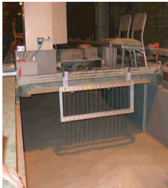
b. Transducer array used for automated scour hole mapping.
