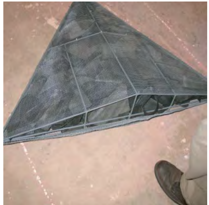
b. Wedge-shaped, impermeable debris cluster after being filled with geotextile.
