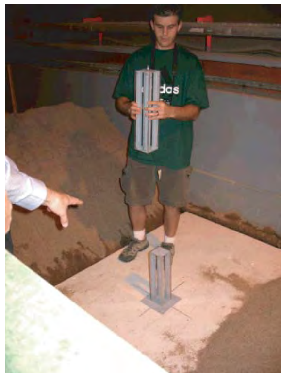
b. Four-inch square pier separated for data collection purposes.
