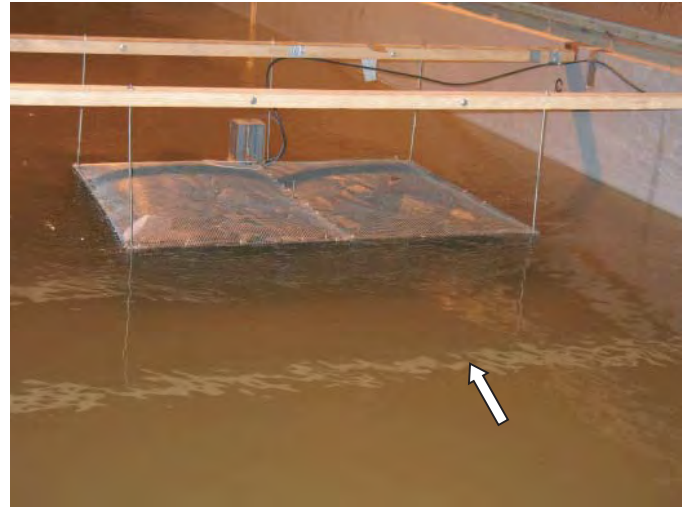
Figure 3.52. 4'W \times 3'L \times 8'H debris cluster located at the water surface during Test 004_03C.
