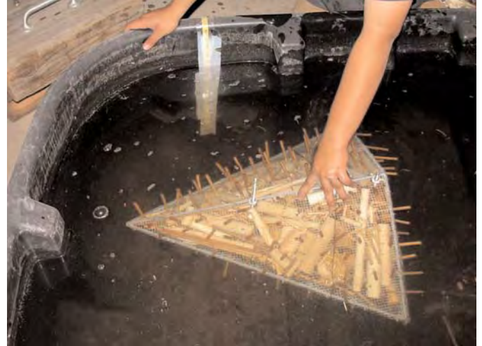
Figure 3.45. Determining porosity of debris cluster.
