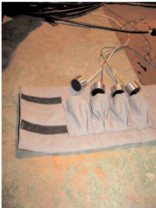
Figure 3.37. Transducers used for automated scour hole mapping.
