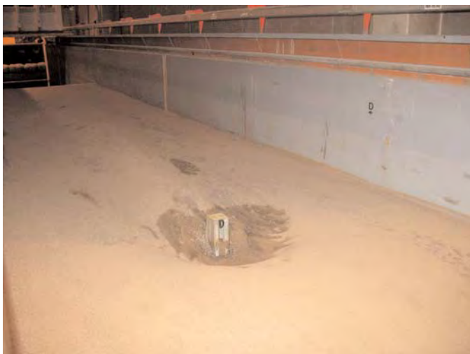
Figure 3.81. Pier D after Test 009_01, 72 hours at 1.0 V_{crit} .
