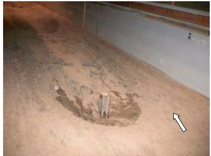
Ambient bed elevation is represented by the top of the pier. Upper segment of the pier and the debris configuration have been removed for data collection purposes.
