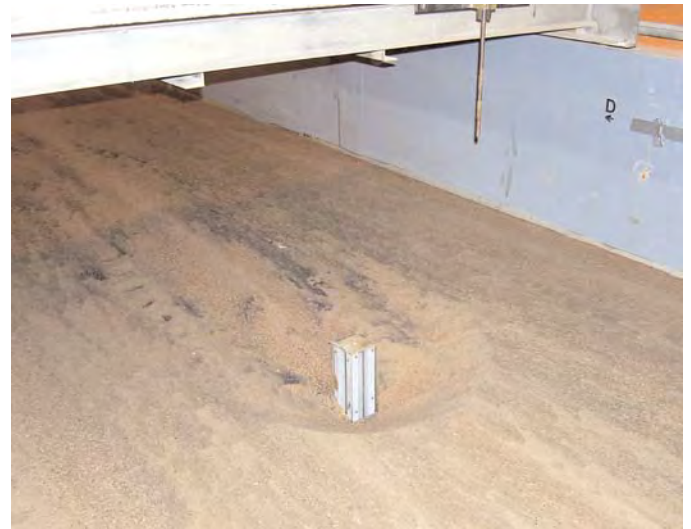
Figure 3.47. Square pier after 72-hour test with no debris (flow from right to left).
