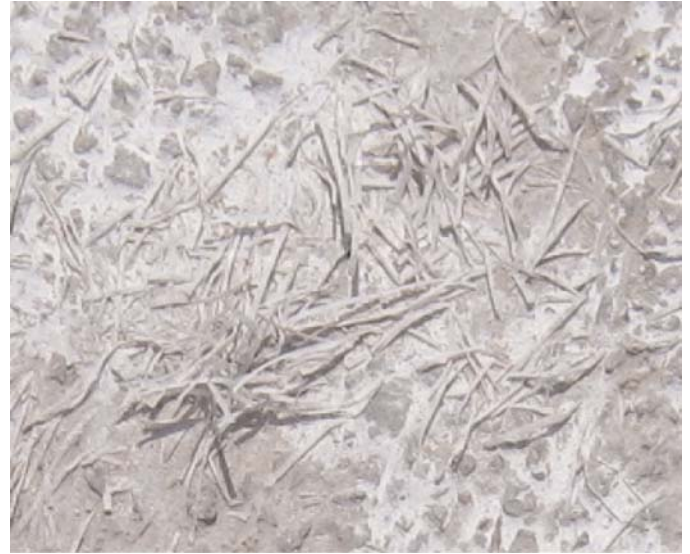
Figure 3.37. Left: Close-up of the interesting combination of EAC and fiber reinforcement, which creates a “fuzzy” appearance. Right: One of the challenges of using fibers in PCC is the so-called clumping, made more visible in the A99 panels because of EAC.
