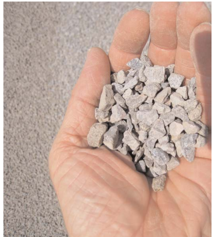
Figure 3.21. Top: Aggregate bins are double sided to accommodate aggregates for top-layer and lower-layer batches. Bottom left and right: Sand (0/2 mm) and crushed granite (4/8 mm) used as aggregates in the gap-graded, top-layer mix.
