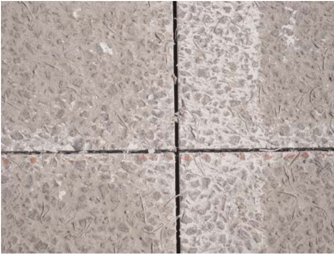
Figure 3.37. Left: Close-up of the interesting combination of EAC and fiber reinforcement, which creates a “fuzzy” appearance. Right: One of the challenges of using fibers in PCC is the so-called clumping, made more visible in the A99 panels because of EAC.
