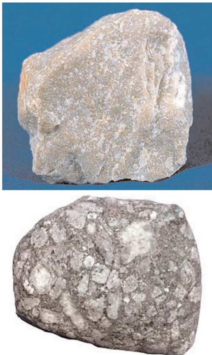
Figure 3.4. Top: A sample of gray quartzite, a high-quality aggregate used in EAC pavements, such as the N279 test sections in the Netherlands (12). Bottom: A hand specimen of diabase, an aggregate frequently encountered in EAC pavements along A1 in Austria (13).
