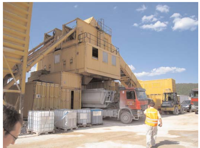
Figure 3.20. The concrete batching plant located near the A6 construction site is specifically designed for placement of two-layer PCC pavement.
