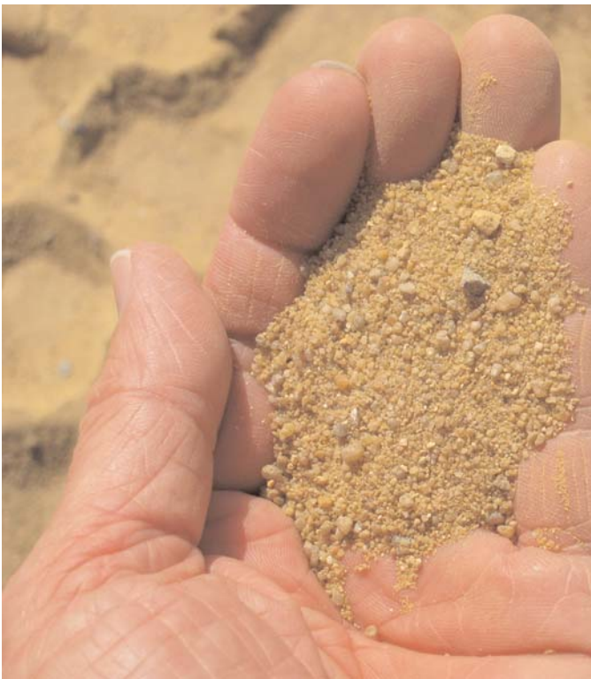
Figure 3.21. Top: Aggregate bins are double sided to accommodate aggregates for top-layer and lower-layer batches. Bottom left and right: Sand (0/2 mm) and crushed granite (4/8 mm) used as aggregates in the gap-graded, top-layer mix.
