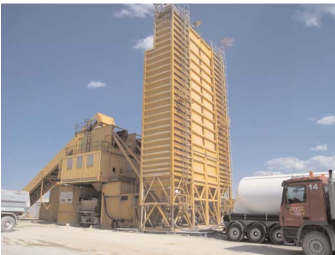
Figure 3.20. The concrete batching plant located near the A6 construction site is specifically designed for placement of two-layer PCC pavement.
