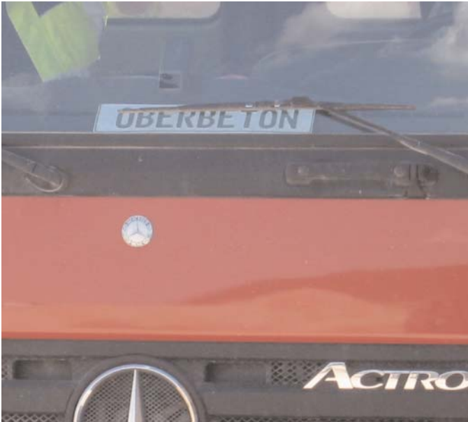
Figure 3.22. Plates on the dash of all trucks (left) allowed the batch plant manager to deliver appropriate layer mixes quickly and efficiently.
