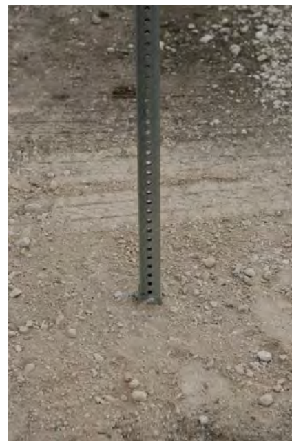
Figure 67. Perforated Square Steel Tubing Sign Support prior to Testing.
