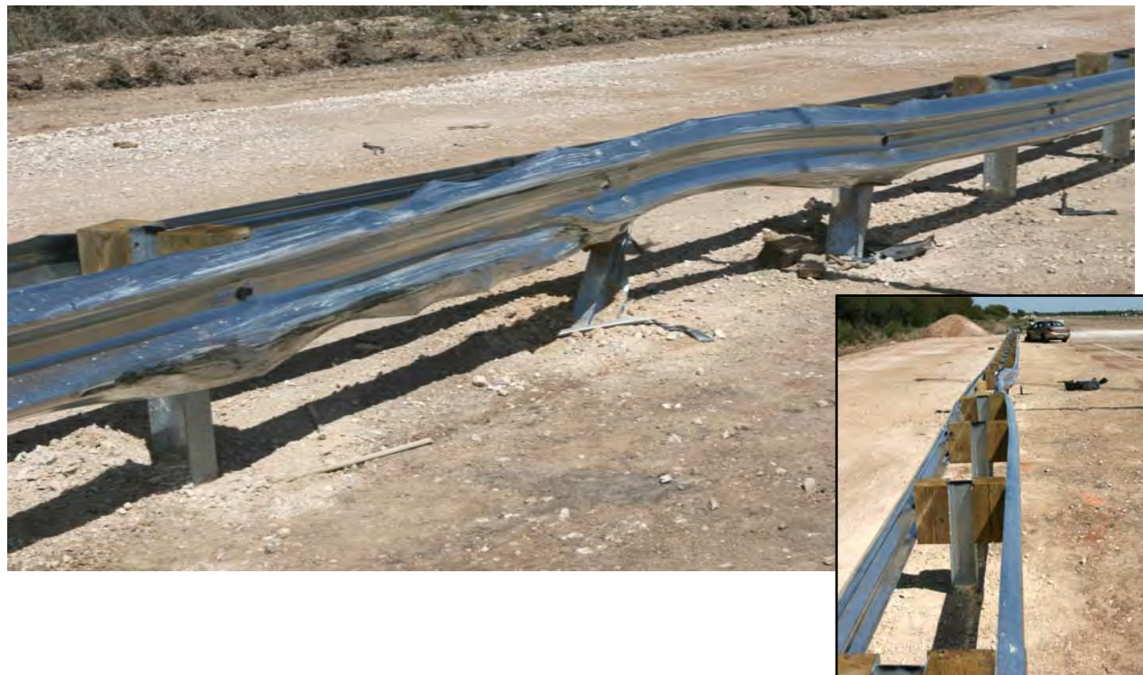
Figure 53. G4(1S) W-Beam Median Barrier after MASH Test 3-10.
