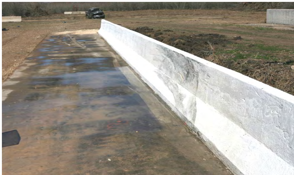
Figure 43. 32-inch New Jersey Shape Barrier after MASH Test 3-11.
