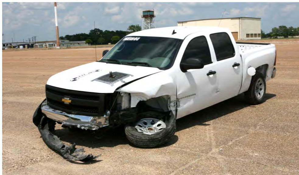
Figure 75. Test vehicle after MASH test 3-11 on the G3 weak post box-beam guardrail.
