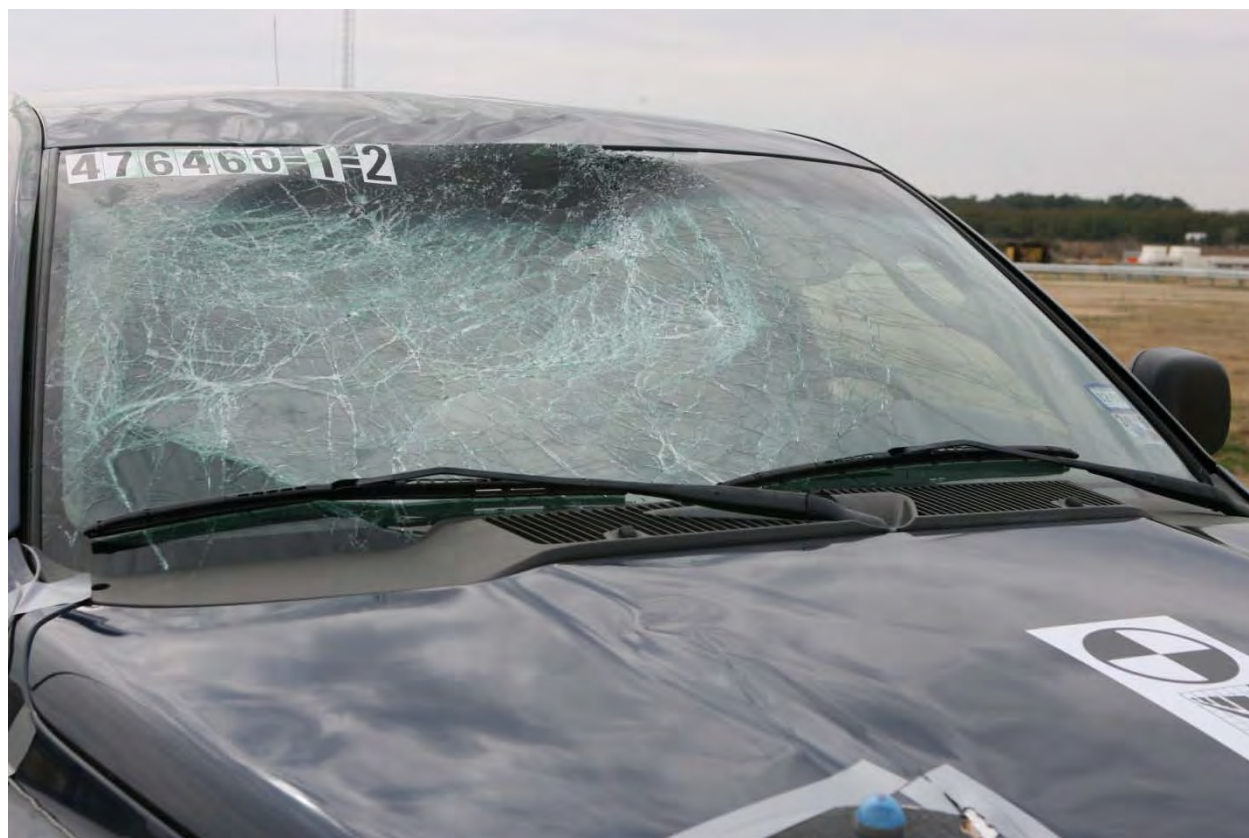
Figure 70. Vehicle after MASH Test 3-62 with Small Sign Supports.
