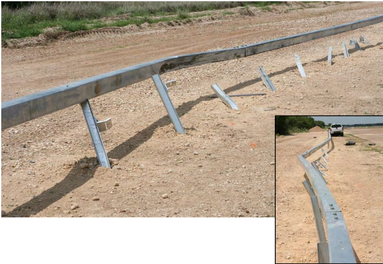
Figure 74. G3 Weak Post Box-Beam Guardrail after MASH Test 3-11.
