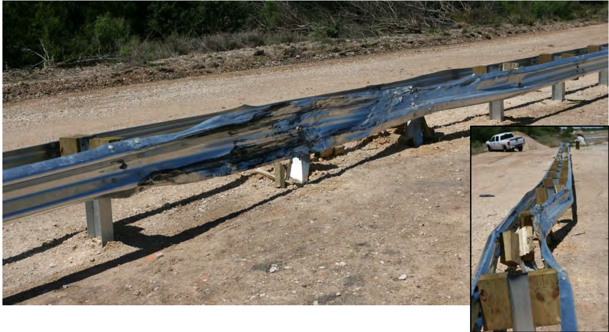
Figure 56. G4(1S) W-Beam Median Barrier after MASH Test 3-11.
