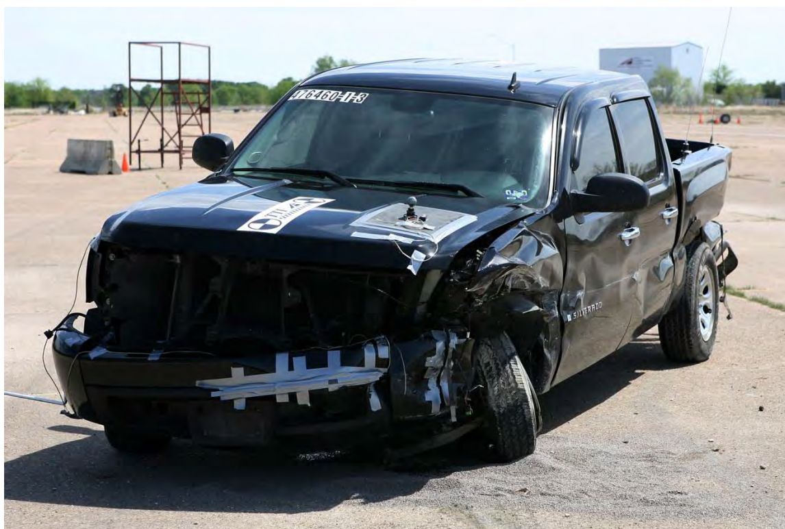
Figure 62. Test Vehicle after MASH Test 3-21 on the PennDOT W-Beam Transition.
