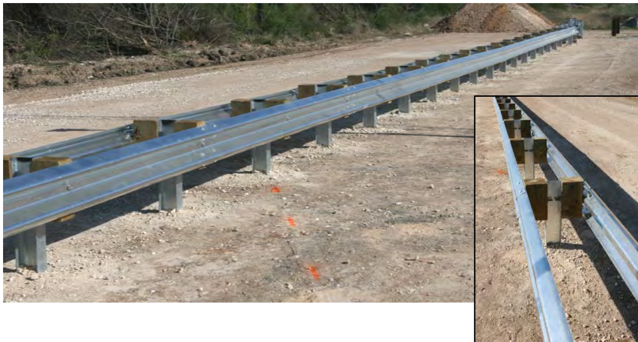
Figure 52. G4(1S) W-Beam Median Barrier Prior to Testing.
