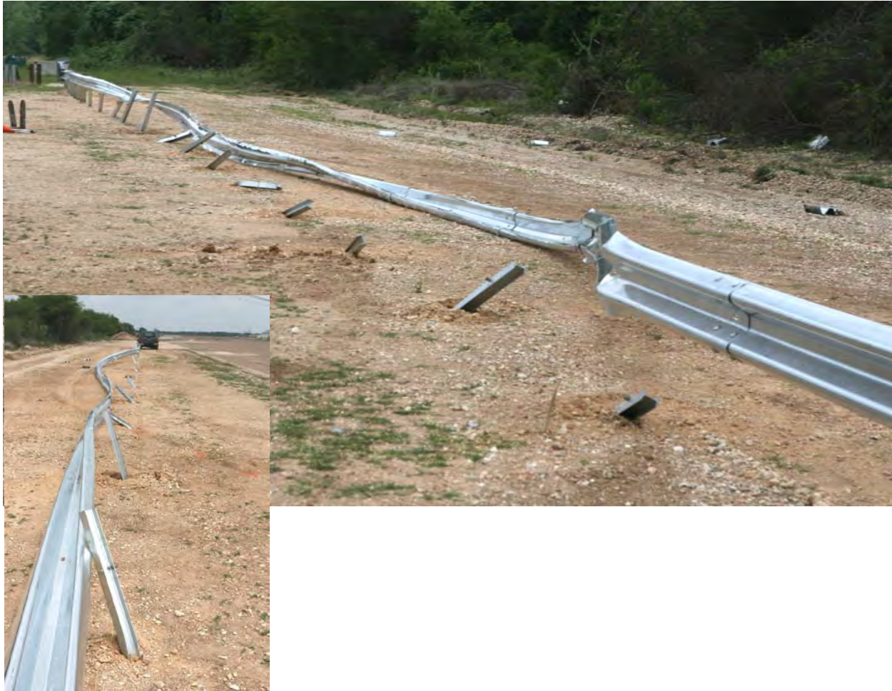
Figure 79. G2 Weak Post W-Beam Guardrail after MASH Test 3-11.
