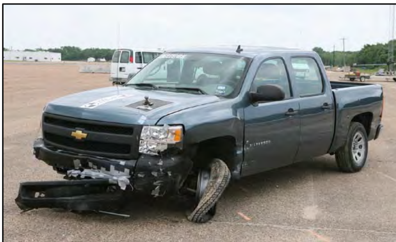
Figure 80. Test Vehicle after MASH Test 3-11 on the G2 Weak Post W-Beam Guardrail.
