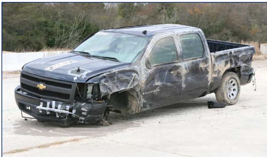
Figure 85. Test Vehicle after MASH Test 3-11 on the G9 Thrie Beam Guardrail.
