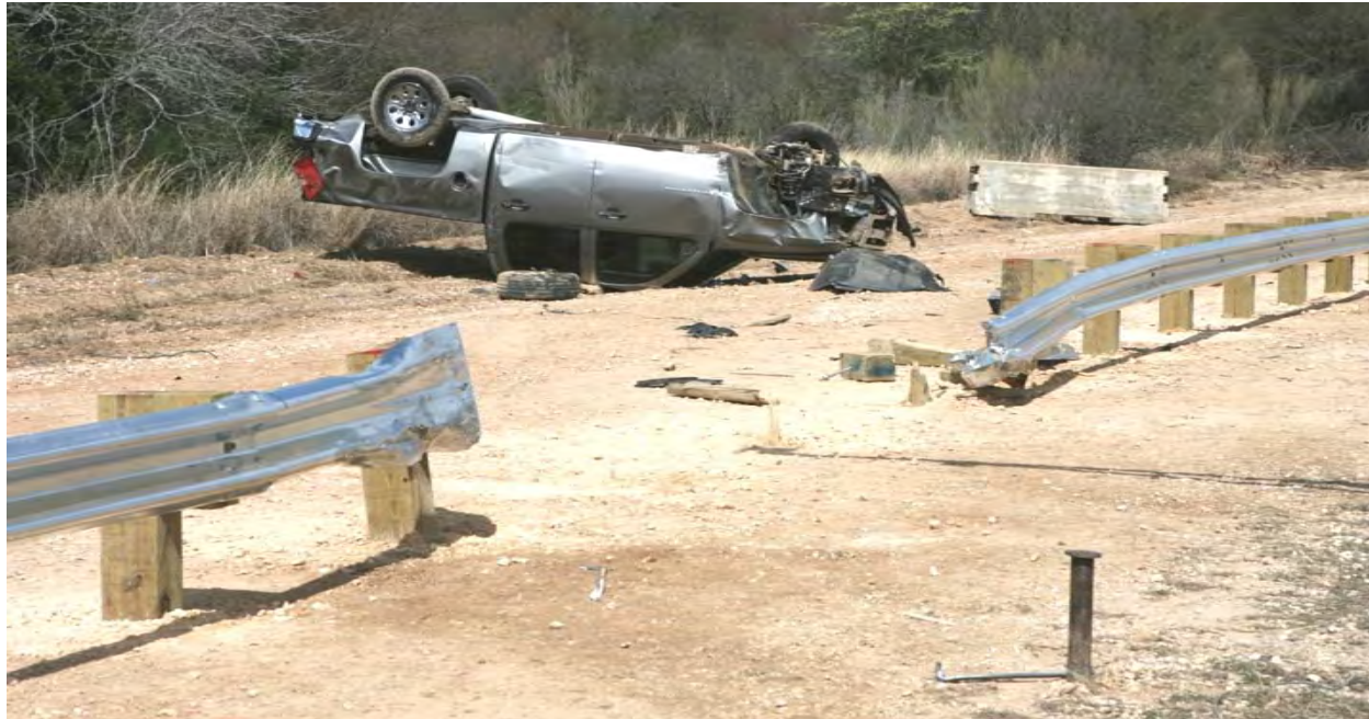
Figure 49. Test Vehicle and G4(2W) W-Beam Guardrail after MASH Test 3-11.
