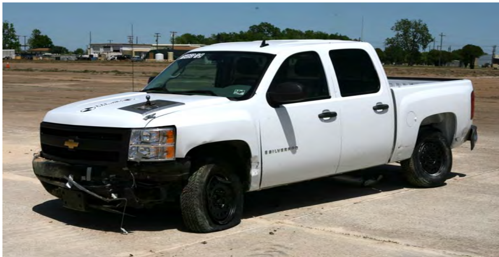
Figure 57. Test Vehicle after MASH Test 3-11 on the G4(1S) W-Beam Median Barrier.
