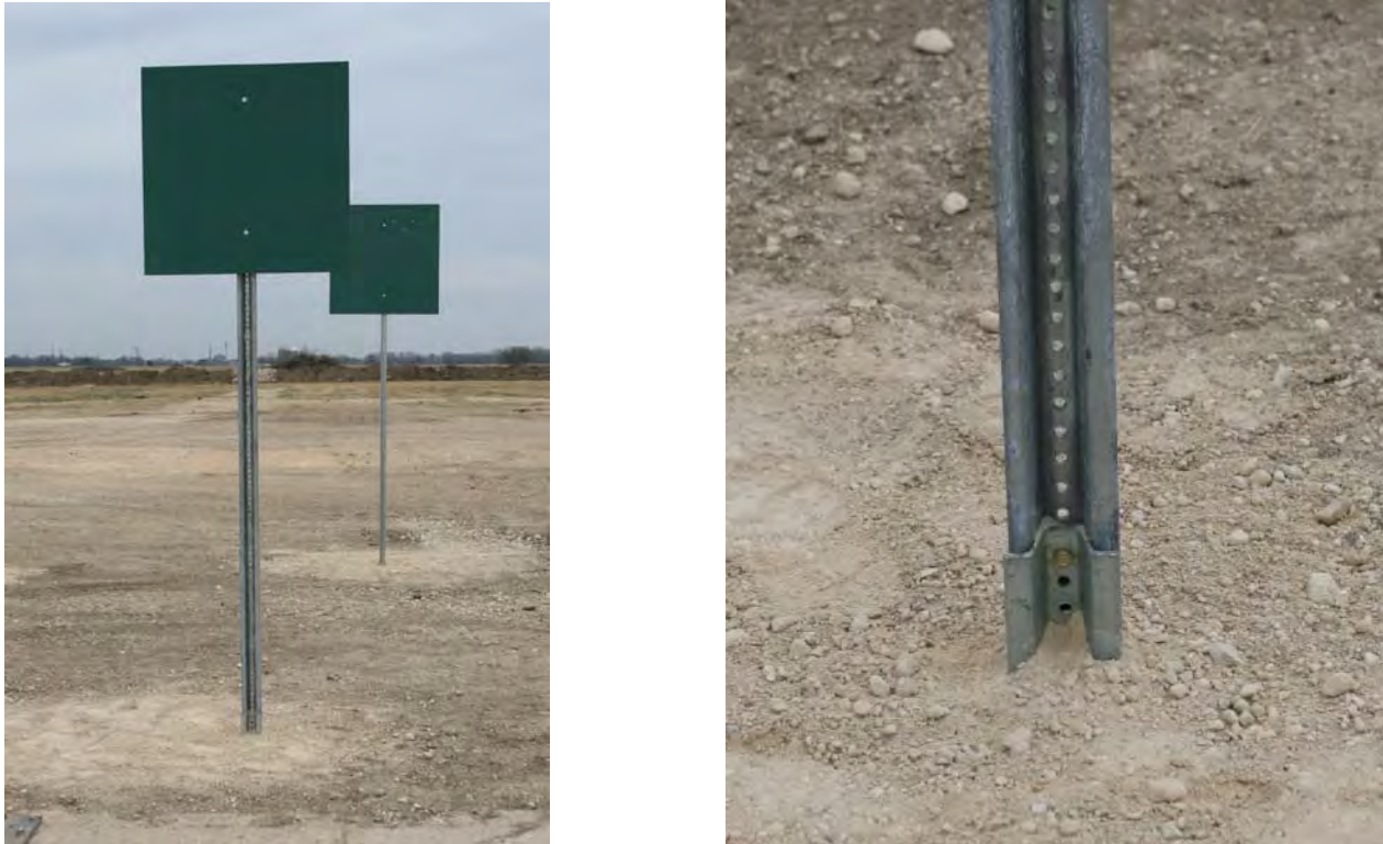
Figure 65. U-Channel Sign Support prior to Testing.
