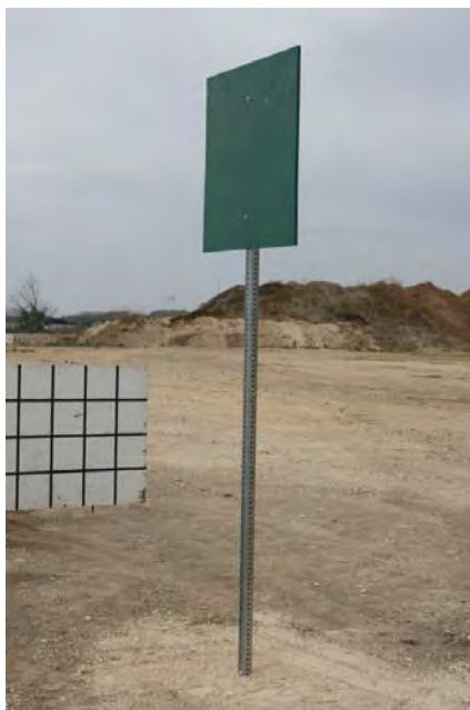
Figure 67. Perforated Square Steel Tubing Sign Support prior to Testing.
