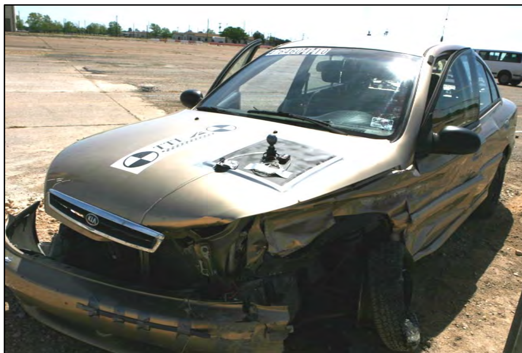
Figure 54. Test Vehicle after MASH Test 3-10 on the G4(1S) W-Beam Median Barrier.
