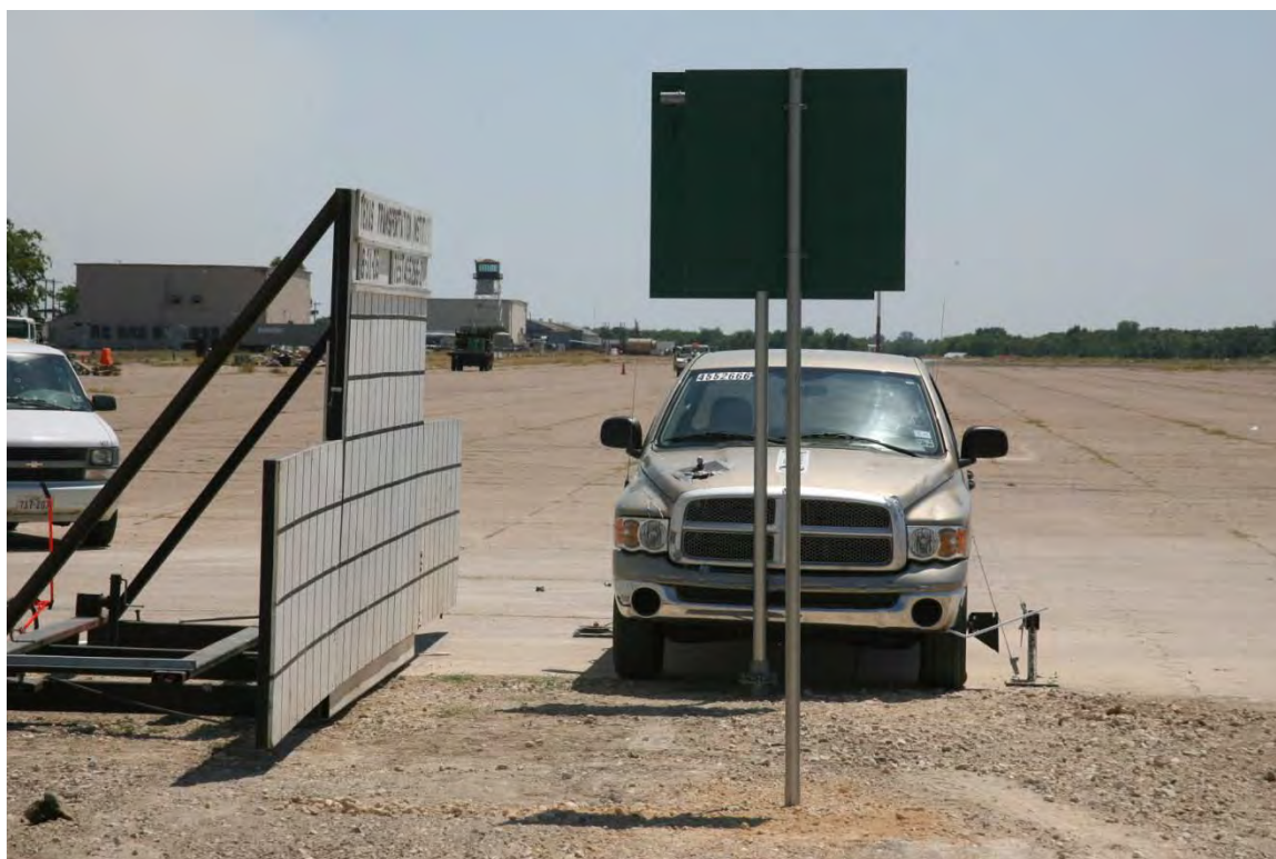
Figure 35. Vehicle/Installation Geometrics for Wedge Anchor & Triangular Slip Base Test.
