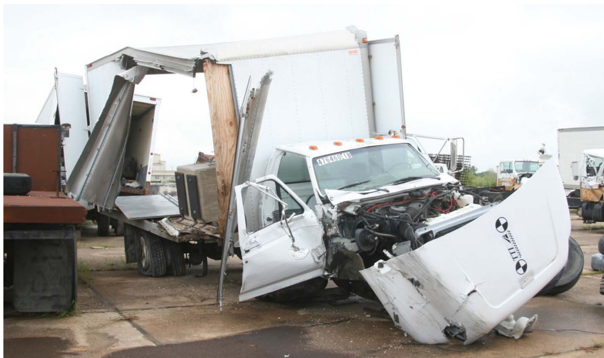
Figure 41. Test Vehicle after MASH test 4-12 on the 32-inch New Jersey Safety Shape Barrier.
