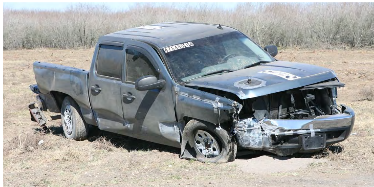
Figure 44. Test vehicle after MASH Test 3-11 on the 32-inch New Jersey Shape Barrier.
