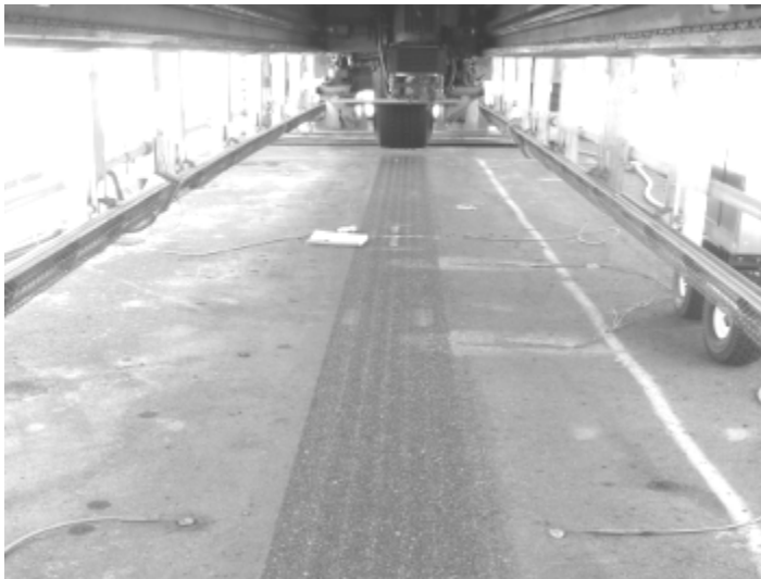
Figure 2-18. A typical HVS test section
