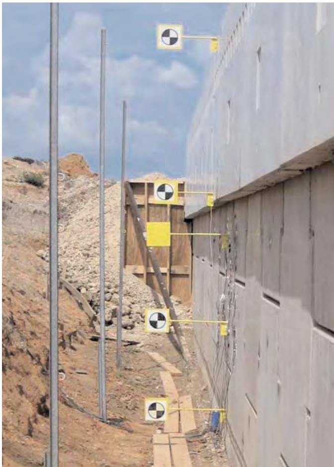
Figure 6.37. Location of displacement bars affixed on the barrier and panels.
