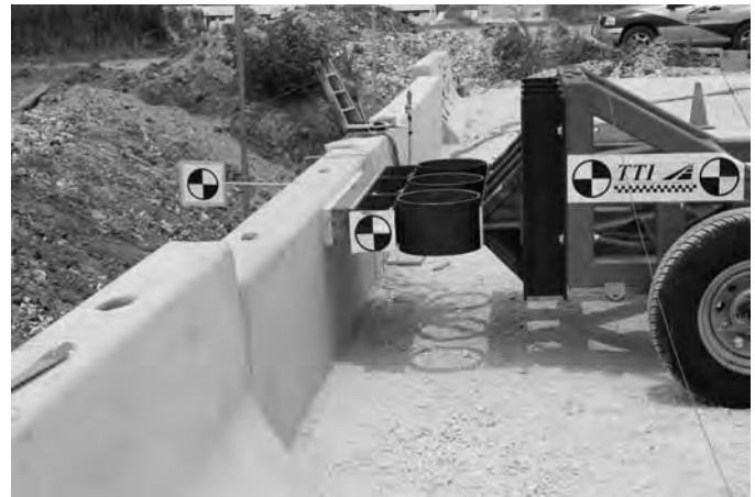
Figure 5.56. Test 2: vertical concrete barrier with 8 ft bar mats.
