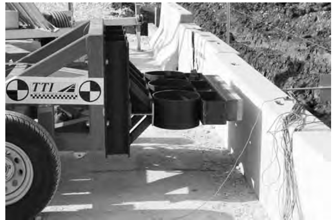
Figure 5.89. Test 4: Vertical wall barrier with 16 ft long strips.
