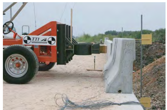
Figure 5.39. Bogie Test 1: N.J. barrier with 16 ft long strip.
