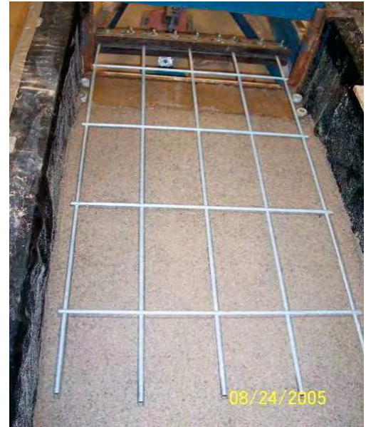
(b) Placing the bar mat on the sand
