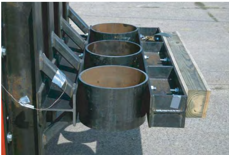
Figure 5.8. Detailed crushable cylinders of test bogie and numerical simulation.
