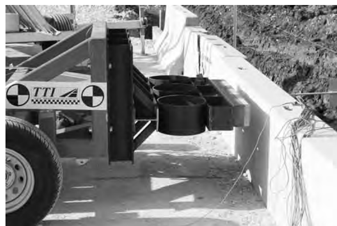
Figure 5.73. Test 3: Vertical wall barrier with 8 ft long strip.
