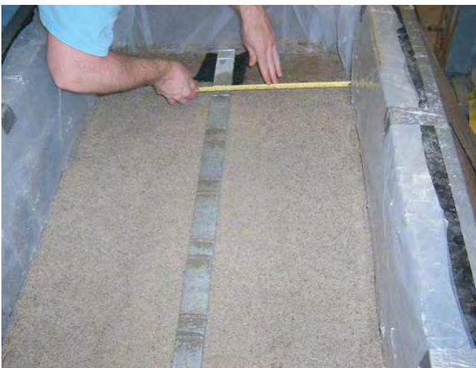
(e) Placing the strip on the sand
