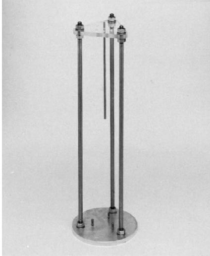
Figure 2-1- A 3-point caliper core measuring apparatus (courtesy of ASTM C 174 [3])
