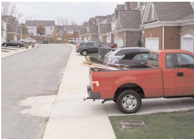
Exhibit 5-50. Insufficient driveway length leads to vehicles blocking the sidewalk.
