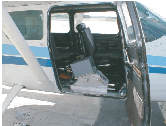
Figure 4.1 Example of a variable-tilt sensor mount. One method of achieving the dual-look approach is to fly the project area twice (once in each configuration) using a variable-tilt mount
