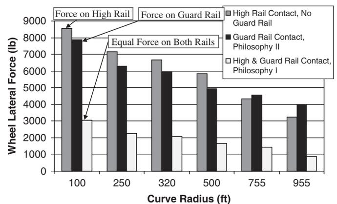
**Figure 4. The wheel lateral force of a Type 1 transit rail car with a guard rail.**
