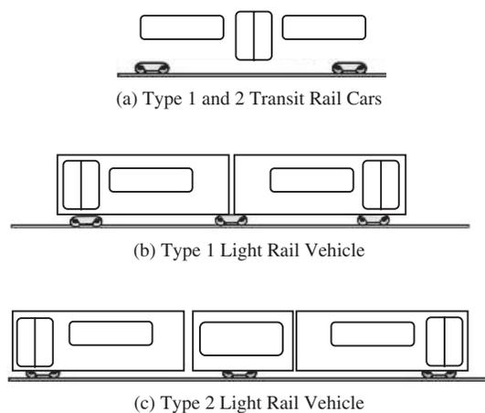
**Figure 3. Transit vehicles structures and layouts.**
