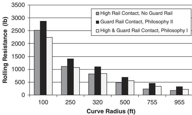
**Figure 5.** The vehicle rolling resistance of a Type 1 transit rail car with a guard rail.
