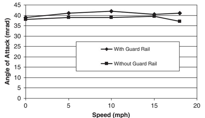
**Figure 10. Measured transit rail car leading axle AOA on TTL track.**
