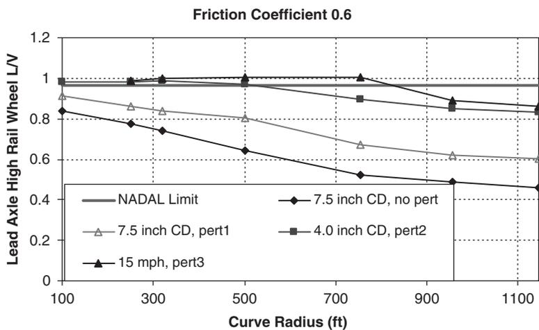
Figure 36. Wheel L/V ratio, Type 1 light rail vehicle, friction coefficient 0.6.
