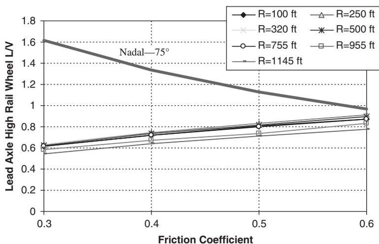
**Figure 38. Wheel L/V ratio, Type 2 light rail vehicle, Level 3 perturbations, 15 mph.**
