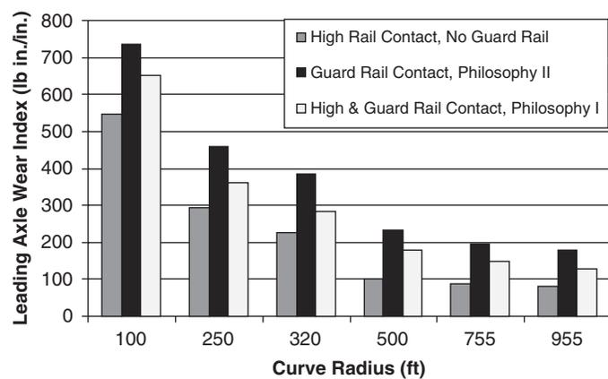
Figure 17. The wear index of a Type 1 light rail vehicle with a guard rail.
