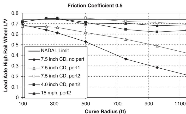
**Figure 26. The wheel L/V ratio of a Type 1 transit rail car with a 0.5 Friction Coefficient and a 63° Flange Angle.\***
