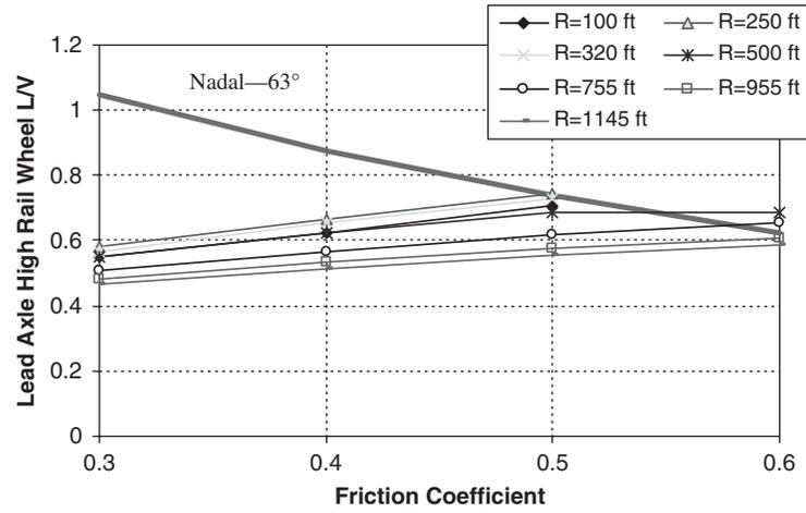
Figure 23. Wheel L/V ratio, Type 1 transit rail car, Level 2 perturbations 15 mph, no guard rail.
