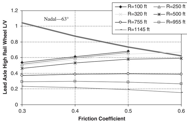
Figure 27. Wheel L/V ratio, Type 1 transit rail car, steady-state curving, 15 mph, worn rail.
