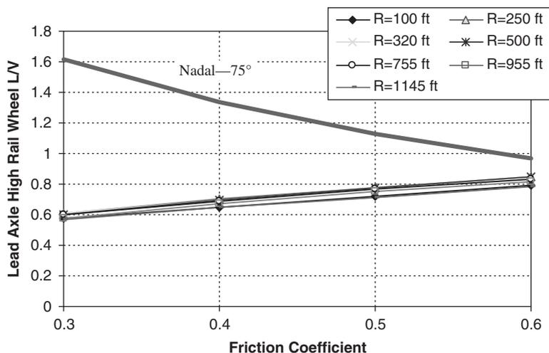
**Figure 32. Wheel L/V ratio, Type 1 transit rail car, 15 mph, 75° flange angle, perturbation Level 3.**
