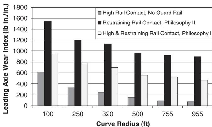
Figure 13. The wear index of a Type 1 transit rail car with a restraining rail.
