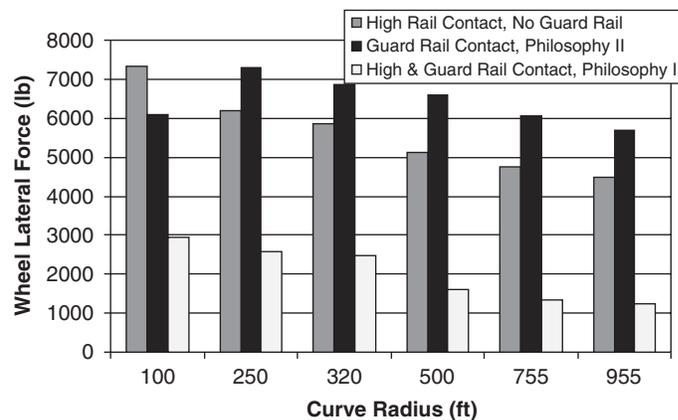
Figure 15. The wheel lateral force of a Type 1 light rail vehicle with a guard rail.
