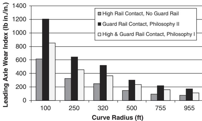
**Figure 8. The wear index of a Type 1 transit rail car with a guard rail.**
