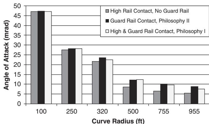
**Figure 18.** The axle AOA of a Type 1 light rail vehicle with a guard rail.
