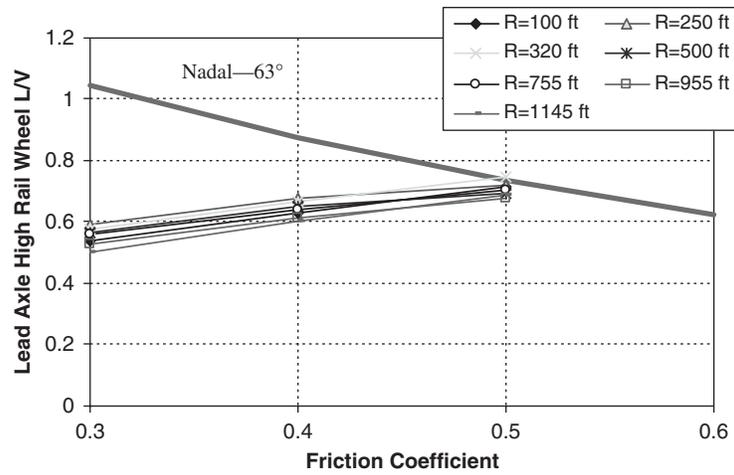
Figure 24. Wheel L/V ratio, Type 1 transit rail car, Level 3 perturbations 15 mph, no guard rail.
