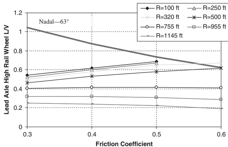
**Figure 22. Wheel LV ratio of a Type 1 transit rail car with steady-state curving 15 mph, no guard rail.**
