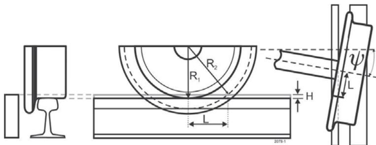
**Figure 6.** Wheel back/restraining rail contact.
