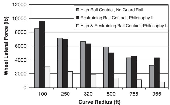
**Figure 11. The wheel lateral force of a Type 1 transit rail car with a restraining rail.**
