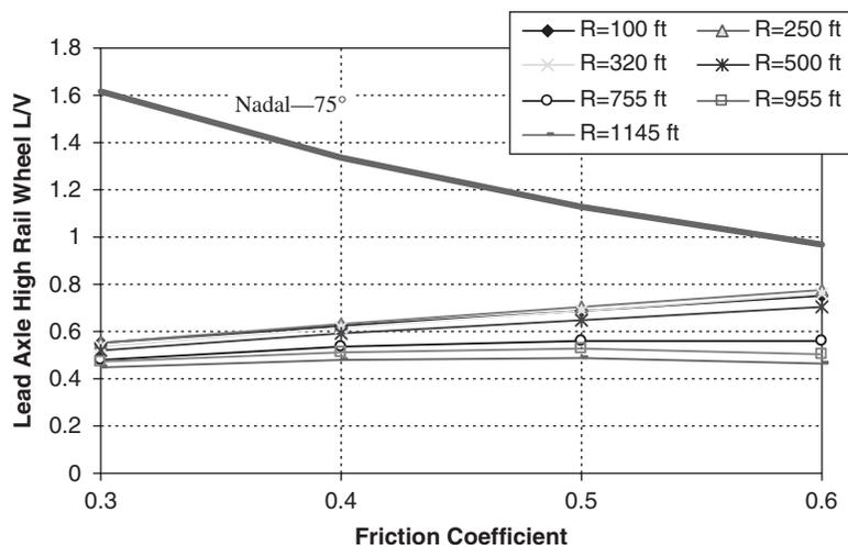
**Figure 30. Wheel L/V ratio, Type 1 transit rail car, 15 mph, 75° flange angle, steady-state curving.**
