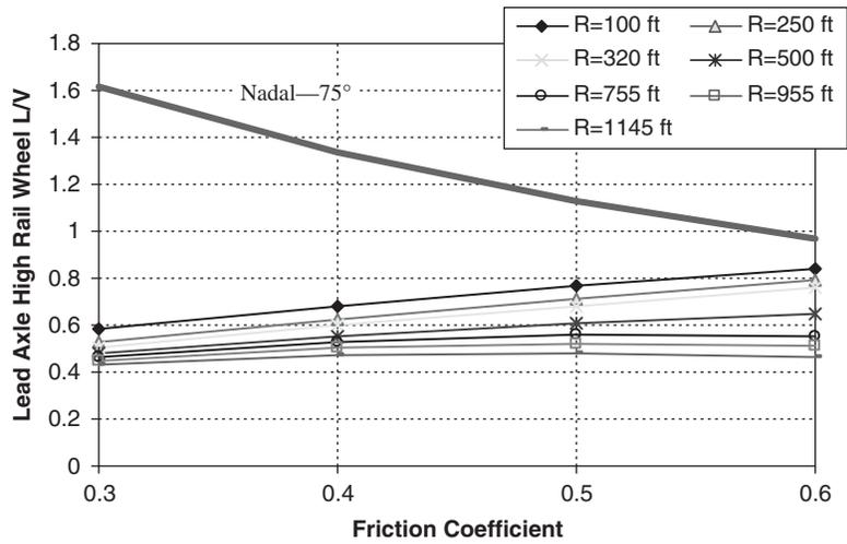
Figure 34. Wheel L/V ratio, Type 1 light rail vehicle, steady-state curving, 15 mph.
