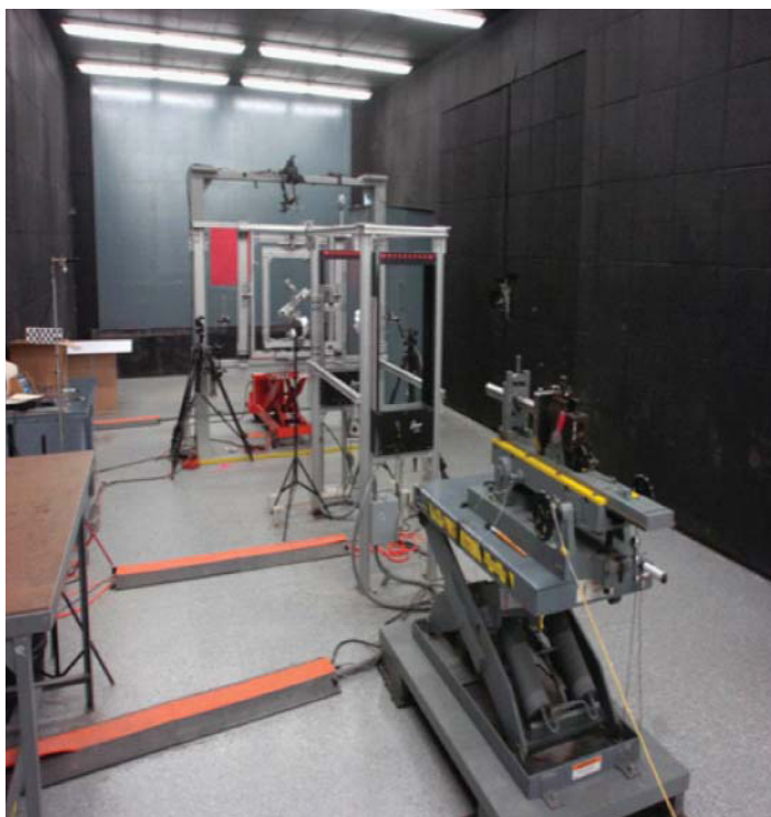
FIGURE 3 The body armor test range at ATC. SOURCE: John Wallace, Technical Director, ATC, “Body armor test capabilities,” Presentation to the committee, on March 10, 2010.
