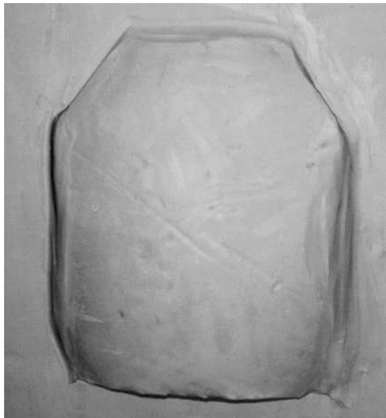
FIGURE 1 The clay appliqué applied to the clay box. SOURCE: Richard Sayre, Deputy Director, and Tracy Sheppard, Executive Officer and Staff Specialist, Office of the Secretary of Defense, Director of Operational Test and Evaluation (OSD DOT&E) Live Fire Test and Evaluation, “DoD in brief to the National Research Council study team,” Presentation to the committee, on November 30, 2009.
