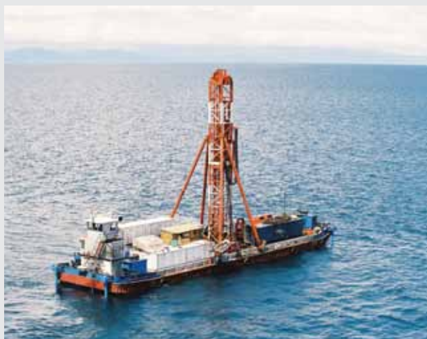
FIGURE 4.4 The drilling barge Viphya on Lake Malawi, East Africa in March 2005. Twenty-five scientists, drillers and mariners lived and worked aboard the vessel for 35 days, recovering long, continuous records from two sites in the lake—the longest a 385-m core from 600-m water depth (Scholz et al., 2006). SOURCE: Photograph courtesy of Jason Agnich.
