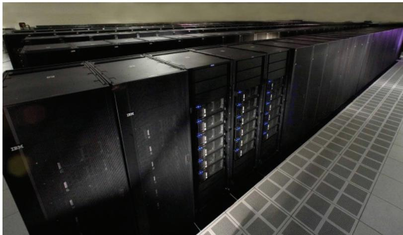
FIGURE 2-6 NNSA's ASC Roadrunner supercomputer was the first general-purpose supercomputer to reach a sustained petaflop. SOURCE: LeRoy N. Sanchez, Records Management, Media Services and Operations, Los Alamos National Laboratory ([http://www.lanl.gov/news/index.php/fuseaction/home.story/story\\_id/13602](http://www.lanl.gov/news/index.php/fuseaction/home.story/story_id/13602)). Image courtesy of Los Alamos National Laboratory.
