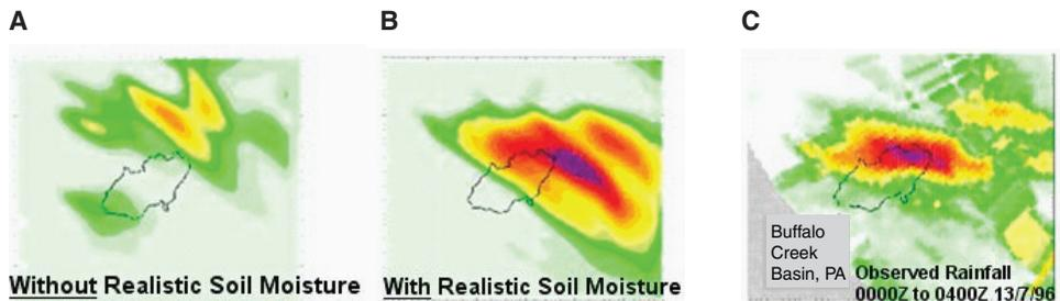
FIGURE 2.6 Soil moisture data improve numerical weather prediction over continents by accurately initializing land surface states. In this example, 24-hour prior forecasts of a high-resolution atmospheric model of rainfall are shown without (A) and with (B) soil moisture input data. The observed data are shown in panel C. Provided by the National Snow and Ice Data Center.
