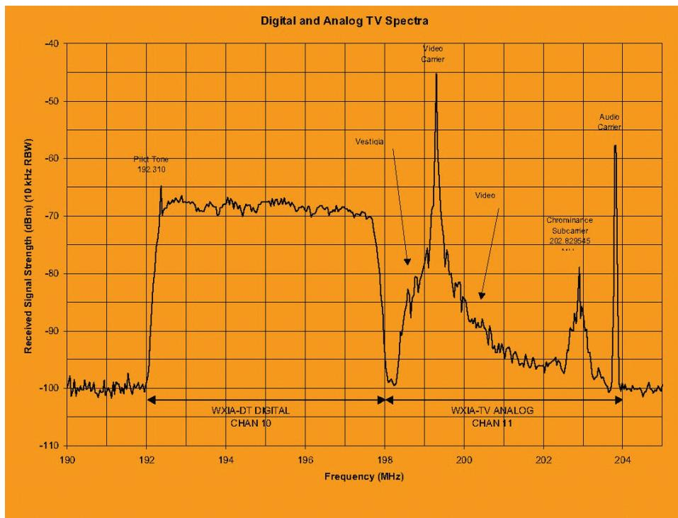
FIGURE 4.1 A comparison of the digital (Channel 10) and analog (Channel 11) television signals. The digital signal is essentially uniform in power across the entire channel, whereas the analog signal transmits most of its information in two narrow bands, leaving holes through which radio astronomers can sometimes observe relatively strong natural sources. Image courtesy of Andrew Clegg, National Science Foundation.
