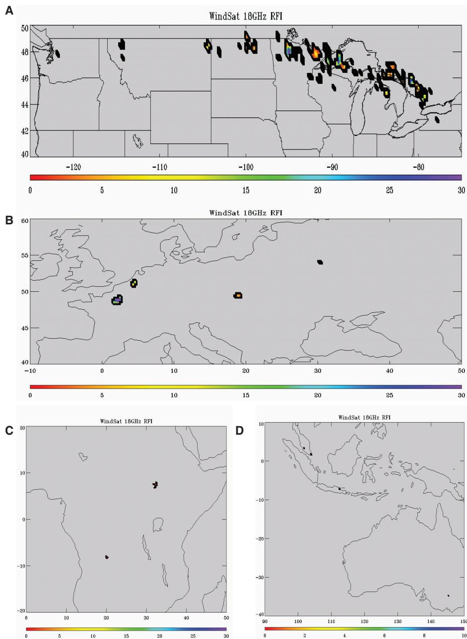
FIGURE 2.20 Cumulative analysis over a 5 year period of WindSat 18.6-18.8 GHz horizontally polarized data indicates sparse occurrences of strong radio frequency interference impacting 18 GHz brightness-temperature measurements over land: (A) North America, (B) Europe, (C) Central Africa, and (D) Southeast Asia/Oceania. Courtesy of the U.S. Naval Research Laboratory.
