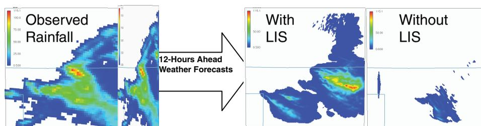
FIGURE 2.4 A depiction of the impact of observations of soil moisture (left) on 12-hour rainfall forecasts that use Weather Research and Forecasting models (for June 12, 2002). Panels at right: Forecasts with and without the Land Information System (LIS) providing improved soil moisture initial and boundary conditions. Image courtesy of NASA.
