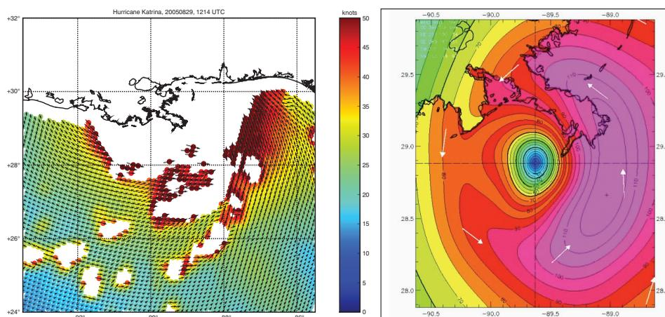
FIGURE 2.9 (Left) Image of the wind speed of Hurricane Katrina (in knots), observed by passive microwave radiometers on WindSat, a Naval Research Laboratory satellite, as Katrina makes landfall near New Orleans on August 28, 2005. (Right) Output from a model that combines data from WindSat and other remote sensing instruments. The model provides information on the hurricane's wind speed. The values over land are extrapolations. Courtesy of the U.S. Naval Research Laboratory.
