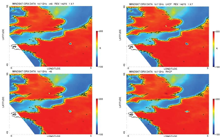
FIGURE 2.19 Brightness-temperature data from the WindSat 18.7  $\pm$ 45° channels (both left) and 18.7 R/LCP channels (both right) showing strong radio frequency interference over Paris and London. Courtesy of the U.S. Naval Research Laboratory.
