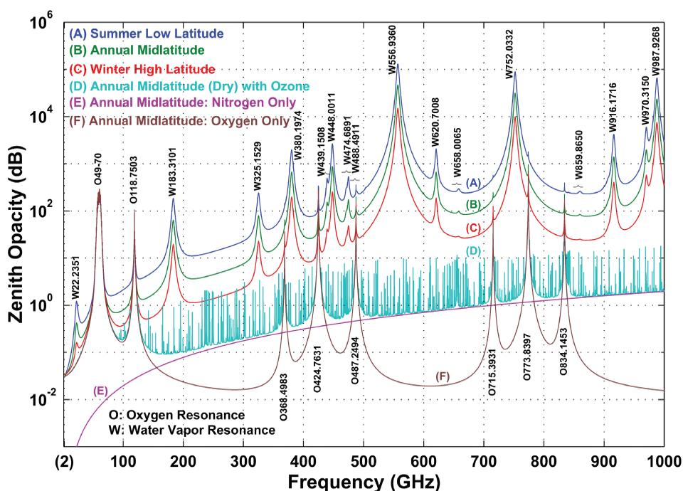
FIGURE 1.2 The opacity of Earth’s atmosphere in the radio range of frequencies from 1 to 1000 GHz for six scenarios. Image courtesy of A.J. Gasiewski, University of Colorado.
