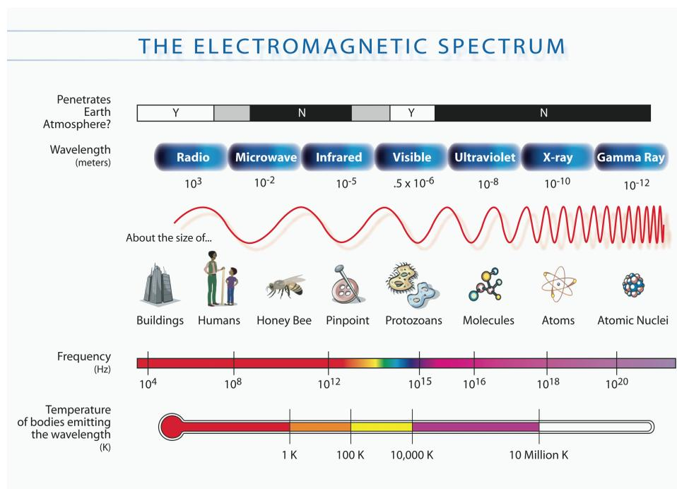
FIGURE 1.1 The characteristics of the electromagnetic spectrum. See Figures 1.2 and 1.3 in this chapter for a more detailed picture of the atmospheric penetration of electromagnetic waves. Image from NASA, *Science Program for NASA's Astronomy and Physics Division*, Washington, D.C., 2006.
