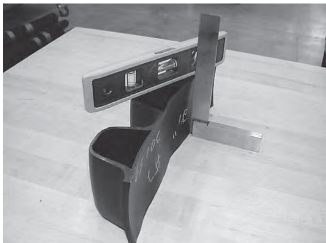
a. Check for Quality of Specimen Cuts
