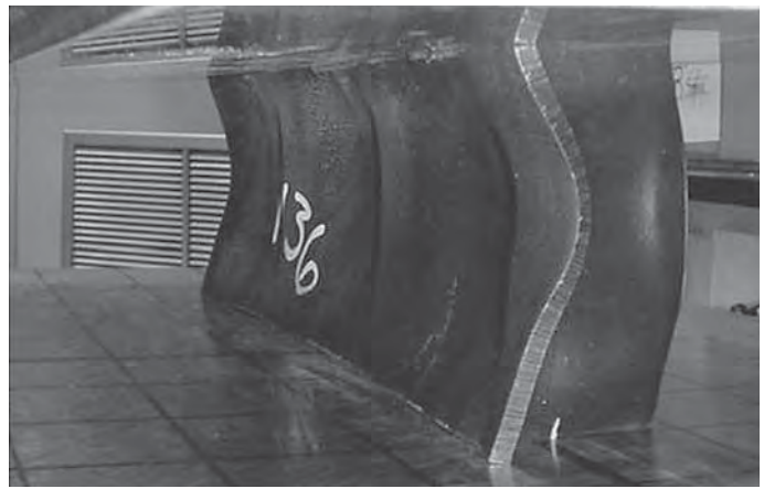
(b) Deformation of D36
