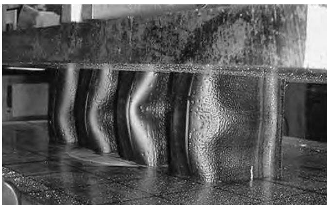
Figure 14. Corrugated HDPE pipe in stub compression test.
