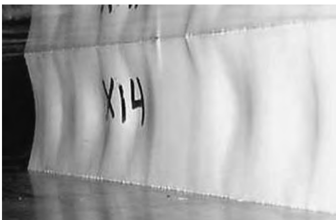
Figure B-11. Deformation in stub compression test for a PVC specimen.
