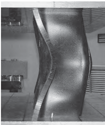
(c) Deformation of D60
