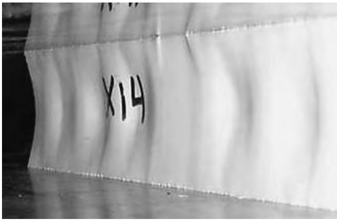
Figure 13. Corrugated PVC pipe in stub compression test.
