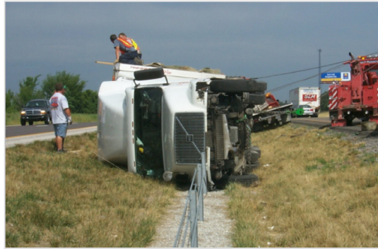
Cable median barrier prevented a truck from crossing a median.
