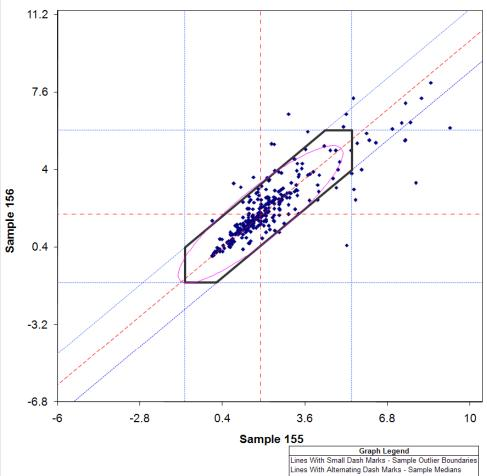
Lines With Small Dash Marks - Sample Outlier Boundar Lines With Alternating Dash Marks - Semple Medians Line With Large Dash Marks - Center Diagonal Black Hexagon - Data Within is Used for Analysis Ellipse - 2 Std Dev for Within and Between Lab Variation
