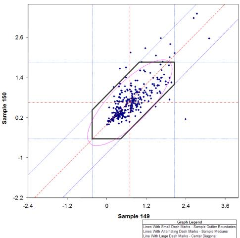
Line With Large Dash Marks - Center Diagonal Black Hexagon - Data Within is Used for Analysis Ellipse - 2 Std Dev for Within and Between Lab Variation
