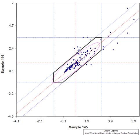
Lines With Small Dash Marks - Sample Outlier Boundarie Lines With Alternating Dash Marks - Sample Medians Line With Large Dash Marks - Center Diagonal Black Hexagon - Data Within is Used for Analysis Ellipse - 2 Std Dev for Within and Between Lab Variation
