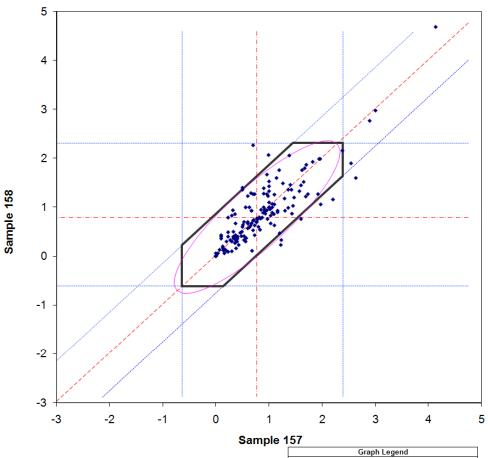
Graph Legend Lines With Small Dash Marks - Sample Outlier Boundaries Lines With Alternating Dash Marks - Sample Medians Line With Large Dash Marks - Center Diagonal Black Hexagon - Data Within is Used for Analysis Ellipse - 2 Std Dev for Within and Between Lab Variation
