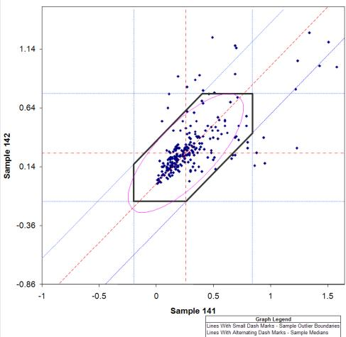
Line With Large Dash Marks - Center Diagonal Black Hexagon - Data Within is Used for Analysis Ellipse - 2 Std Dev for Within and Between Lab Variation Source of Data: AASHTO Materials Reference Laboratory Proficiency Sample Program
