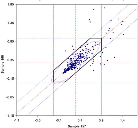
Graph Legend Lines With Small Dash Marks - Sample Outlier Boundaries Lines With Alternating Dash Marks - Sample Medians Line With Large Dash Marks - Center Diagonal Black Hexagon - Data Within is Used for Analysis Ellipse - 2 Std Dev for Within and Between Lab Variatio
