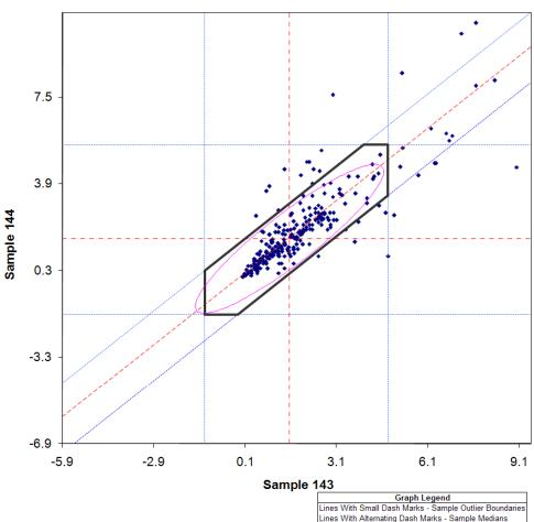
Lines With Small Dash Marks - Sample Outlier Boundaries Lines With Alternating Dash Marks - Sample Medians Line With Large Dash Marks - Center Diagonal Black Hexagon - Data Within is Used for Analysis Ellipse - 2 Std Dev for Within and Between Lab Variation
