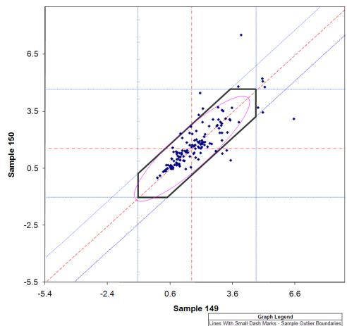
Lines With Alternating Dash Marks - Sample Medians Line With Large Dash Marks - Center Diagonal Black Hexagon - Data Within is Used for Analysis Ellipse - 2 Std Dev for Within and Between Lab Variation
