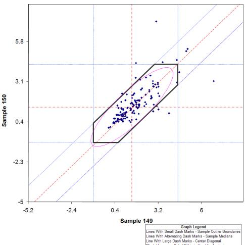
Black Hexagon - Data Within is Used for Analysis Ellipse - 2 Std Dev for Within and Between Lab Variation
