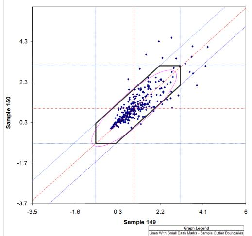
Lines With Alternating Dash Marks - Sample Medians Line With Large Dash Marks - Center Diagonal Black Hexagon - Data Within is Used for Analysis Ellipse - 2 Std Dev for Within and Between Lab Variatio
