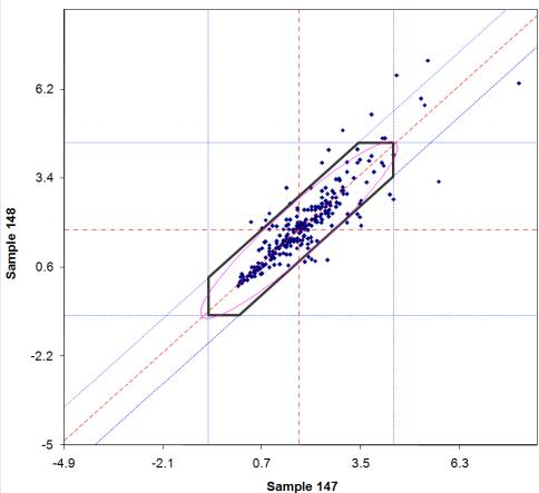
Graph Legend Lines With Small Dash Marks - Sample Outlier Boundaries Lines With Alternating Dash Marks - Sample Medians Line With Large Dash Marks - Center Diagonal Black Hexagon - Data Within is Used for Analysis Ellipse - 2 Std Dev for Within and Between Lab Variation
