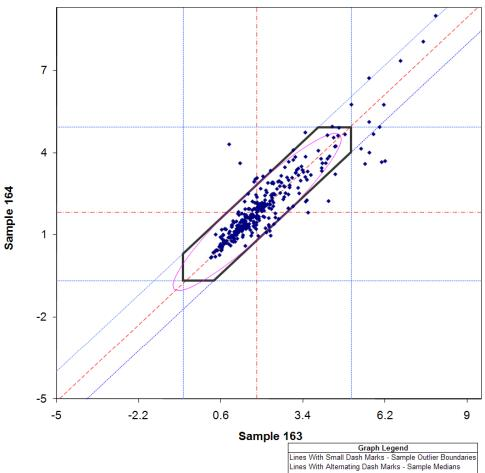
Line With Large Dash Marks - Center Diagonal Black Hexagon - Data Within is Used for Analysis Ellipse - 2 Std Dev for Within and Between Lab Variation
