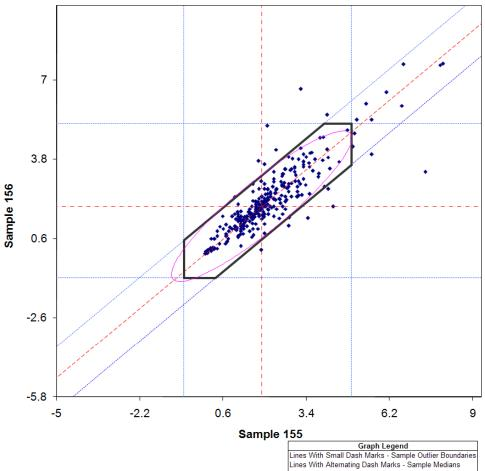
Lines With Small Dash Marks - Sample Outlier Boundari Lines With Alternating Dash Marks - Sample Medians Line With Large Dash Marks - Center Diagonal Black Hexagon - Data Within is Used for Analysis Ellipse - 2 Std Dev for Within and Between Lab Variation
