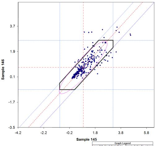
Lines With Small Dash Marks - Sample Outlier Boundaries Lines With Alternating Dash Marks - Sample Medians Line With Large Dash Marks - Center Diagonal Black Hexagon - Data Within is Used for Analysis Ellipse - 2 Std Dev for Within and Between Lab Variation
