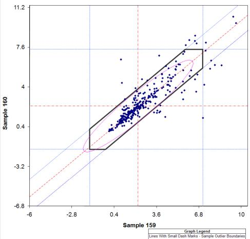
ines With Alternating Dash Marks - Sample Medians Line With Large Dash Marks - Center Diagonal Black Hexagon - Data Within is Used for Analysis Ellipse - 2 Std Dev for Within and Between Lab Variation
