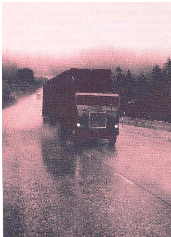
FIGURE 6 Wake of splash and spray thrown by 18 wheels.
