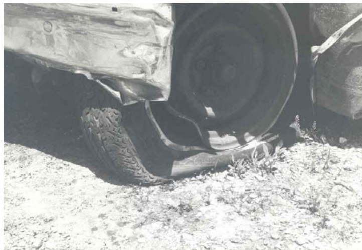
FIGURE 10 Rim damage and air out from high speed curb impact.
