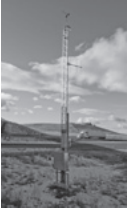
Roadway weather information system environmental sensor station in Idaho.
