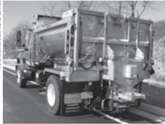
New truck equipped with radial dump spreader and salt slurry generator; state DOTs are ordering trucks with the features developed and tested for the HMCV.
