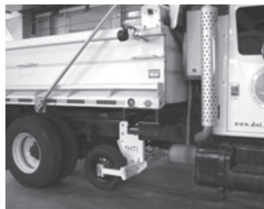
Friction wheel for measuring road grip under an Ohio DOT truck.
