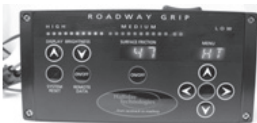
Ohio DOT sponsored research for the HMCV on friction-measuring equipment developed for use on racetracks.
