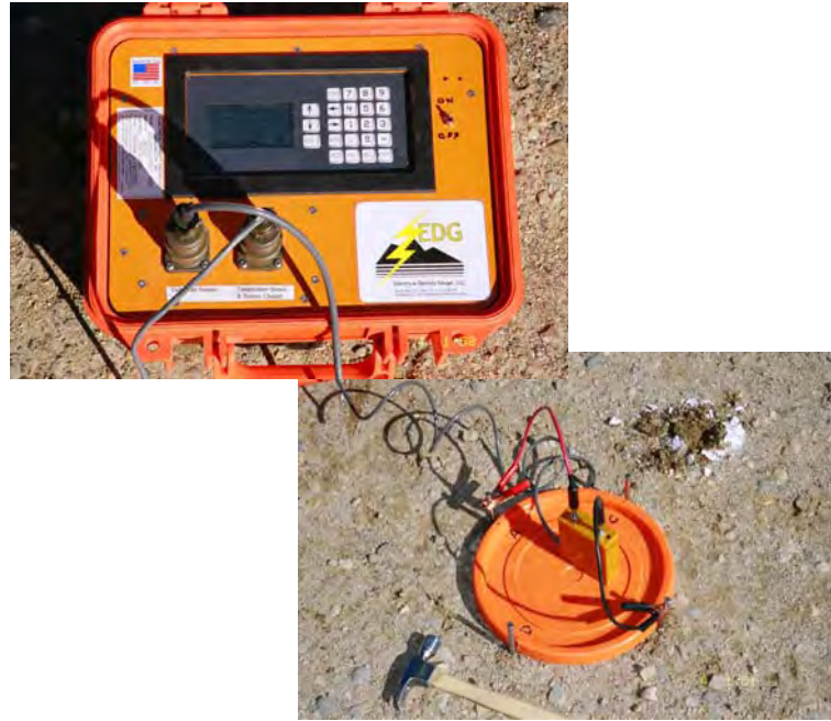
Figure 53. EDG Used to Measure the Density and Water Content of the Unbound Layers
