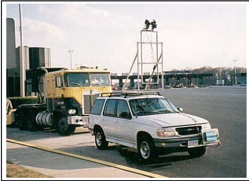
Figure 12. Infrared Camera Attached to Data Collection Vehicle
