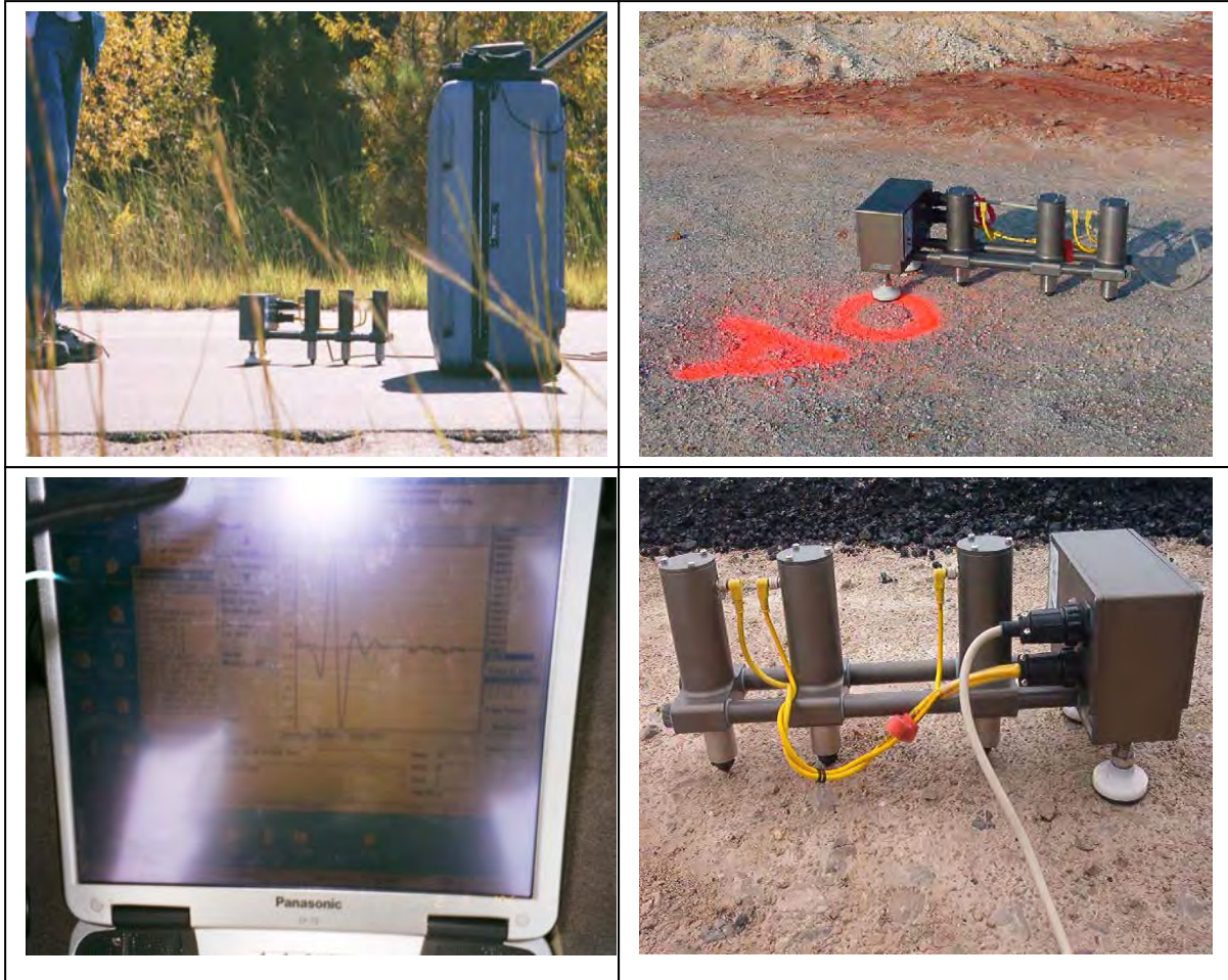
Figure 78. DSPA and PSPA Being Used to Test Different Materials
