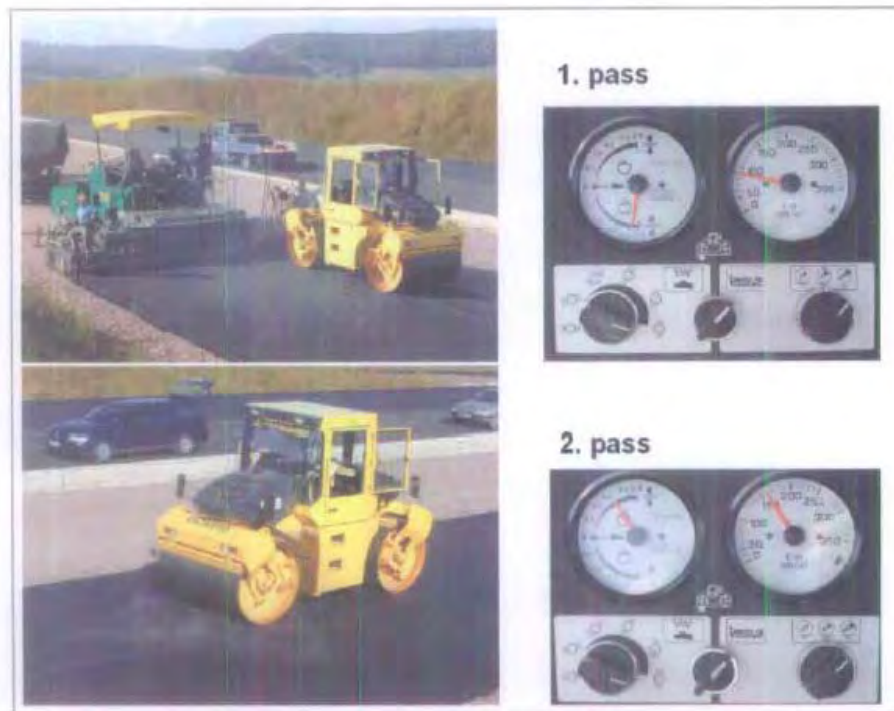
Figure 22. The Asphalt Manager from BOMAG
