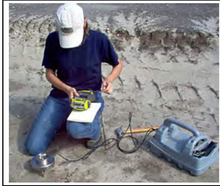
Figure 24. Photo of the Purdue TDR Method (courtesy of Durham Geo Website)
