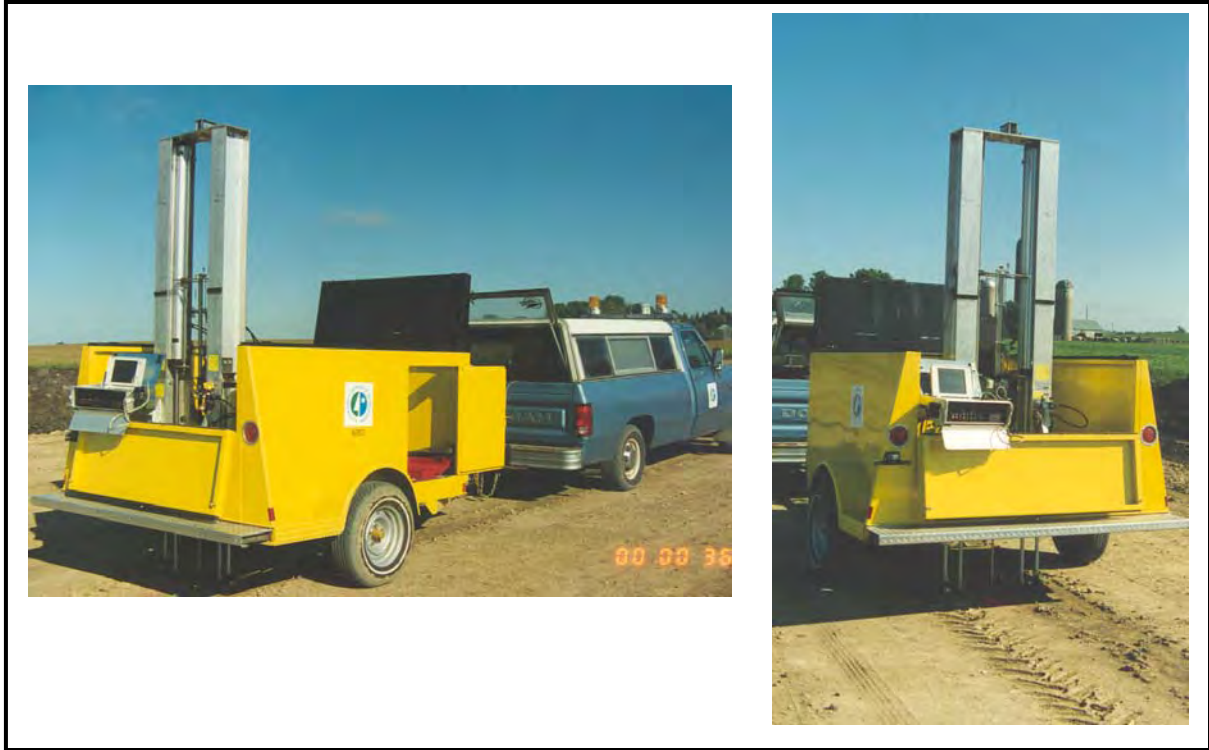
Figure 4. Automated DCP Attached to a Trailer (courtesy of Minnesota Road Research Section, Office of Materials, Minnesota DOT)
