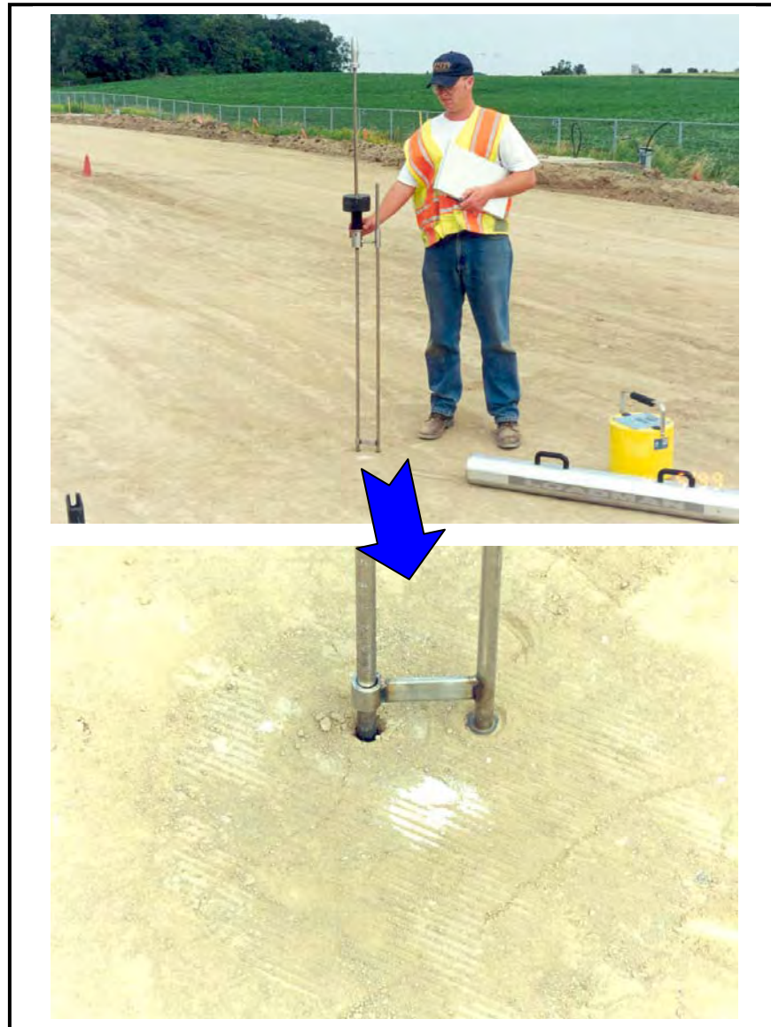
Figure 3. Photo of Manual DCP in Operation (courtesy of Minnesota Road Research Section, Office of Materials, Minnesota DOT)
