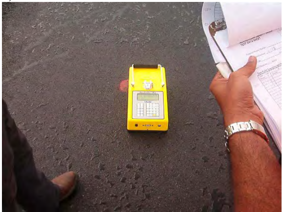
c) and d) Non-nuclear density testing with multiple devices after rain in 24 hours
