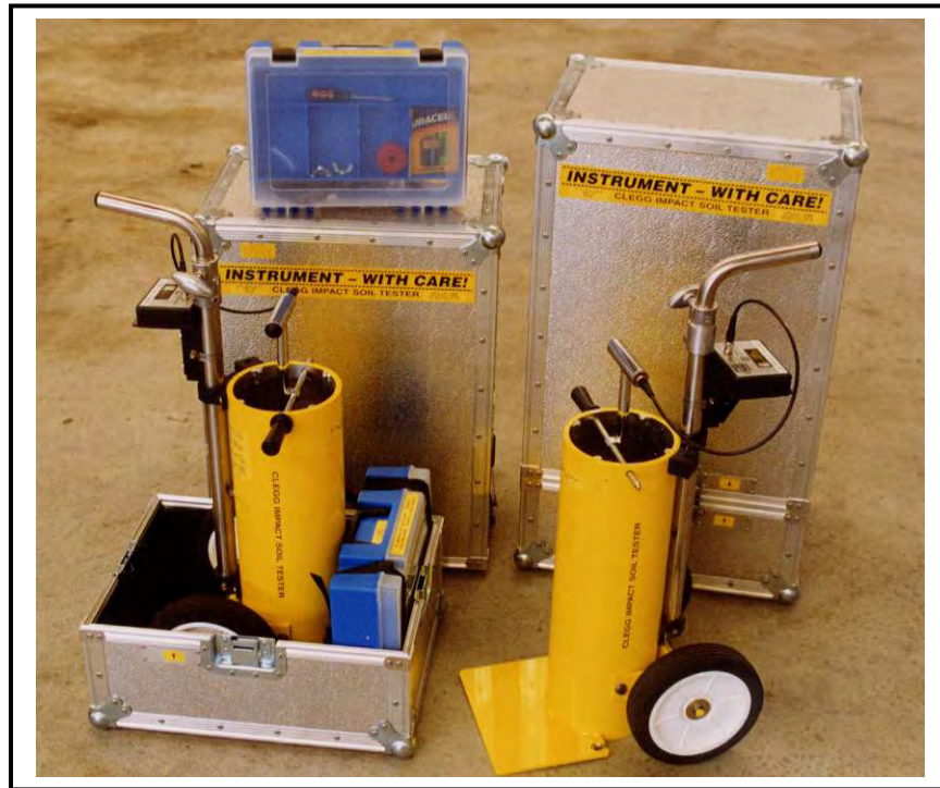
Figure 5. Photo of the Clegg Impact Soil Tester (courtesy of SDi WebSite)
