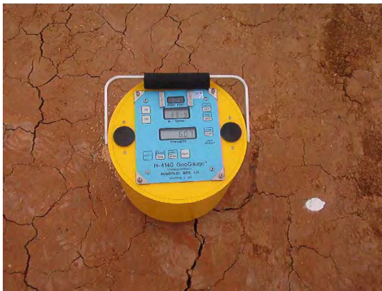
d) Geogauge testing on subgrade soil
