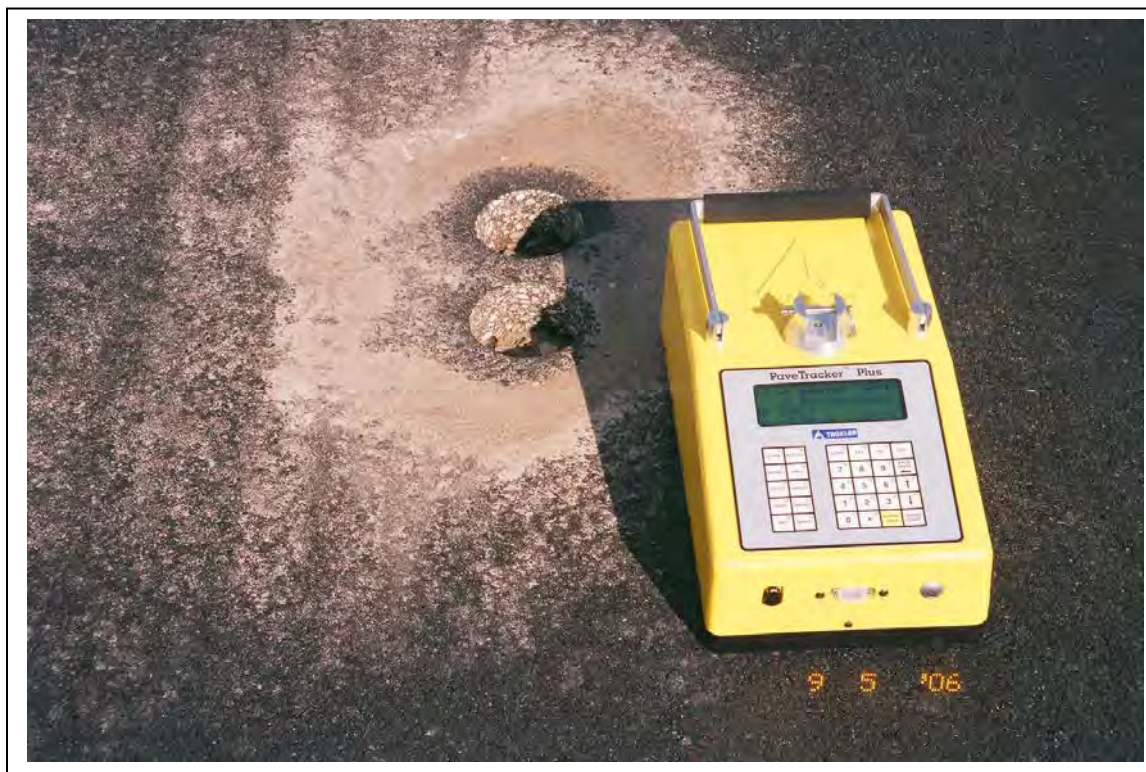
Figure B.55. The PSPA and Non-Nuclear Density Gauges Were Used to Test the HMA Base and Other Mixtures in the Areas Where the North Dakota DOT and Contractor Took Cores for QA Purposes
