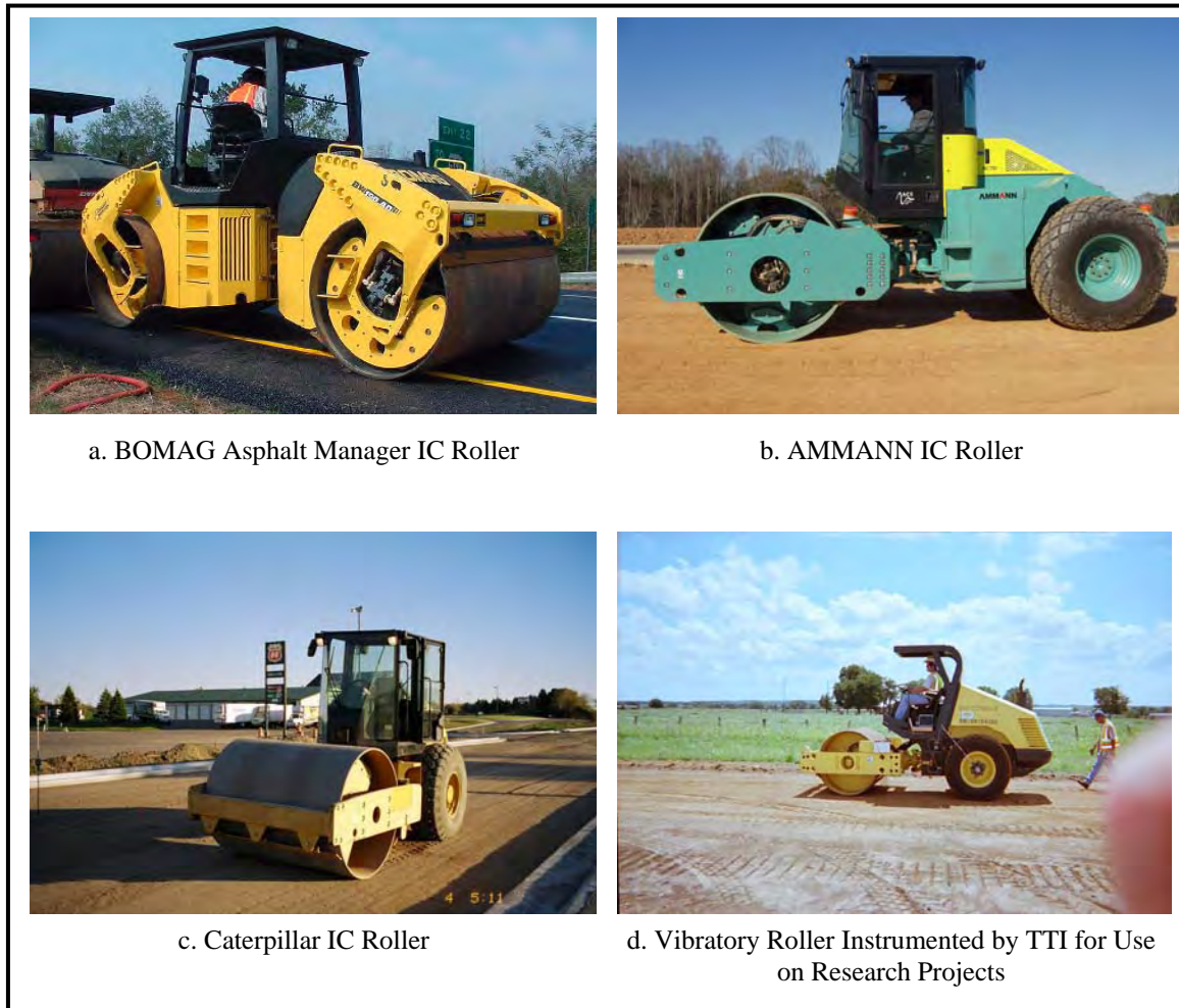
Figure 19. Fully Equipped Rollers Measuring the Stiffness of the Material Being Compacted
