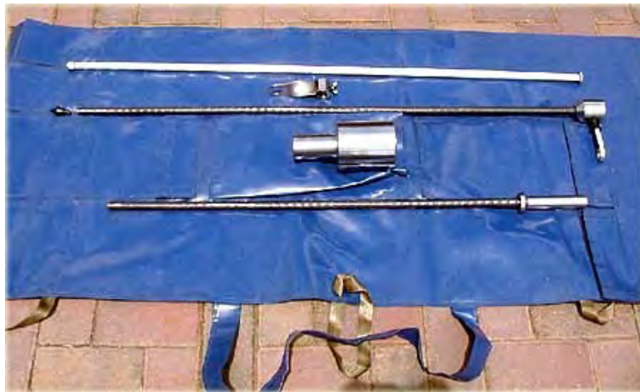
Figure 81. The DCP Before Assembly for Use in Measuring the In-Place Strength of Unbound Materials and Layers
