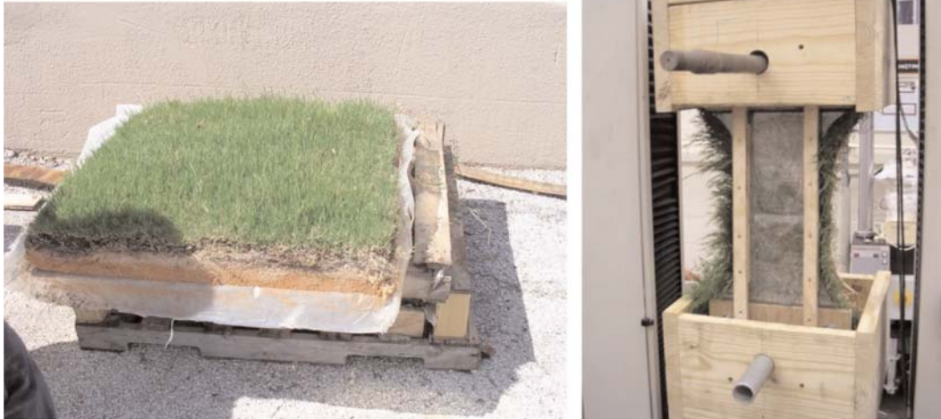
Figure 10-11. Reinforced turf material (left) and dog-bone specimen in tensile test jig (right).
