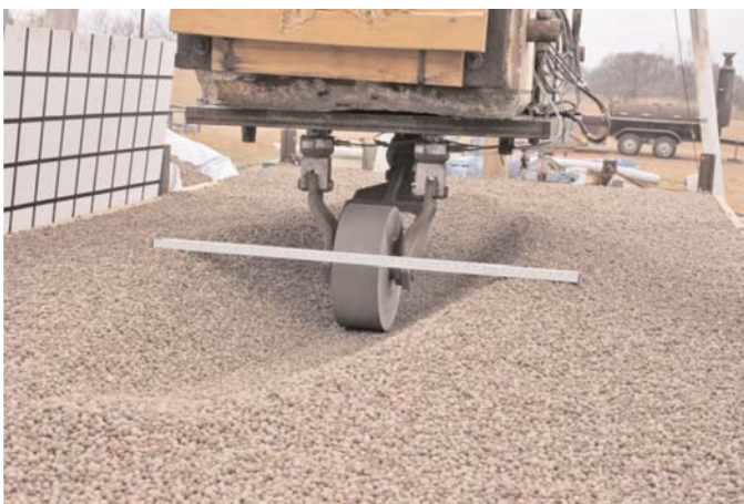
Figure 10-9. Post-test view of rut in engineered aggregate created by pendulum wheel.
