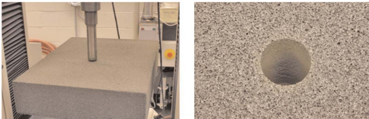
Figure 9-9. Punch test of glass foam test specimen pre-test (left) and post-test (right).
