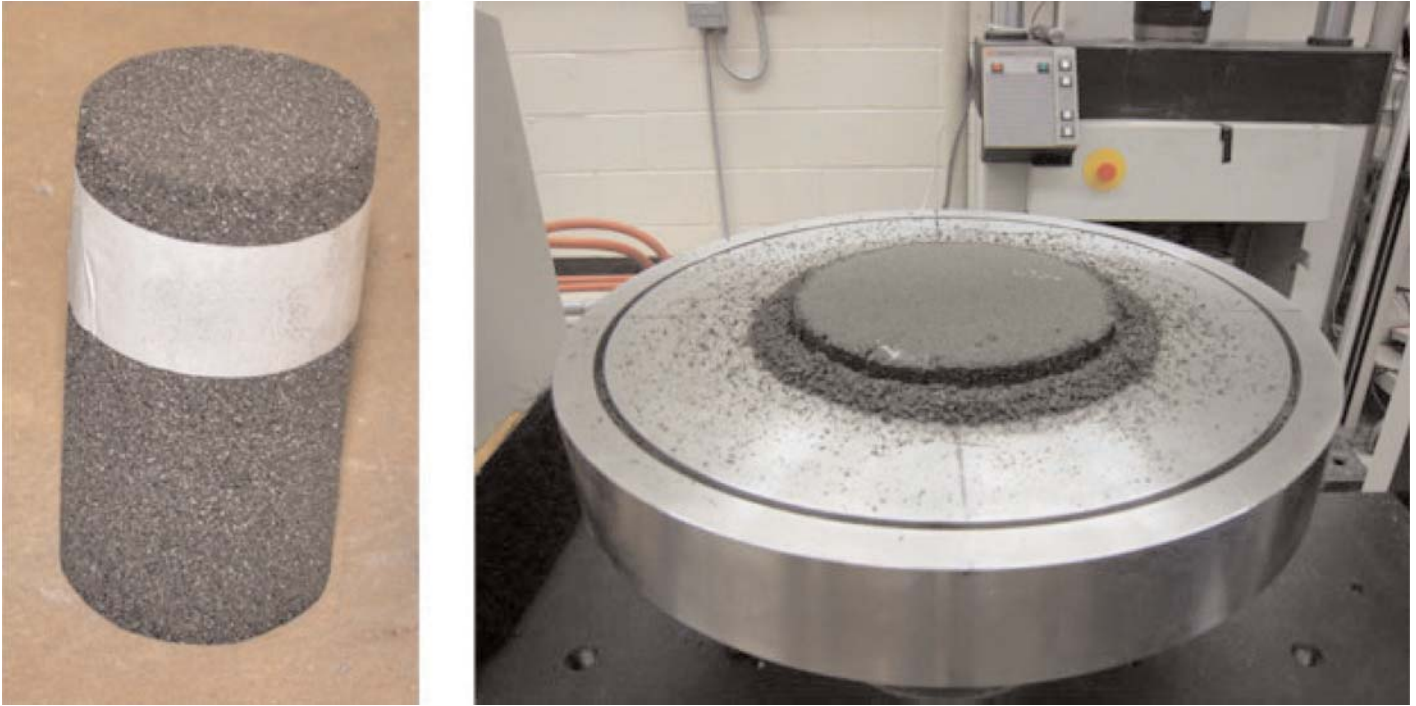
Figure 9-4. Low-rate uncapped platen test of glass foam pre-test (left) and post-test (right).
