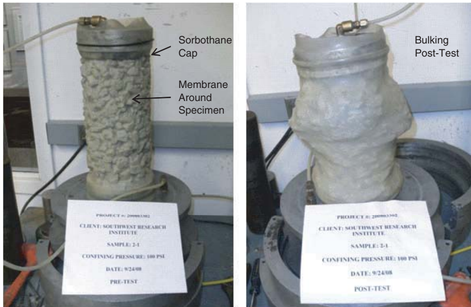
Figure 11-9. Hydrostatic triaxial compression test of aggregate foam pre-test (left) and post-test (right), 100 psi confining pressure.
