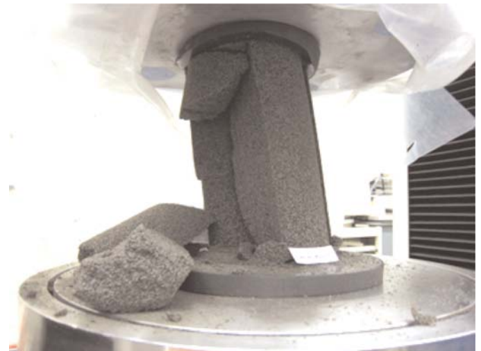
Figure 9-5. Mid-test splitting of low-rate capped platen test cylinder of glass foam.
