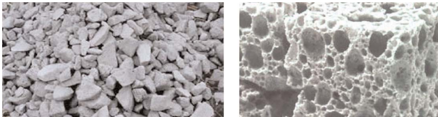
Figure 11-1. Aggregate foam material: pile of aggregate (left) and close-up of microstructure (right) (43).
