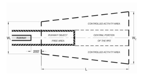
Figure 4. Runway protection zone diagram.
