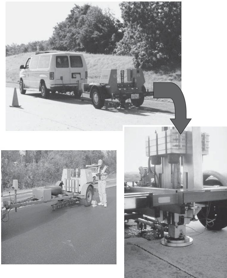
Figure 5. Trailer mounted FWD.
