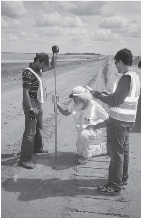
Figure 9. DCP test and large aggregate particles encountered at some of the projects, resulting in refusal of the test.
