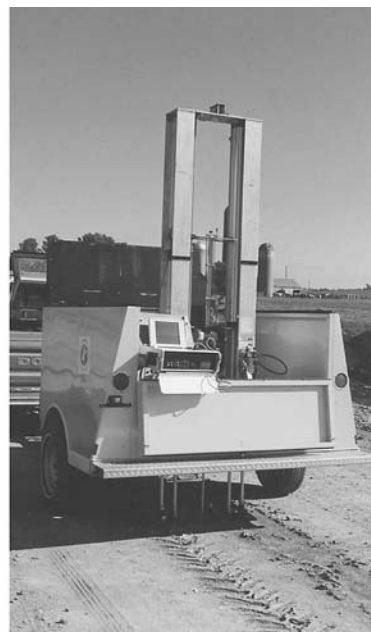
Figure 10. Automated DCP attached to a trailer (courtesy of Minnesota Road Research Section, Office of Materials, Minnesota DOT).
