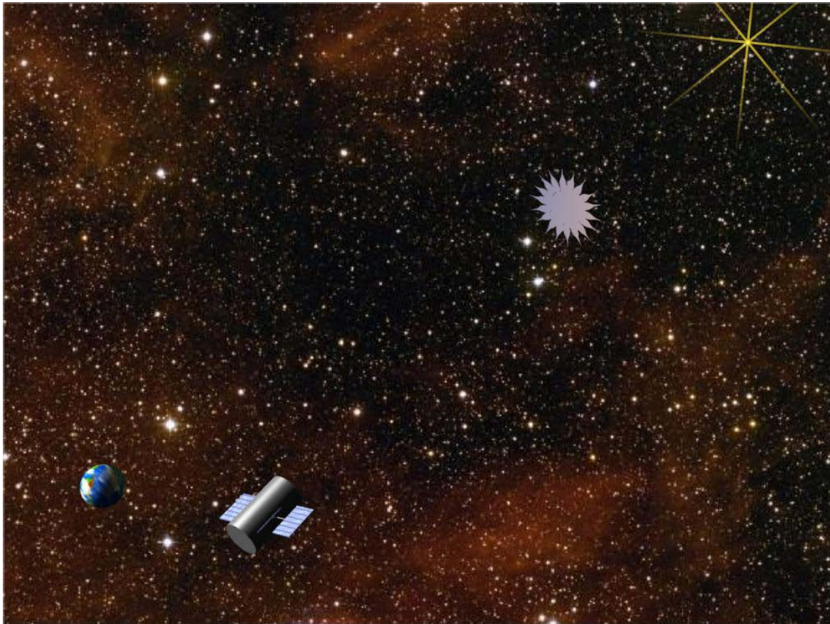
FIGURE F-6 An artist's rendering of the New Worlds Observer concept for imaging a distant planetary system. Light from the central star is blocked by a large external occulter disk that is shaped to control diffraction of the starlight around the occulter. A telescope placed in the right location can image the surrounding planetary system without glare from the central star. SOURCE: Webster Cash, The New Worlds Imager, Final Report to the NASA Institute for Advanced Concepts for Phase I Study , NIAC Phase I study report, 2005. Courtesy of Webster Cash, University of Colorado.
