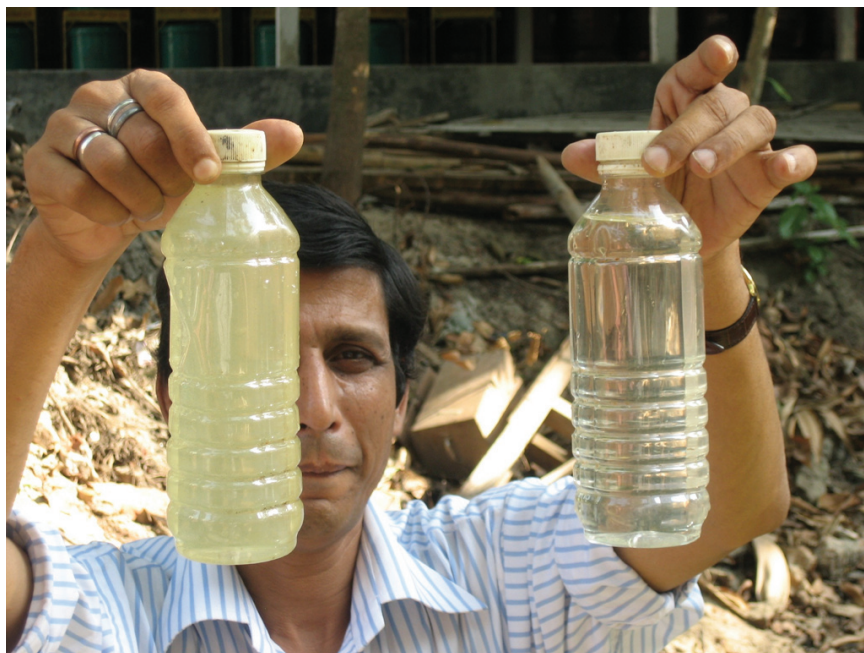
FIGURE 3-5 Water that appears to be of high quality (right) upon initial draw from the tube well can contain high concentrations of iron and arsenic—the water starts to become turbid (left) through a process of oxidization and self-attenuation.
