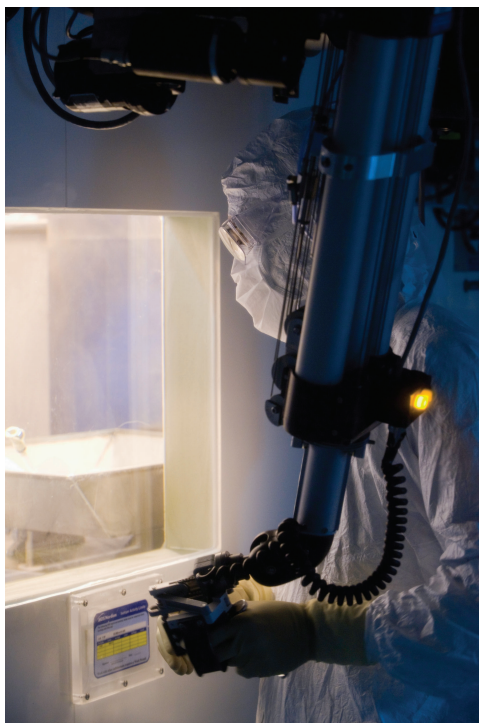
FIGURE 2.6 (a) Hot cells in use at CNEA for processing of LEU targets to recover Mo-99. (b) Worker operating hot cell manipulators at MDS Nordion. SOURCE: Courtesy of CNEA and MDS Nordion, respectively.
