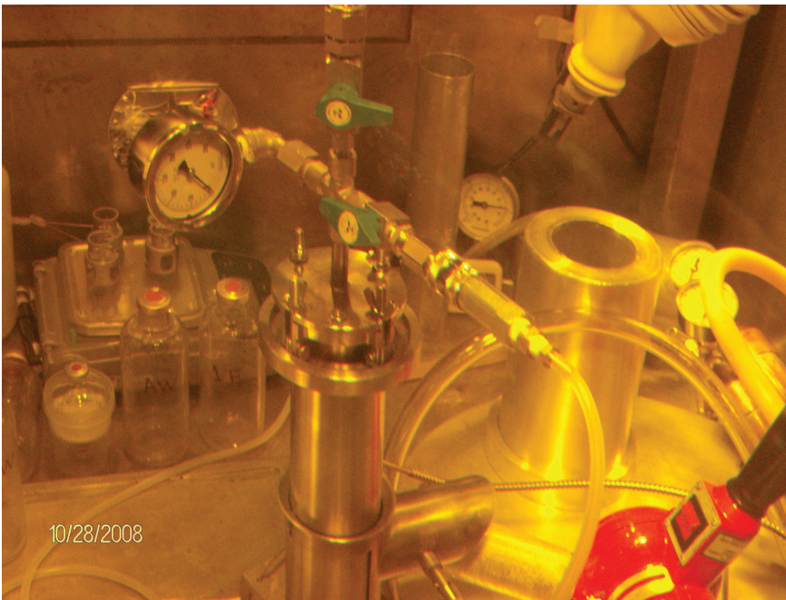
FIGURE 2.7 (a) View into a hot cell at CNEA showing the target processing equipment. (b) View into a hot cell at MURR showing the new dissolver for the LEU metal foil targets. SOURCE: Courtesy of CNEA and the University of Missouri, respectively.
