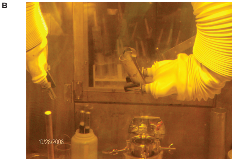
FIGURE 7.1 (a) LEU metal foil targets developed by Argonne National Laboratory. (b) Views into the hot cell at the Missouri University Research Reactor (MURR) showing the irradiated LEU foil target being removed from the target cladding in preparation for dissolution. SOURCES: Courtesy of George Vandergrift, Argonne National Laboratory, and the University of Missouri, respectively.
