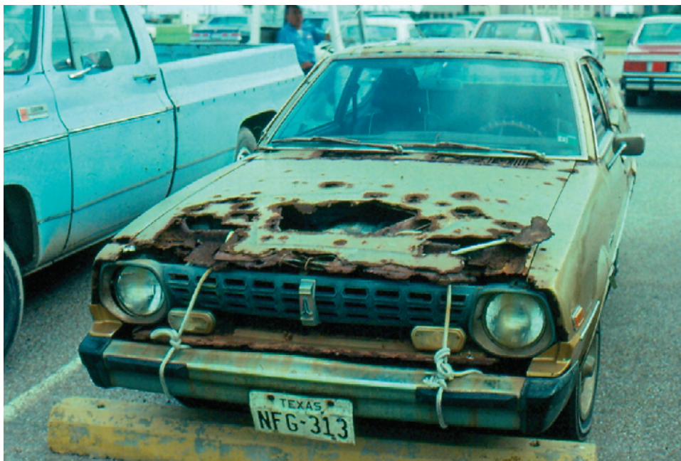
FIGURE 1-3 Corrosion on an automobile operating in a warm, moist chloride environment. While anticorrosion technology for cars has improved tremendously in recent years, this picture shows the extreme corrosion that is still possible. Courtesy of Richard Griffin.
