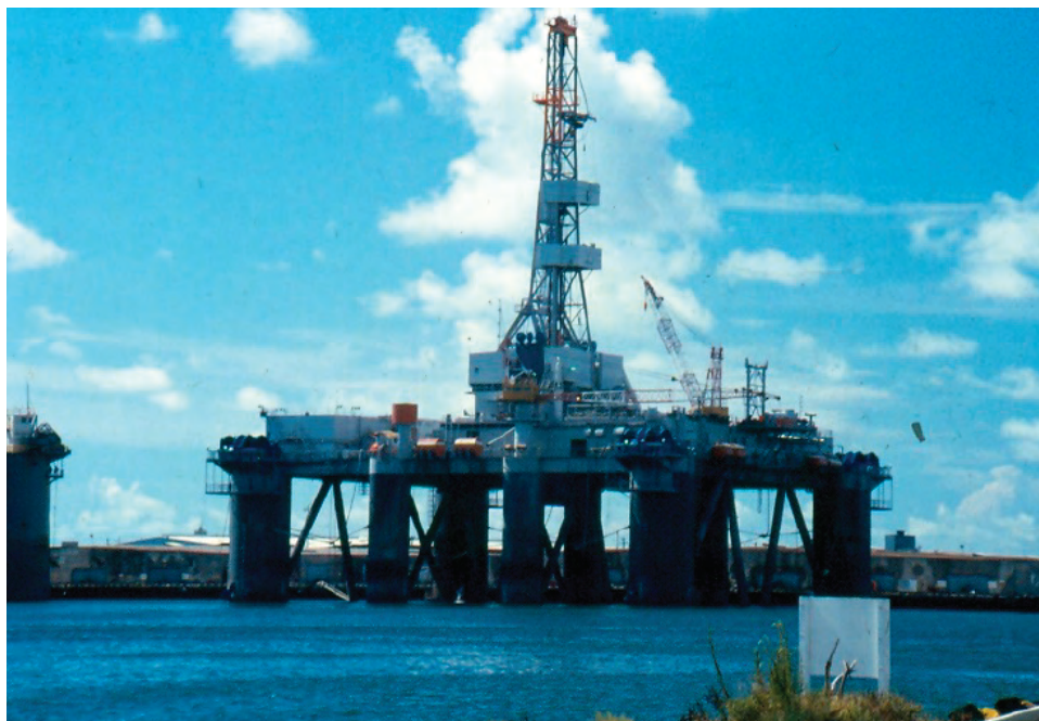
FIGURE 1-1 Offshore semisubmersible drilling rig used in the production of oil and gas. Courtesy of Richard Griffin.
