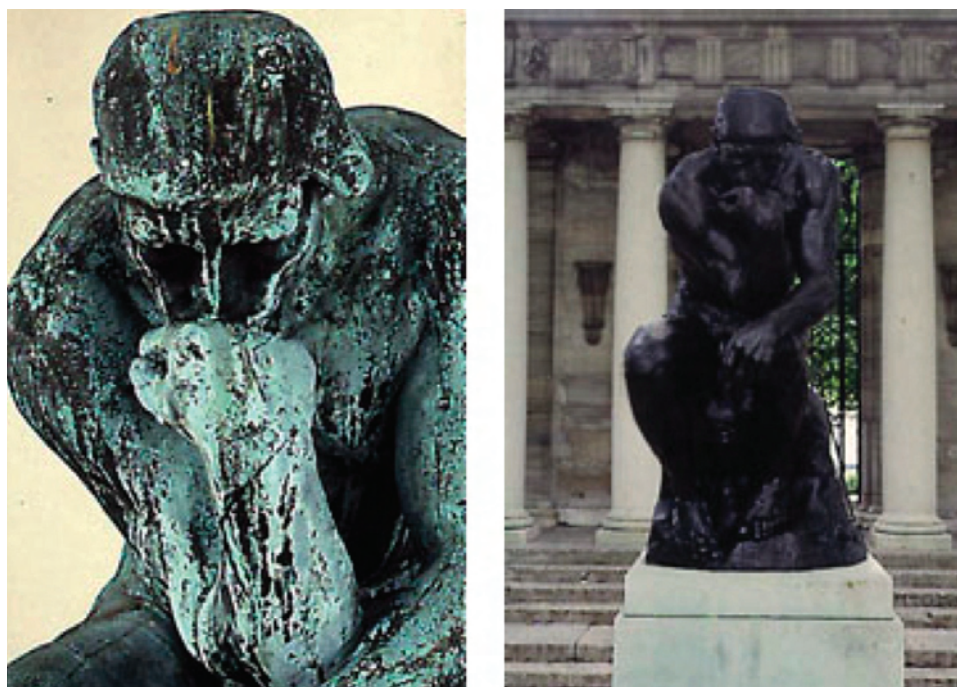
FIGURE 1-7 Corrosion on Rodin's "Thinker." Courtesy of Philadelphia Museum of Art: Bequest of Jules E. Mastbaum, 1929.
