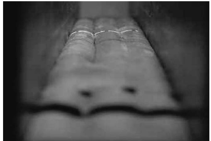
Figure 2.2. Initial debonding of bearing.
