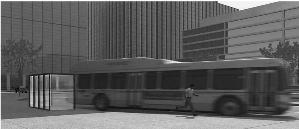
Figure 1-4. Illustration of Collision Type 4—collision with pedestrian running alongside bus when pulling away from a bus stop.
