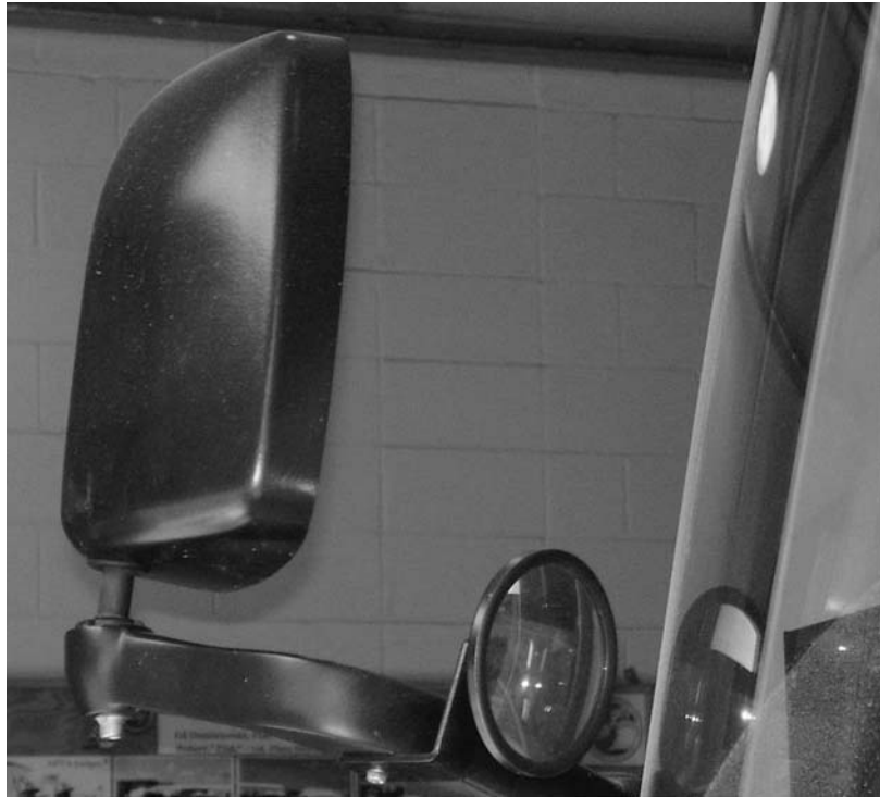
Figure 2-11. Convex mirror on right side with downward slant.
