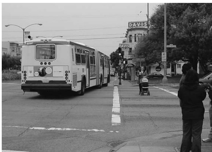
Figure 2-18. Bus stop located on far-side of intersection.
