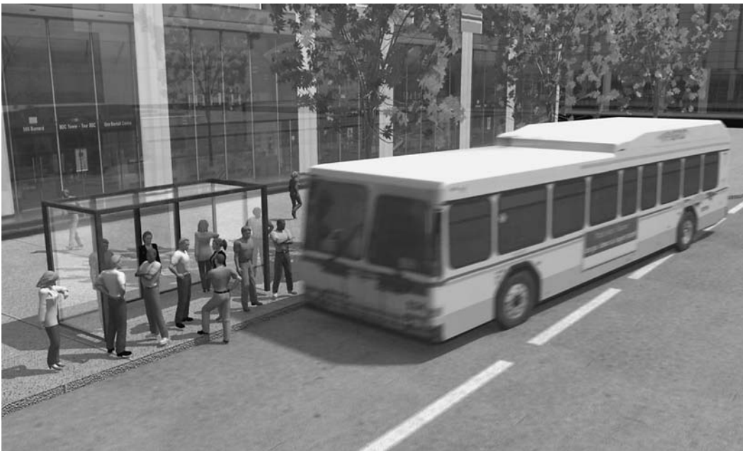
Figure 1-3. Illustration of Collision Type 3—collision between pedestrian and bus pulling into bus stop.
