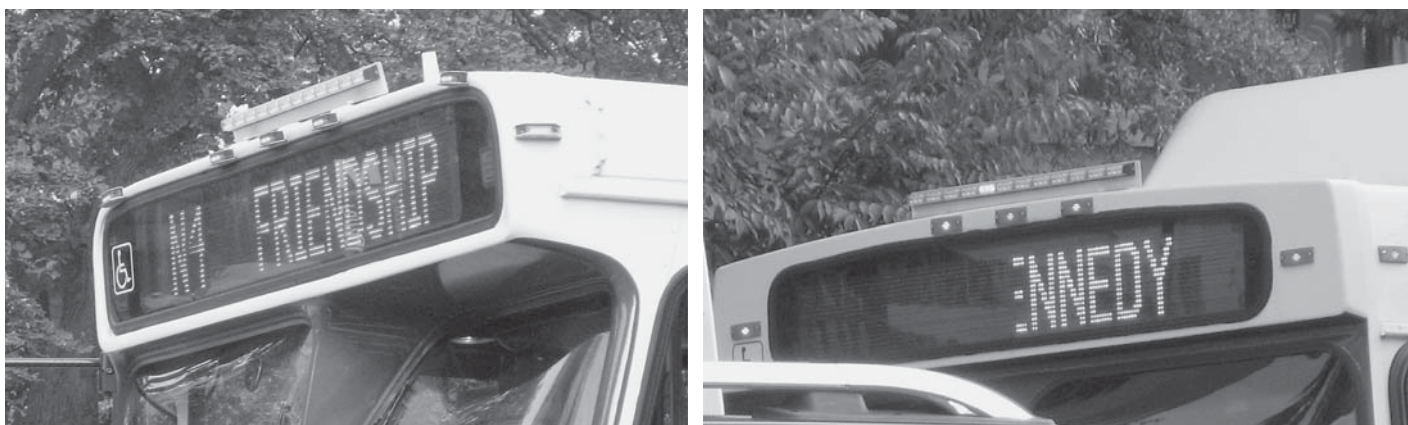
Figure 2-15. LED light strip on front-top of bus.
