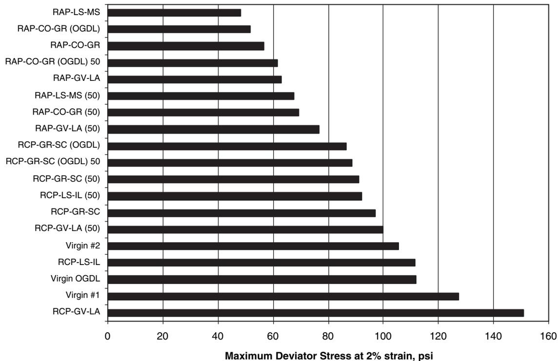
Figure 5.11. Shear strength at 2-percent strain in repeated load triaxial test.
