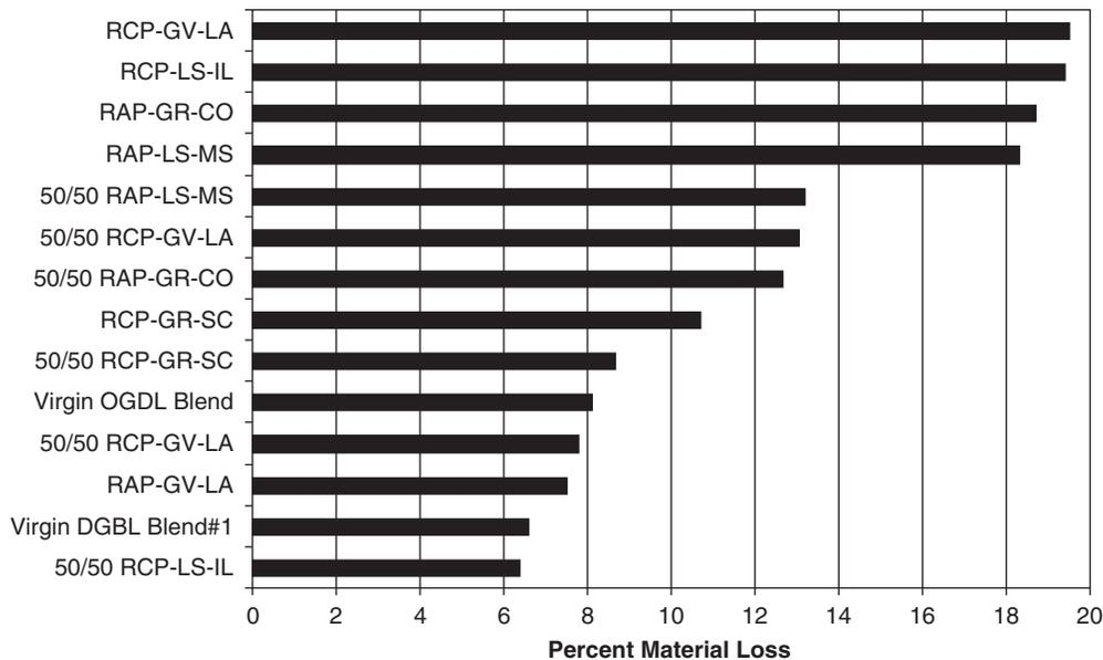
**Figure 5.1. Results of Micro-Deval tests.**
