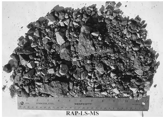
**Figure 3.9. Photograph of RAP-LS-MS material used for laboratory testing.**
