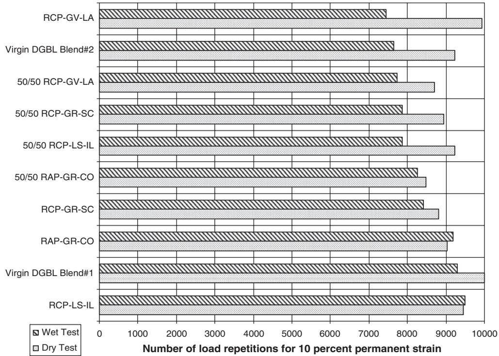
**Figure 4.14. Failure load repetitions for wet and dry tests.**
