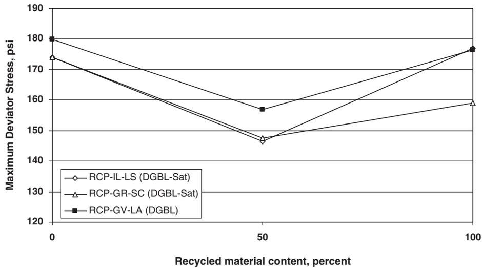
Figure 5.9. Repeated load triaxial test results for RCP-DGBL samples.
