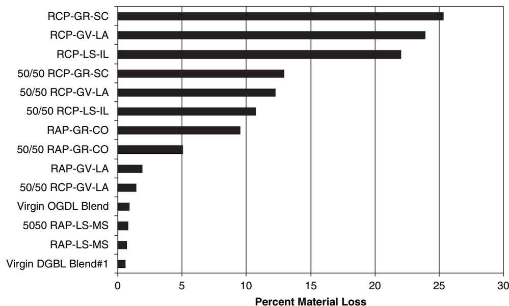
Figure 5.2. Canadian Freeze-Thaw test results.
