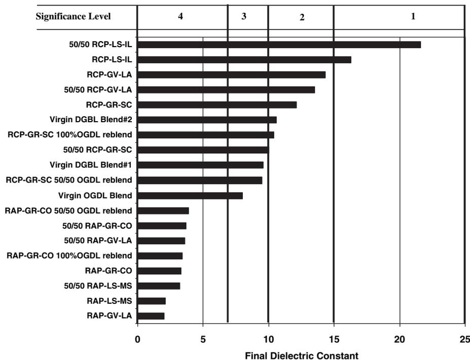
Figure 5.19. Performance potential based on frost susceptibility.
