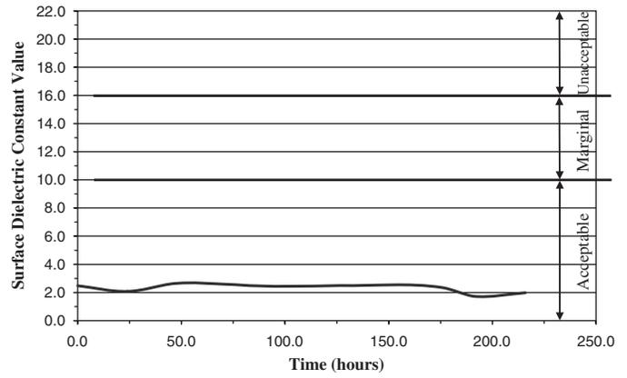
Figure 4.19. Dielectric constant value curve with time for RAP-GV-LA.
