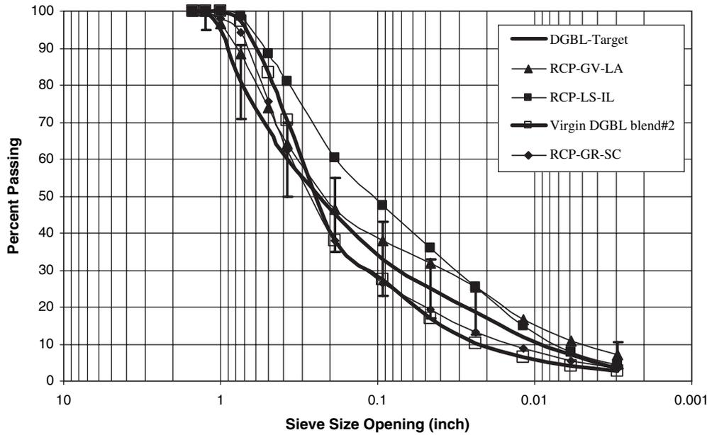
Figure 4.1. Gradation results of RCP as-received DGBL samples.
