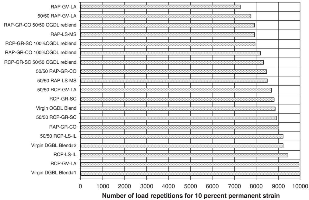
**Figure 4.13. Number of load repetitions at 10-percent permanent strain (dry tests).**
