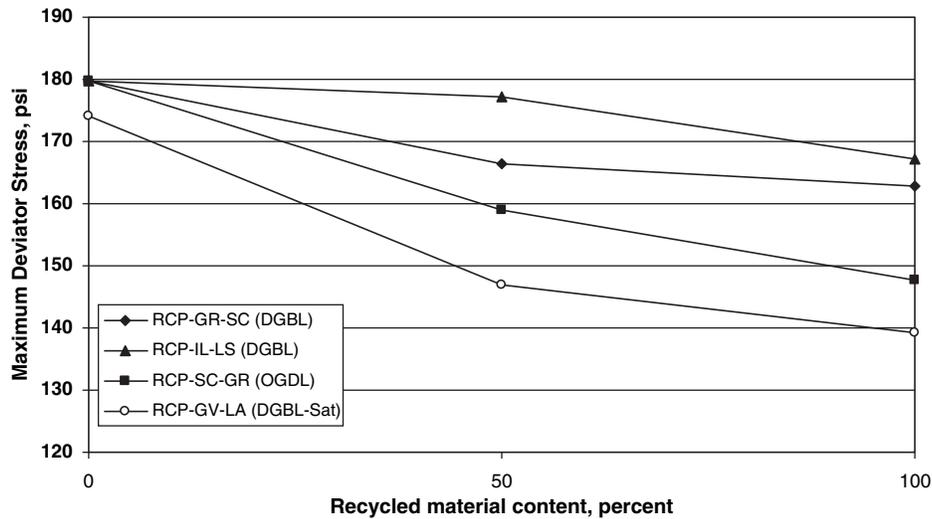
Figure 5.8. Repeated load triaxial test results for RCP samples.
