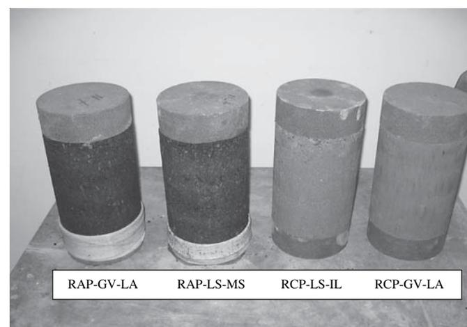
**Figure 4.16. Molded RAP and RCP samples.**
