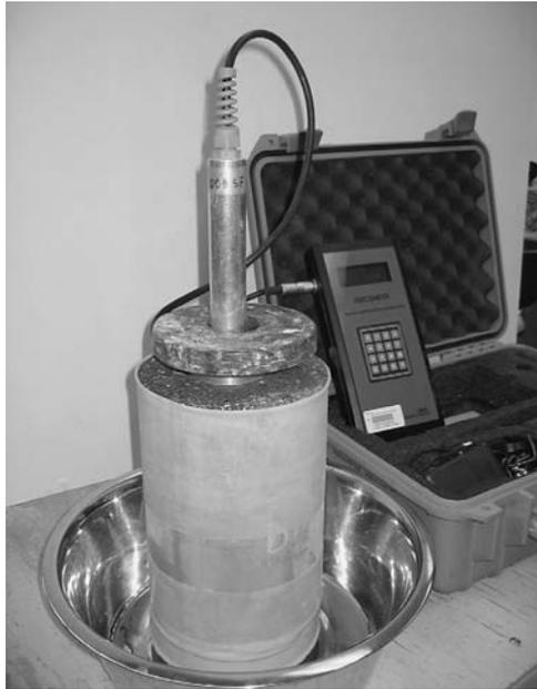
Figure 4.17. Apparatus used to make surface dielectric measurements.
