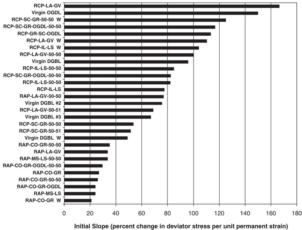
Figure 5.15. Order of materials based on initial load-strain slope.
