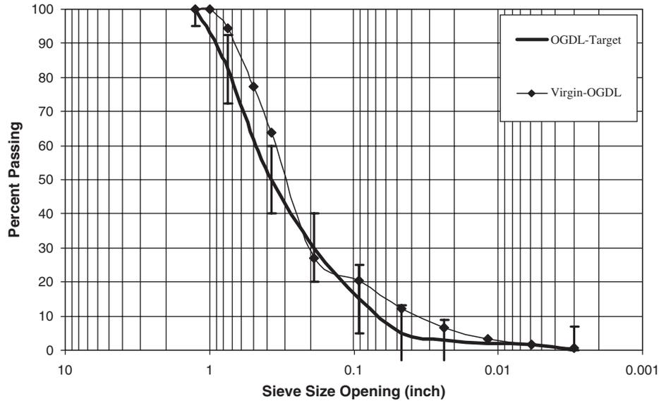
Figure 4.5. Gradation results of virgin aggregate OGDL-blended sample.
