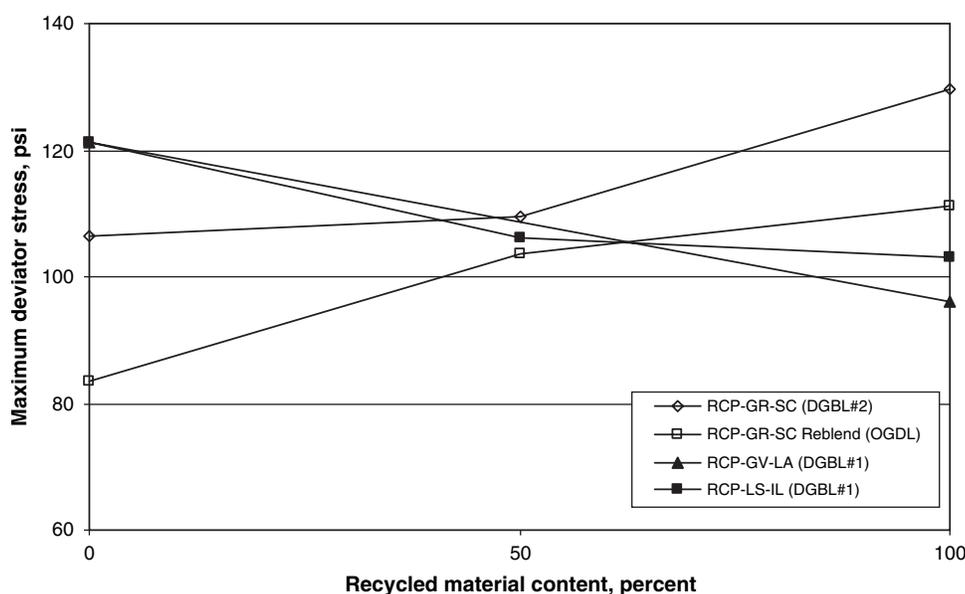
Figure 5.5. Maximum deviator stress versus recycled material content (RCP).
