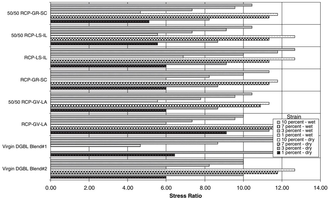
Figure 4.12. Stress ratios for dry and wet triaxial tests on RCP samples.
