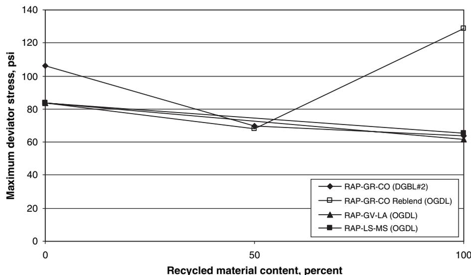
Figure 5.4. Maximum deviator stress versus recycled material content (RAP).
