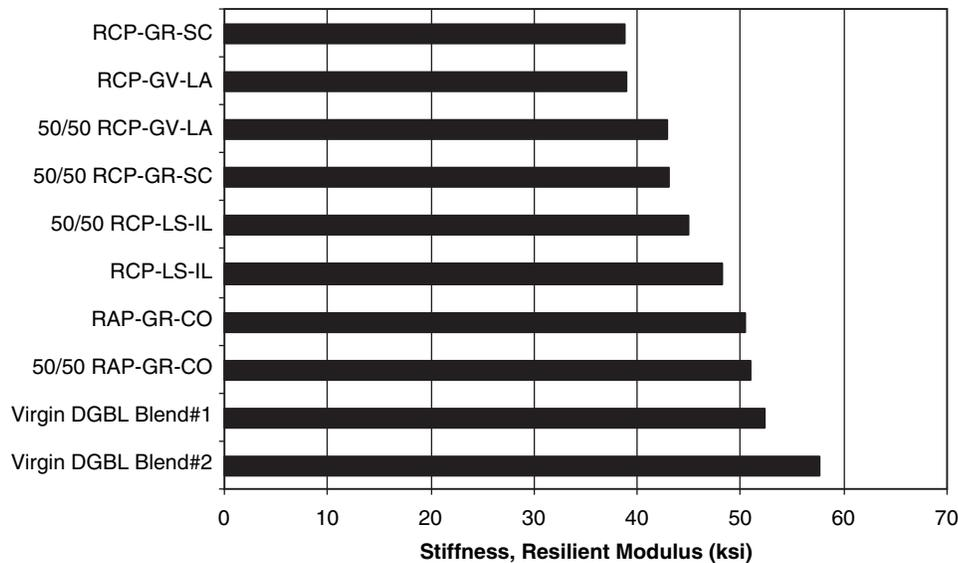
**Figure 5.17. Estimated stiffness at 100 psi bulk stress (sat. repeated load triaxial test).**
