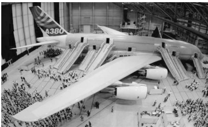
Figure 10. Airbus A380 certification test. (Photo source: FAA, www.Airporttech.tc.faa.gov/safety/patterson1.asp )
