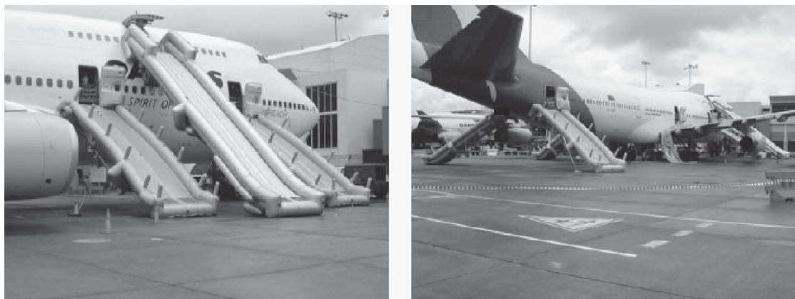
Figure 10: Slide emergency evacuation of a Boeing 747-438 (Sydney, Australia, July 2, 2003) (Photo source: Australian Transport Safety Bureau)
