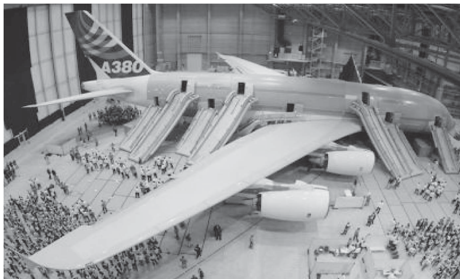
Figure 11: Airbus A380 Certification Test (Source: http://www.airporttech.tc.faa.gov/safety/patterson1.asp )
