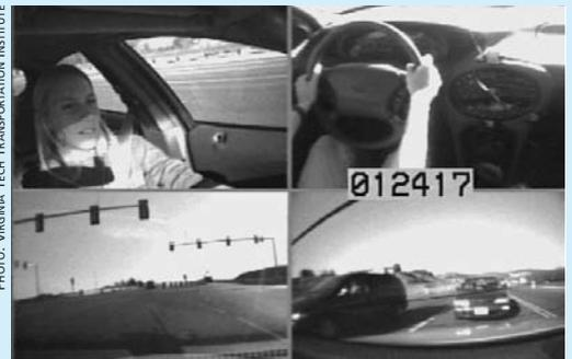
Simultaneous video images from the 100-Car Study recorded (clockwise from top left) the driver's face, the view over the driver's shoulder, the rear view, and the left-side view.
