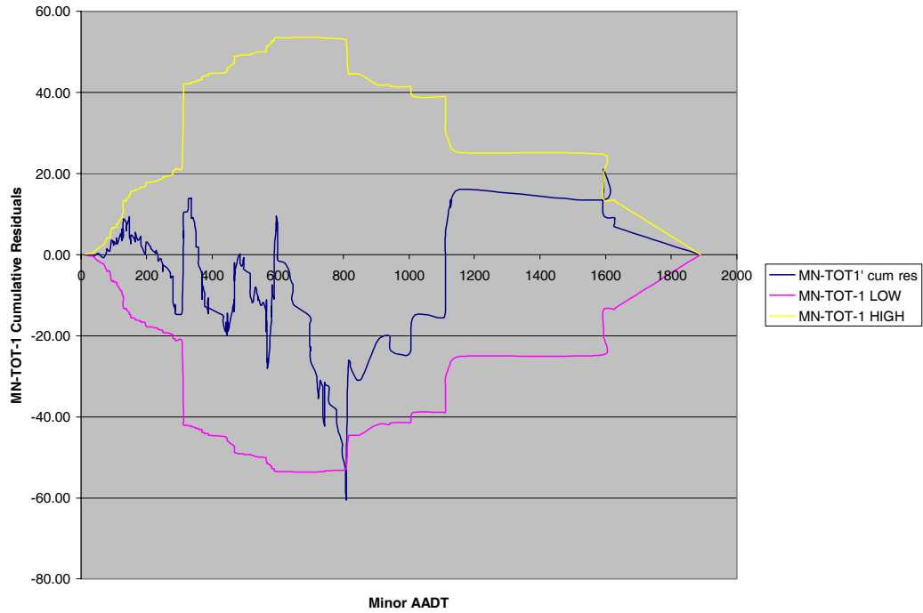
Figure D7 CURE Plot for the Minnesota Model and Total Crashes (Minor AADT)
