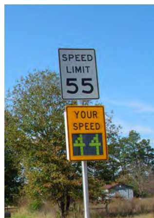
Exhibit 2-5 Dynamic curve-warning sign (Photo: TXDOT)
