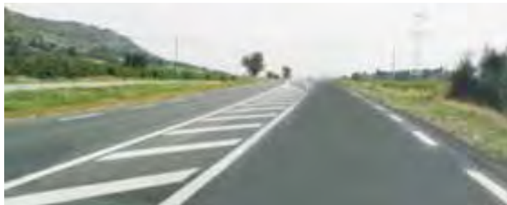
Exhibit 2-14 Examples of wider longitudinal pavement markings in France
