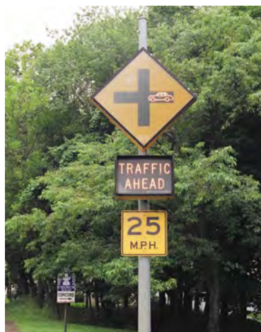
Exhibit 2-6 Dynamic warning sign used as a Collision Avoidance System (Photo: PennDOT)
