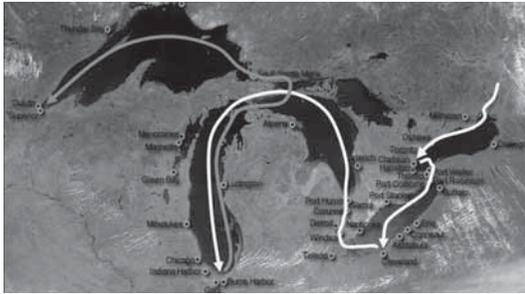
Typical transit of a transoceanic vessel on the Great Lakes: the inbound leg includes stops in Hamilton, Ontario; Cleveland, Ohio; and Burns Harbor, Indiana, where cargo is discharged and Great Lakes' ballast water is loaded, mixing with residual water in the ballast tanks. The inbound leg terminates in Lake Superior, where mixed ballast water is discharged—along with surviving species—when outbound cargo is loaded in the Twin Ports of Duluth, Minnesota, and Superior, Wisconsin.
