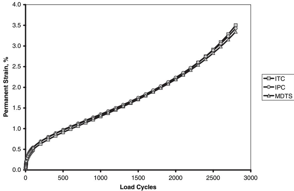
**Figure 20.** Average permanent strain response for unconfined repeated load tests.
