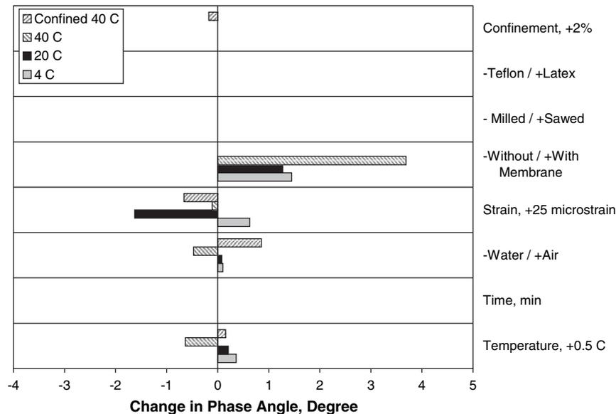
**Figure 7. Effect of statistically significant ruggedness factors on the phase angle.**
