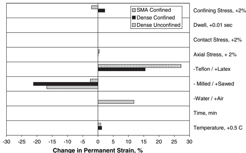
**Figure 13. Effect of statistically significant ruggedness factors on the permanent strain after 500 load cycles.**
