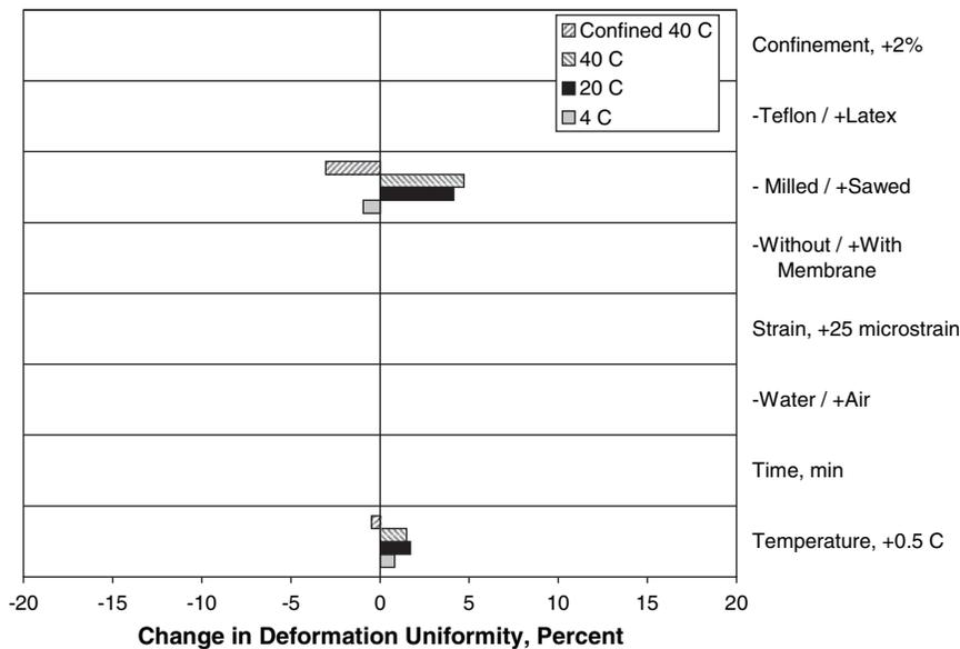
**Figure 10. Effect of statistically significant ruggedness factors on the deformation uniformity.**
