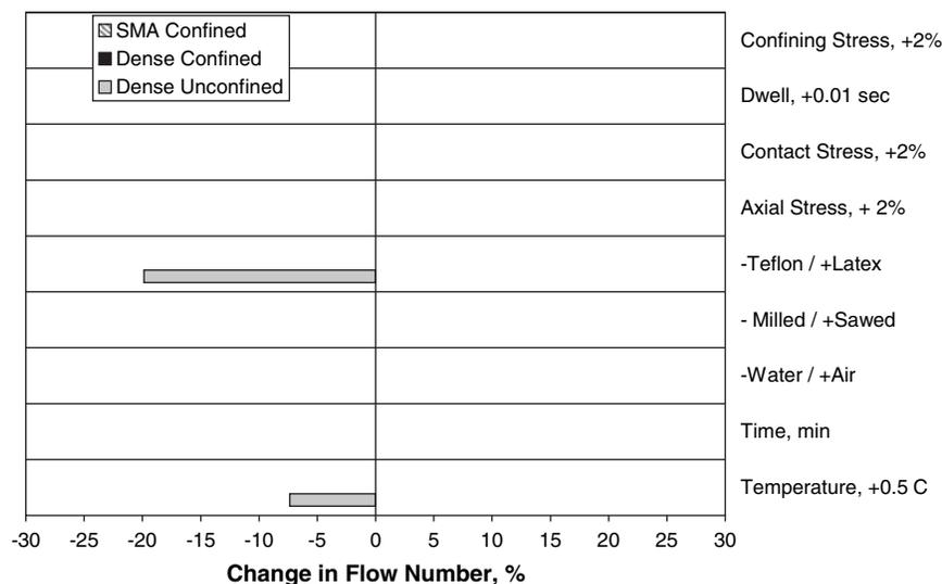
**Figure 12. Effect of statistically significant ruggedness factors on the flow number.**
