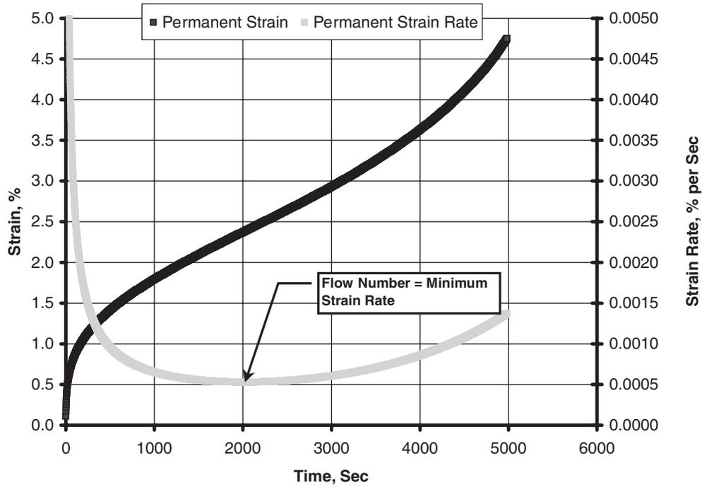
**Figure 1. Schematic of Flow Time Test Data.**
