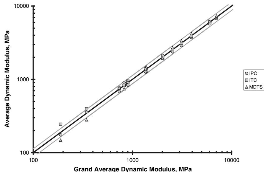
**Figure 18.** Comparison of mean dynamic moduli from the three machines.
