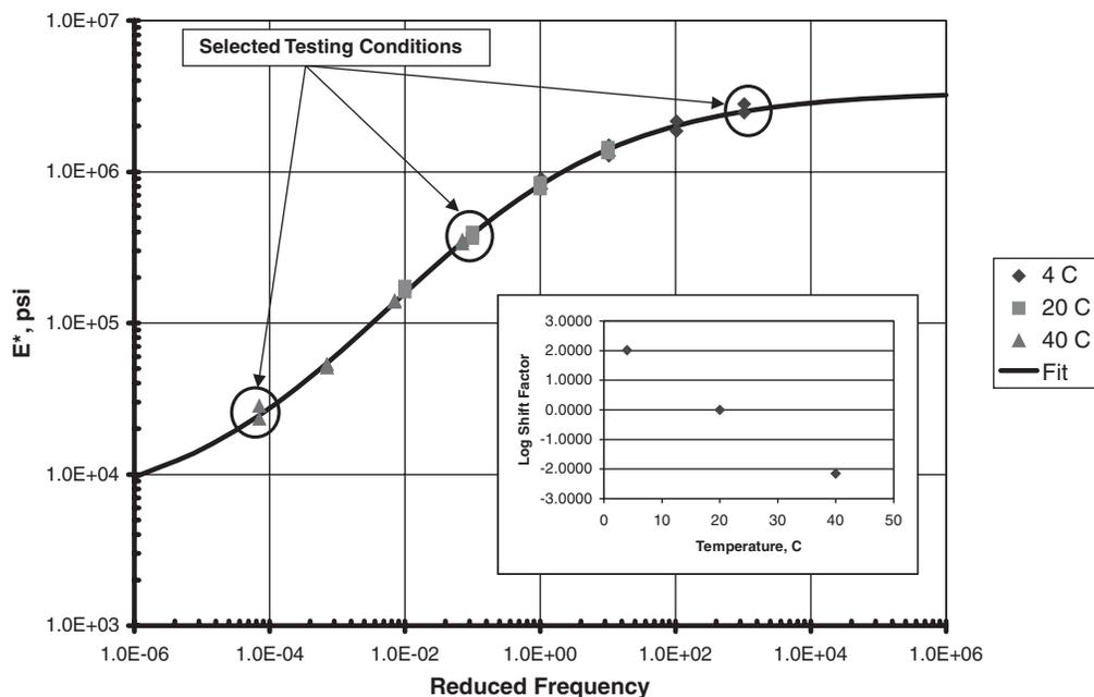
Figure 1. Typical dynamic modulus master curve.
