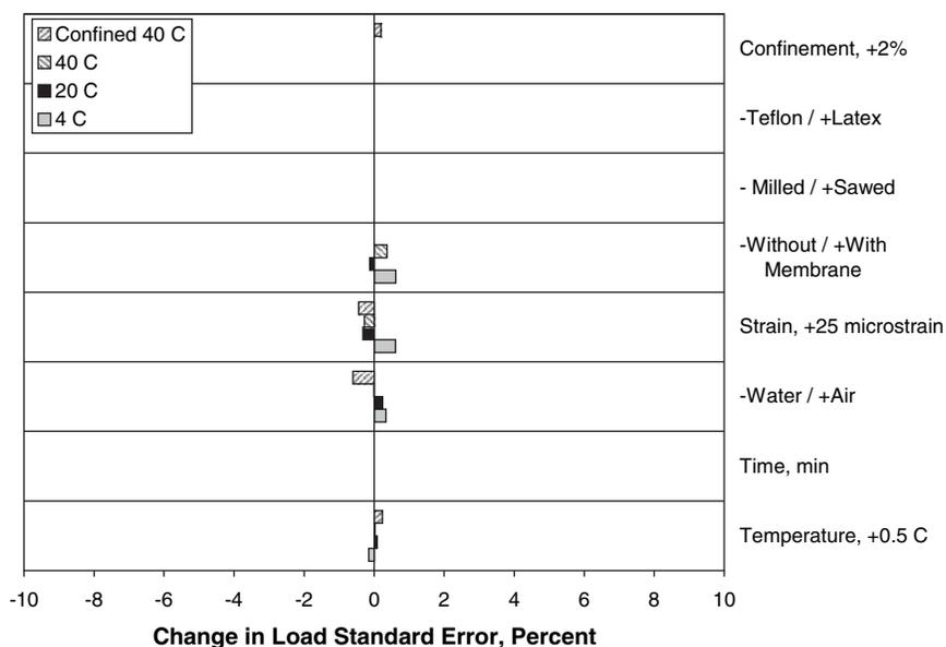
**Figure 8. Effect of statistically significant ruggedness factors on the load standard error.**
