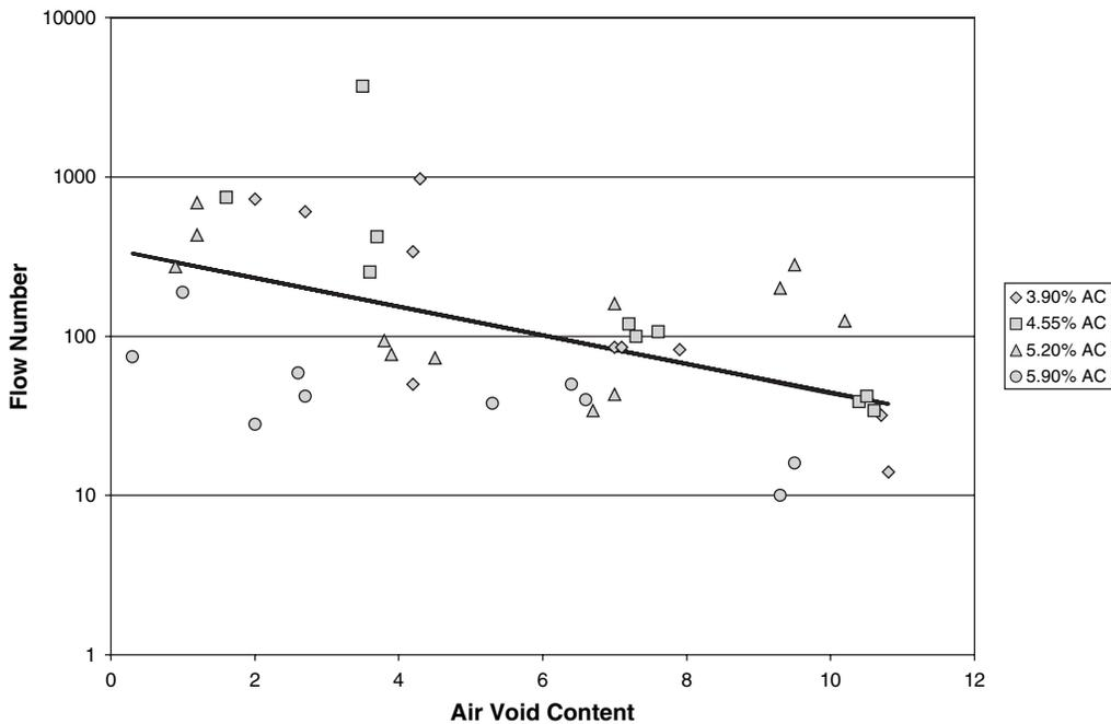
**Figure 4. Effect of air voids on confined flow number [data from Project 9-19 (10)].**
