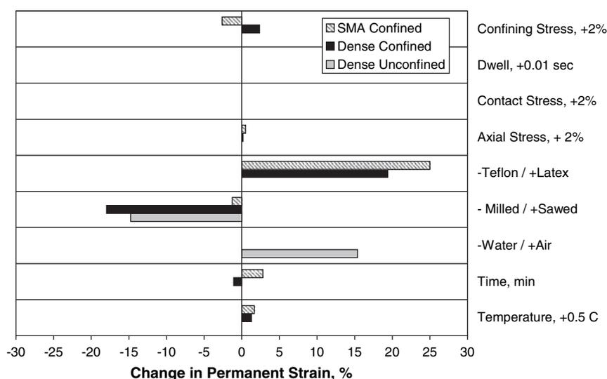
**Figure 14. Effect of statistically significant ruggedness factors on the permanent strain after 1,000 load cycles.**
