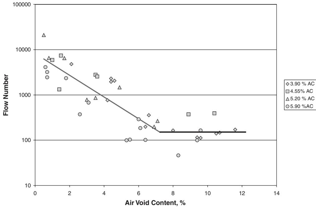
**Figure 3. Effect of air voids on unconfined flow number [data from Project 9-19 (10)].**
