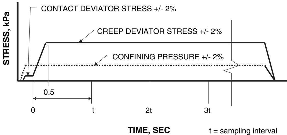
**Figure 5. Schematic of Loading and Data Acquisition.**
