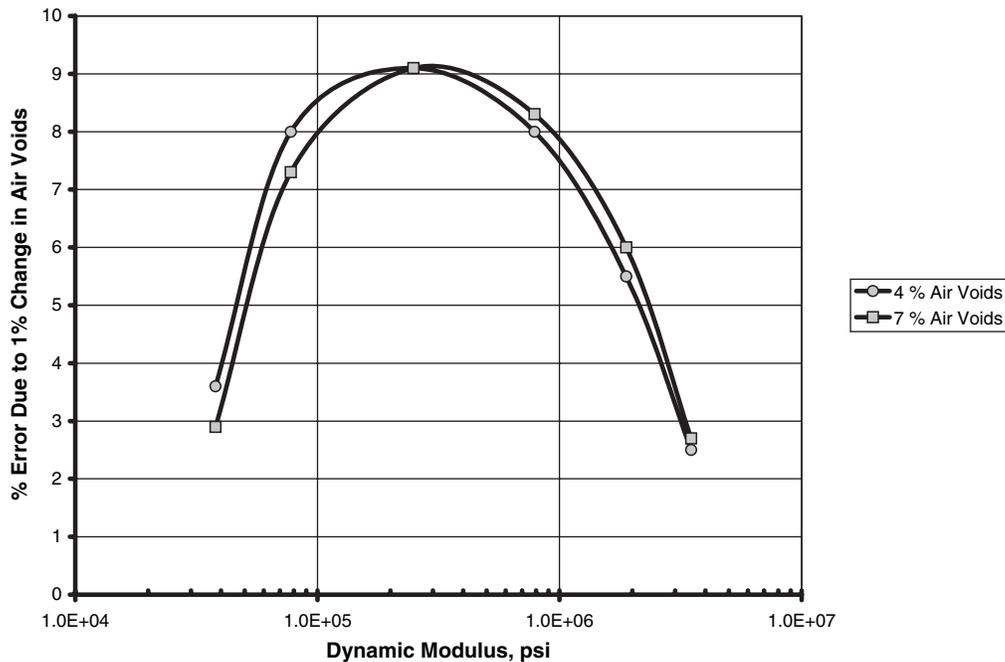
Figure 2. Estimated testing error for current air void tolerance.
