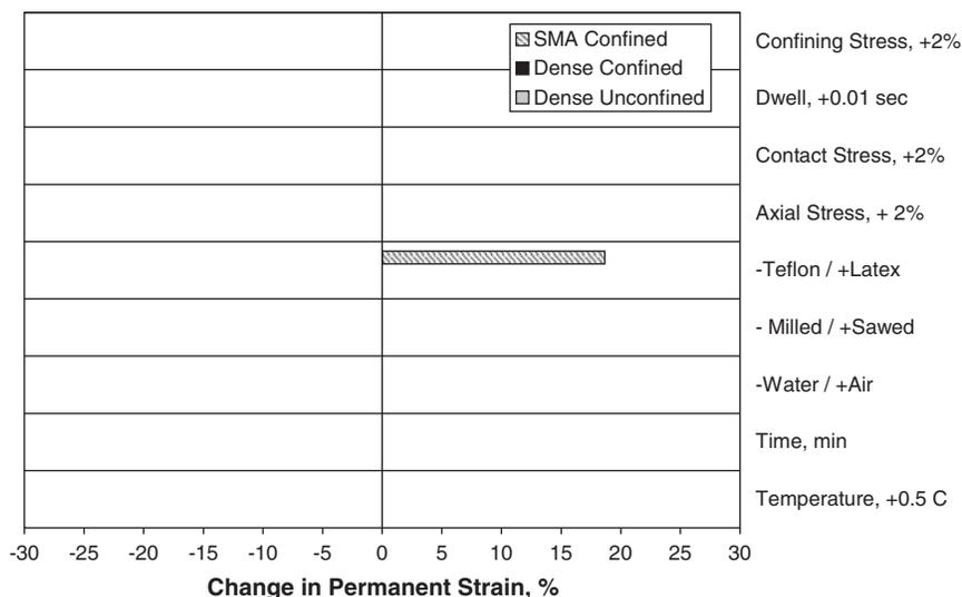
**Figure 16. Effect of statistically significant ruggedness factors on the permanent strain after 5,000 load cycles.**
