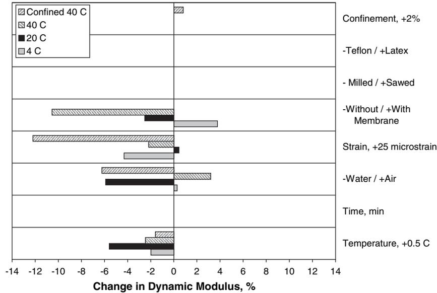
**Figure 6. Effect of statistically significant ruggedness factors on the dynamic modulus.**
