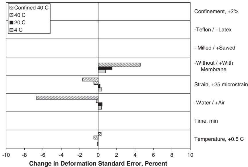
**Figure 9. Effect of statistically significant ruggedness factors on the deformation standard error.**
