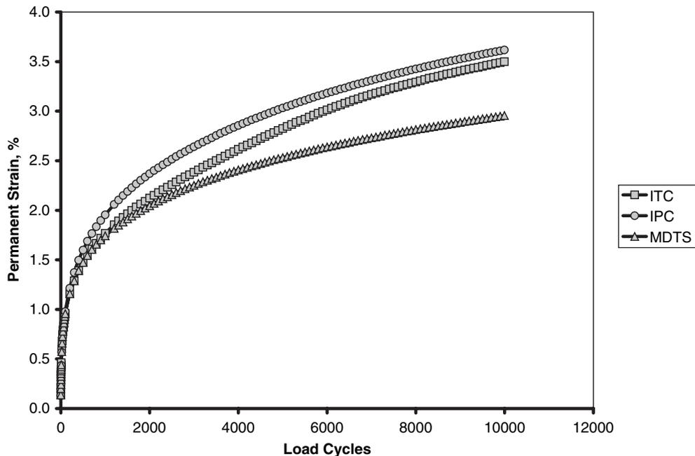
**Figure 21.** Average permanent strain response for confined repeated load tests.
