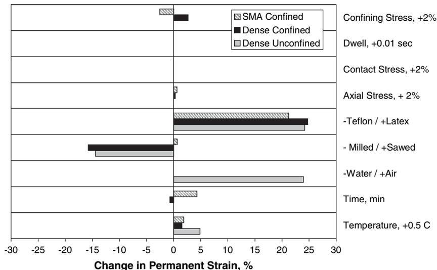
**Figure 15. Effect of statistically significant ruggedness factors on the permanent strain after 2,000 load cycles.**
