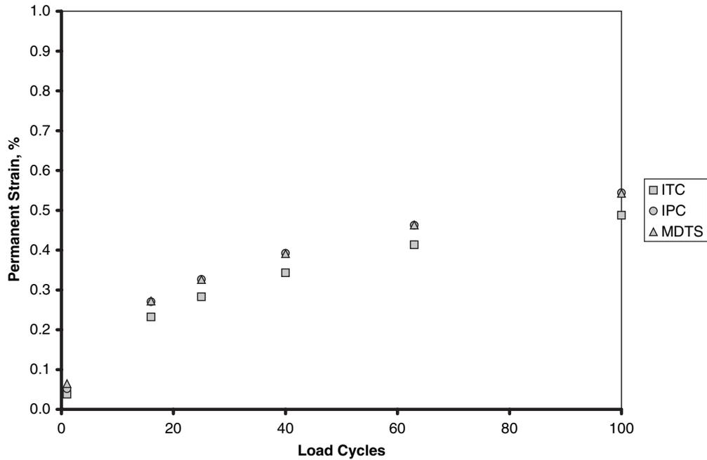
**Figure 22. Comparison of permanent deformation response for the early portion of the unconfined repeated load tests.**
