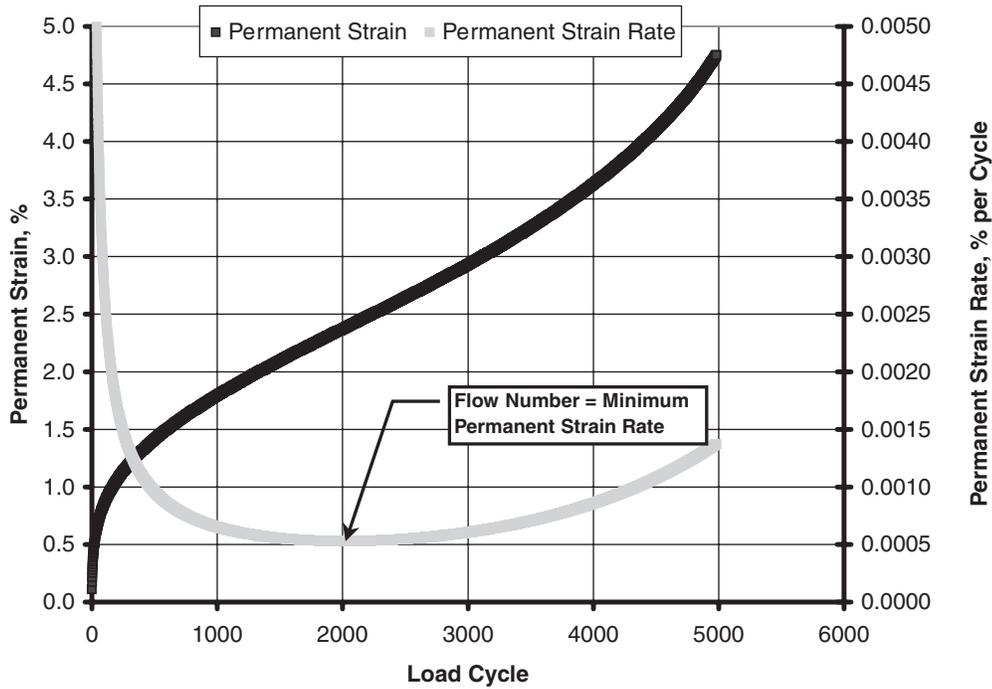
**Figure 2. Schematic of Flow Number Test Data.**
