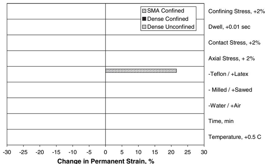
**Figure 17. Effect of statistically significant ruggedness factors on the permanent strain after 8,000 load cycles.**
