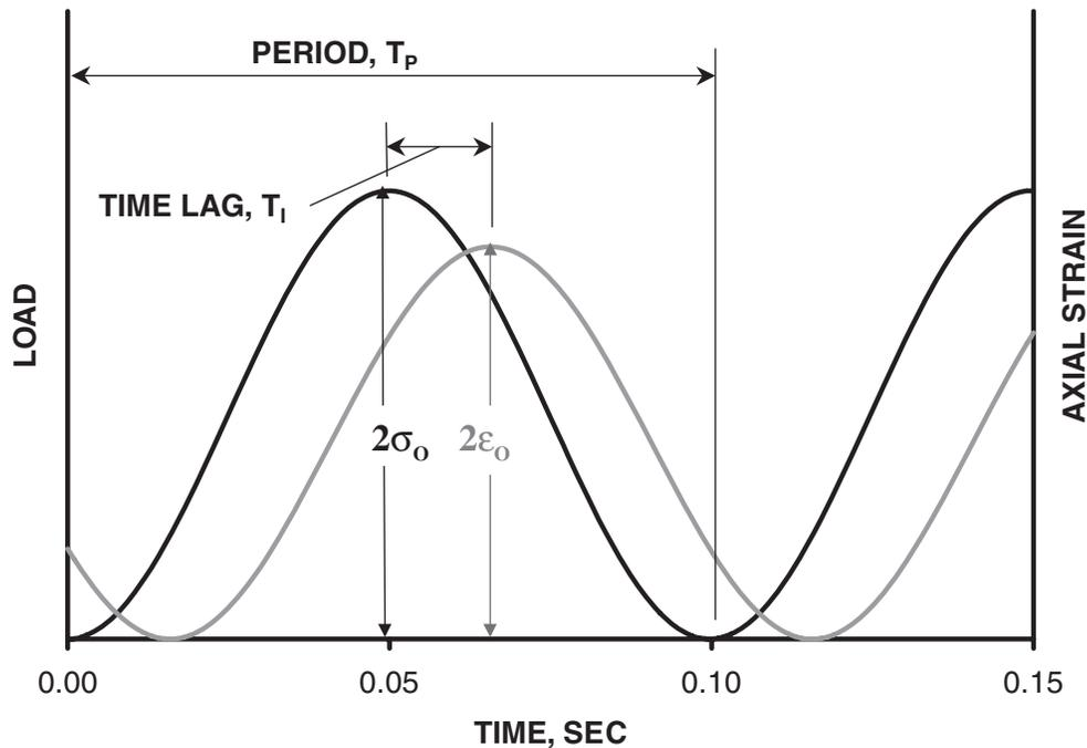
Figure 3. Schematic of Dynamic Modulus Test Data.
