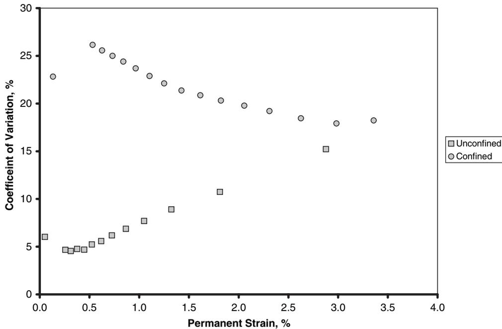
**Figure 23. Coefficient of variation for unconfined and confined repeated load tests.**
