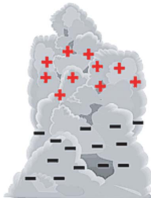
Figure 2. An idealized small thunderstorm with charges separated into a simple electrical dipole (5).
