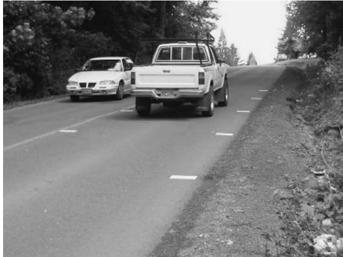
Exhibit 4-4. Peripheral transverse pavement markings.
