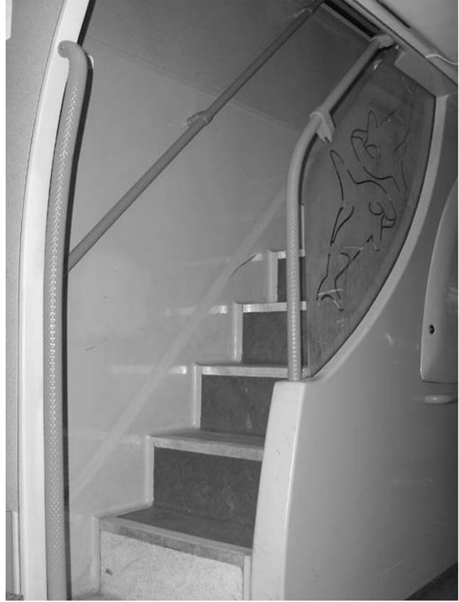
FIGURE 19 Internal double-deck staircase as seen from below. (Source: BC Transit.)
