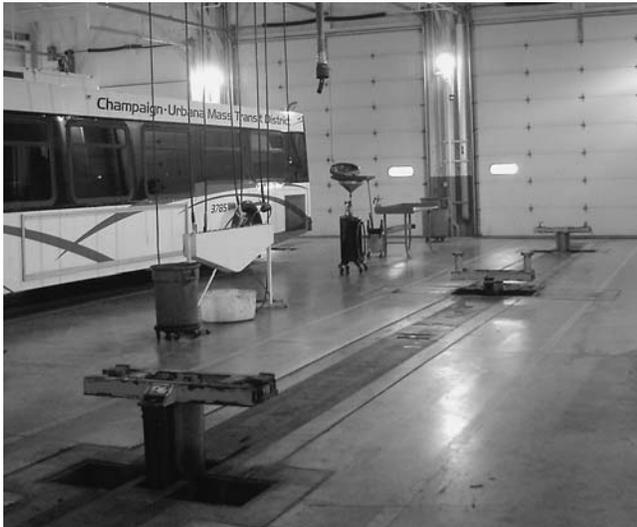
FIGURE 26 MTD hoist equipment for articulated buses.
