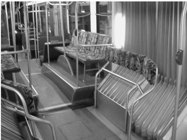
FIGURE 23 Hip rests used in MTD articulated buses.
