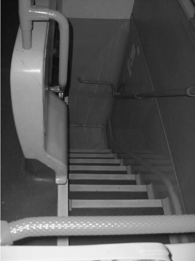
FIGURE 18 Internal double-deck staircase as seen from above. (Source: BC Transit.)
