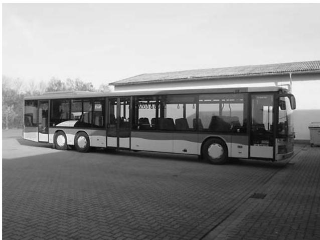
FIGURE 27 A 15-m low-floor EVB Linenbus.
