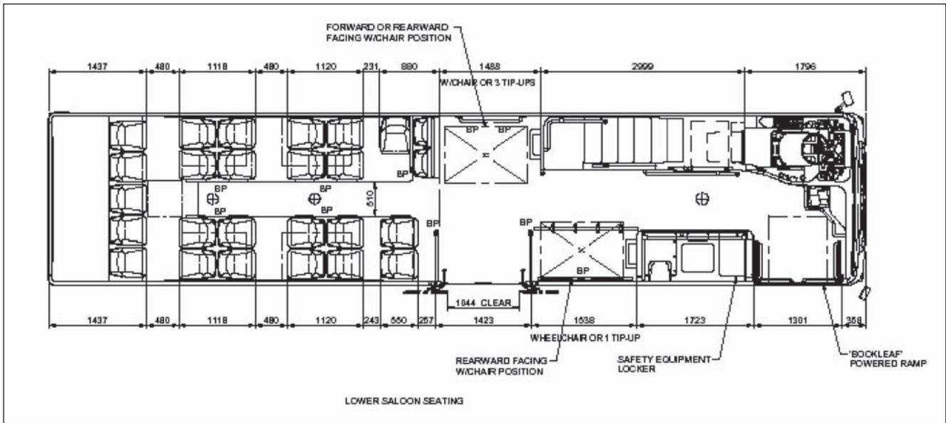
FIGURE 14 Floor plan of lower deck of Victoria's double-deck bus. (Source: Alexander Dennis.)
