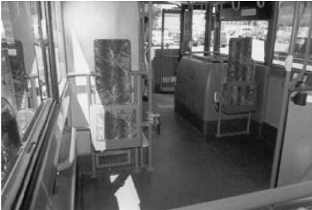
FIGURE 20 Wheelchair positions on BC Transit low-floor double-deck buses: Combi system roadside and rear-facing system curbside. Note: Both wheelchair positions have backrests with flip-down seats.
