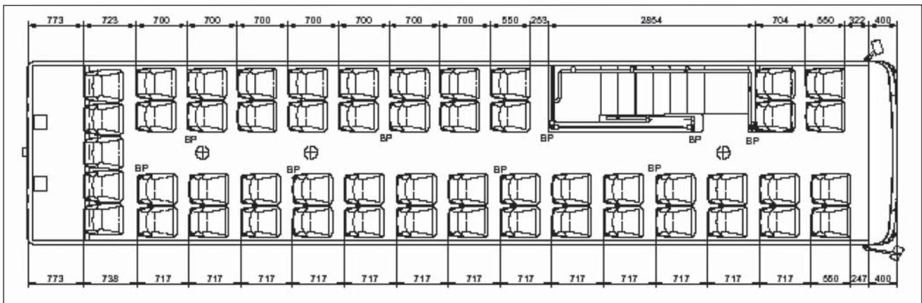
FIGURE 15 Floor plan of upper deck of Victoria's double-deck bus. (Source: Alexander Dennis.)
