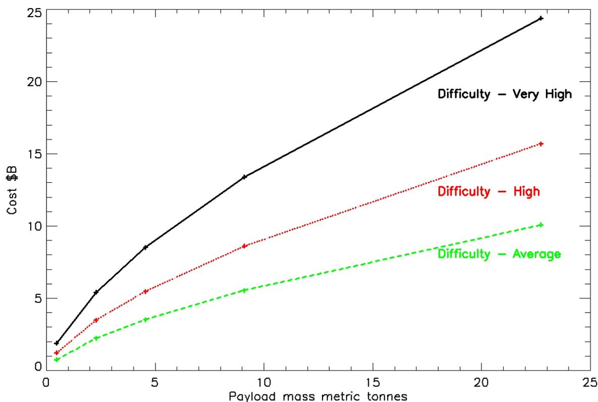
FIGURE 1.1 Estimated costs as a function of payload mass for three classes of difficulty for solar system exploration missions utilizing NASA's Advanced Mission Cost Model. NOTE: For comparison, the Cassini-Huygens payload mass was approximately 4.6 metric tons. Note that the Ares V capabilities would actually span a number of payload masses in this figure. For example, Ares V could launch 10 metric tons to Uranus or Neptune, and significantly more to Jupiter and Mars.
