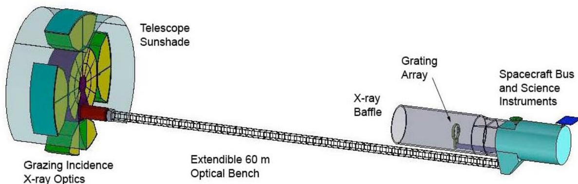
FIGURE 2.2 Artist's conception of one possible version of the Generation-X x-ray telescope. SOURCE: Courtesy of Roger Brissenden, Smithsonian Astrophysical Observatory.
