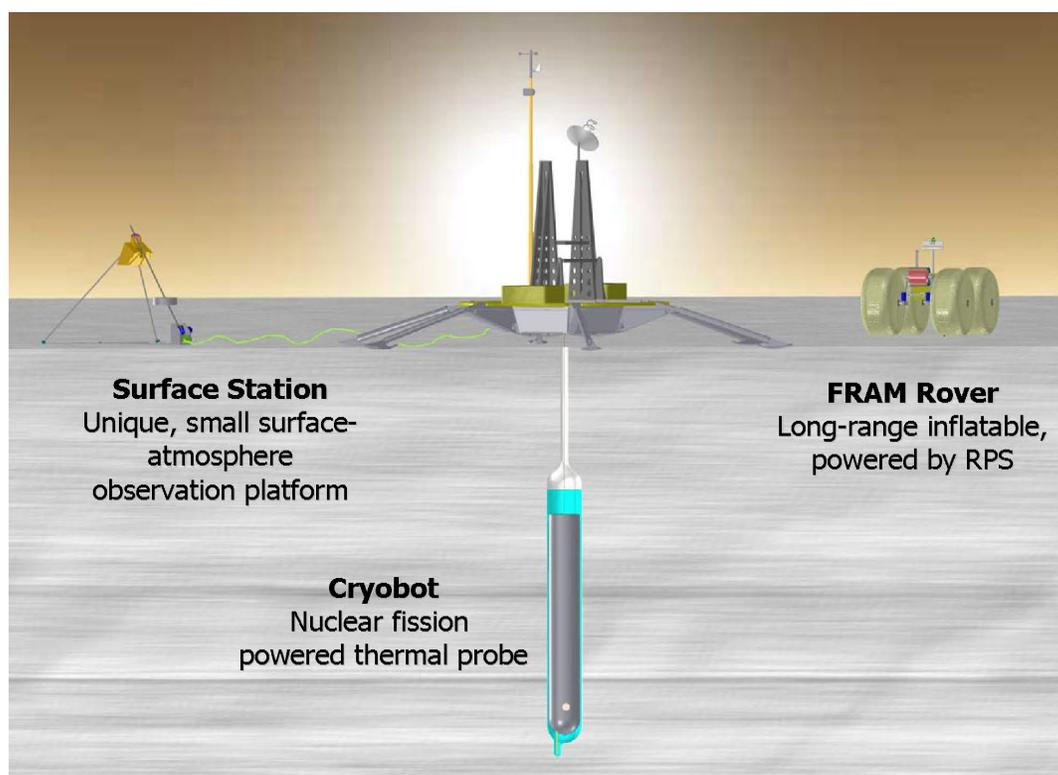
FIGURE 2.11 Illustration of the Palmer Quest spacecraft elements, including a cryobot powered by a nuclear reactor, and the surface station and rover. SOURCE: Courtesy of NASA, Jet Propulsion Laboratory, California Institute of Technology.
