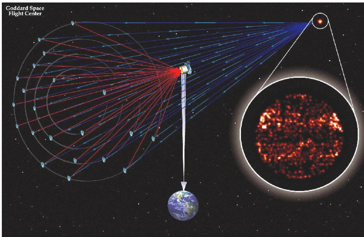
FIGURE 2.6 Illustration of the Stellar Imager, which uses a large array of formation-flying mirrors (left) to focus light on a common beam-combining hub (center) to produce ultrahigh-resolution images of stars and other celestial targets (right). SOURCE: Courtesy of K. Carpenter, NASA Goddard Space Flight Center.
