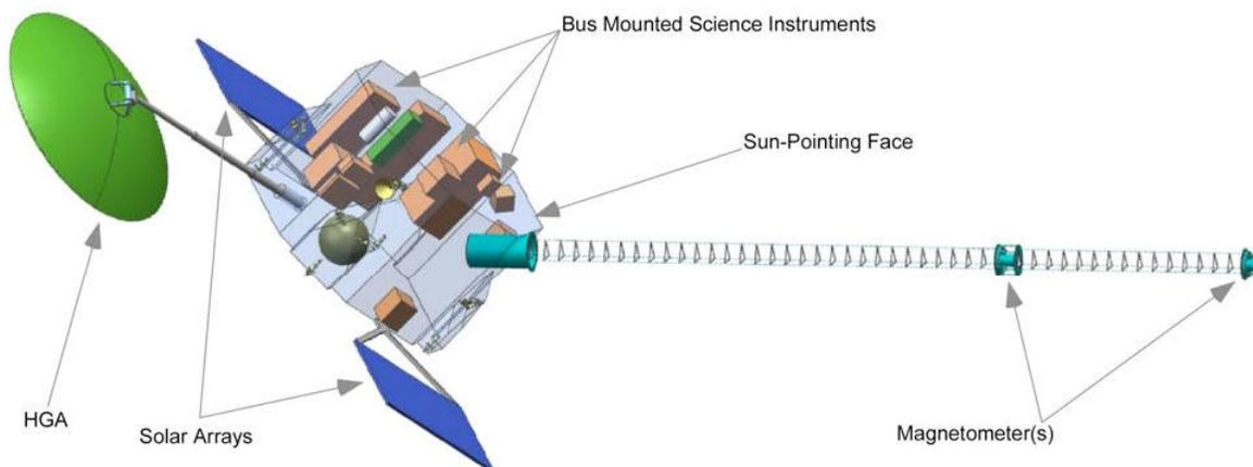
FIGURE 2.8 Illustration of the Solar Polar Imager spacecraft. SOURCE: Courtesy of NASA, Jet Propulsion Laboratory, California Institute of Technology.
