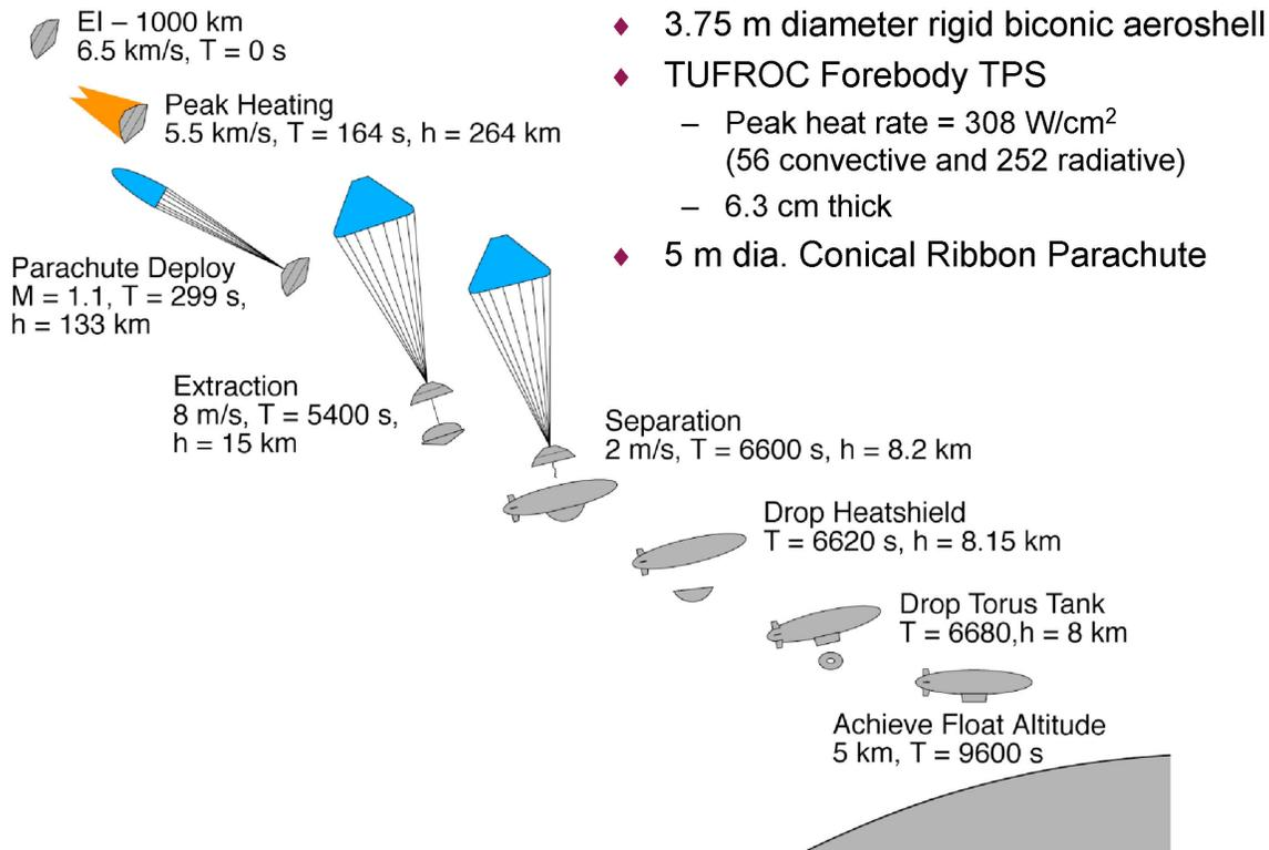
FIGURE 2.10 Illustration of the deployment sequence for the Titan Explorer airship. SOURCE: Courtesy of Joel S. Levine, NASA.
