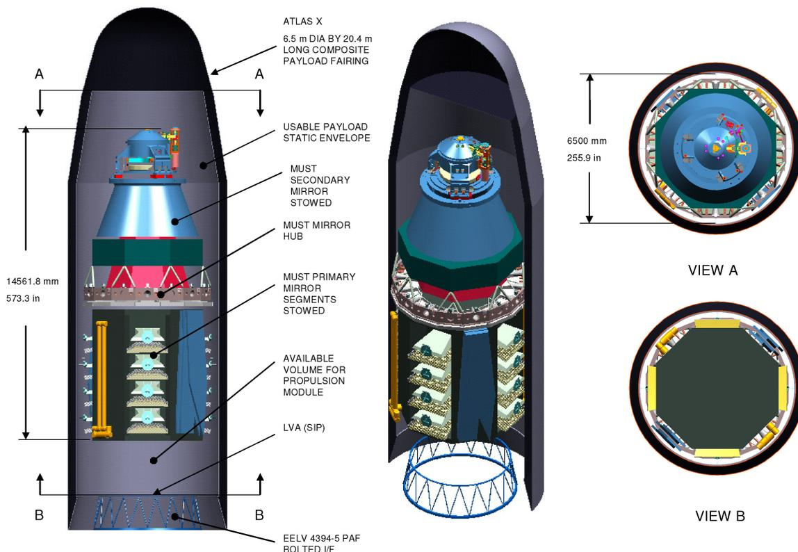
FIGURE 2.5 Artist illustration of the Modern Universe Space Telescope (MUST) inside its launch vehicle prior to assembly in space. SOURCE: Courtesy of NASA.
