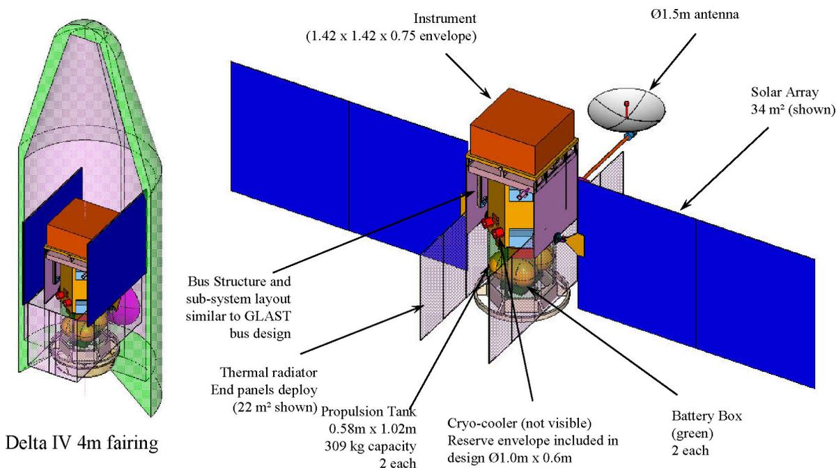
FIGURE 2.1 Artist's illustration of the Advanced Compton Telescope in both mission configuration and stowed within a Delta IV payload shroud. SOURCE: Courtesy of S. Boggs, NASA.
