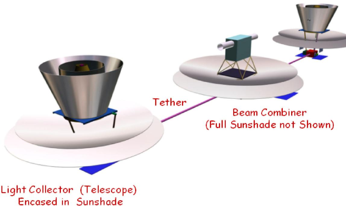
FIGURE 2.4 Artist's illustration of the Kilometer-Baseline Far-Infrared/Submillimeter Interferometer. SOURCE: Courtesy of the SPECS Consortium, prepared as part of a NASA Vision Missions study.
